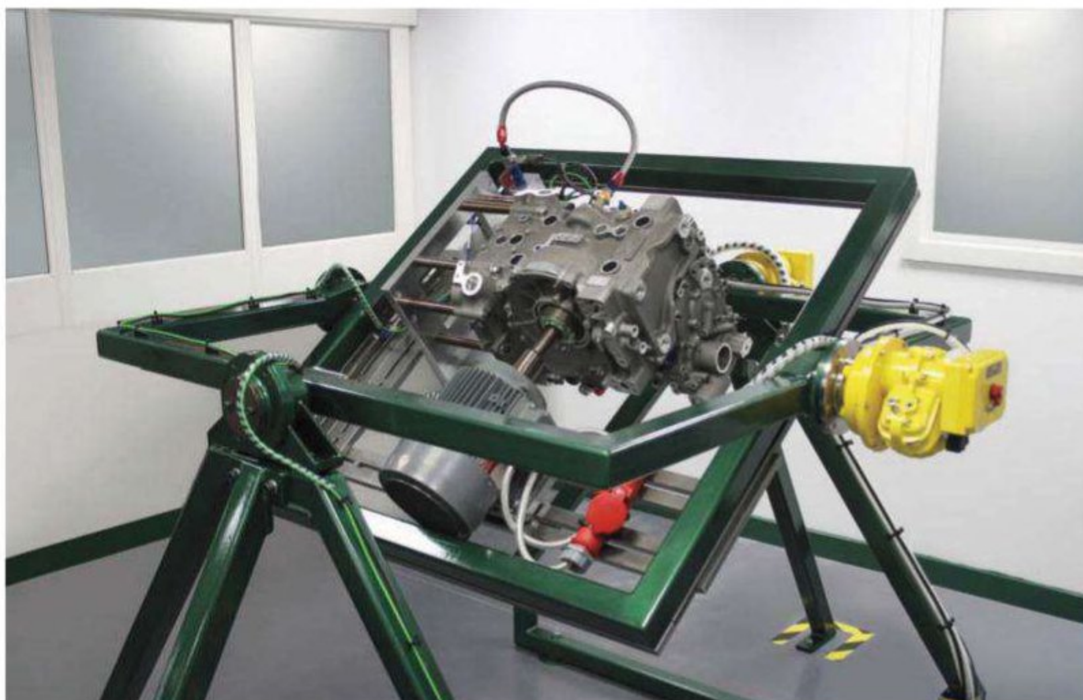
In house gimbal test rig allowed Xtrac to do physical simulations of the g forces the gearbox will undergo on track
