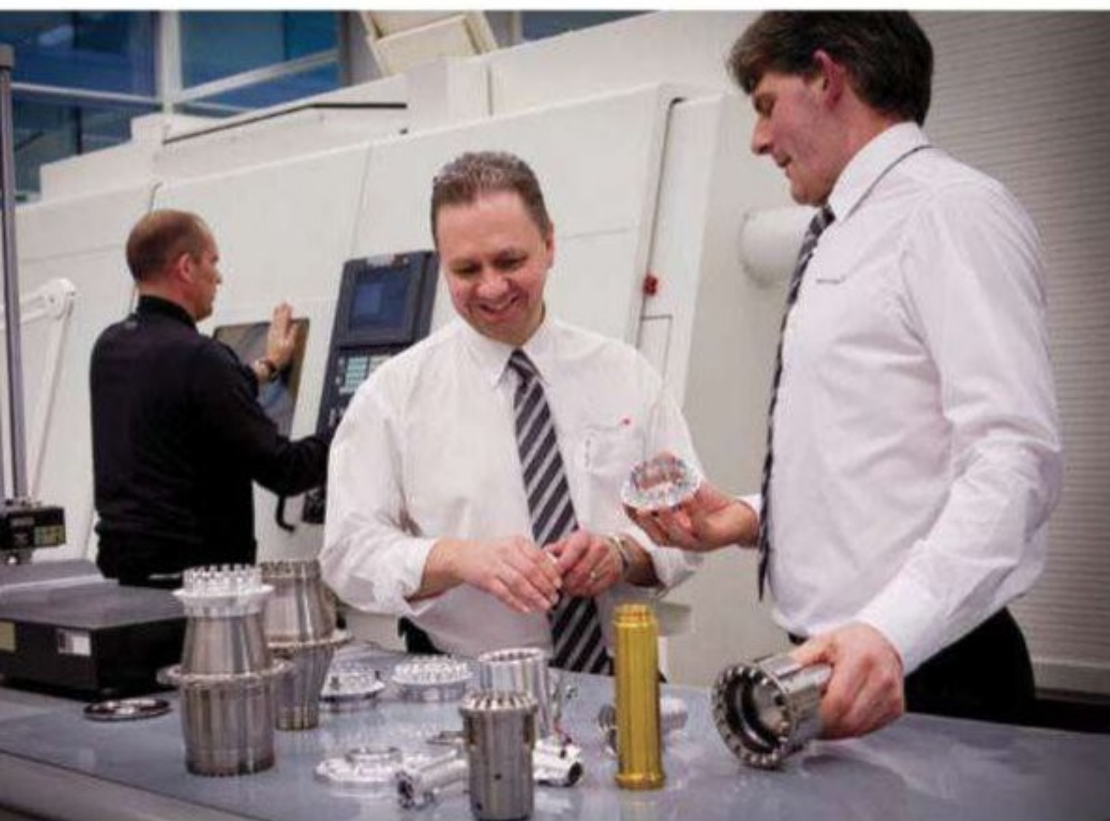
Wheel gun jaws are made in titanium to save on weight - not to make the job of the pit crew easier, but to save money on travel. With the wheel guns being shipped several thousand miles around the world over the course of a season, the saving on shipping outweighs the cost of manufacture
