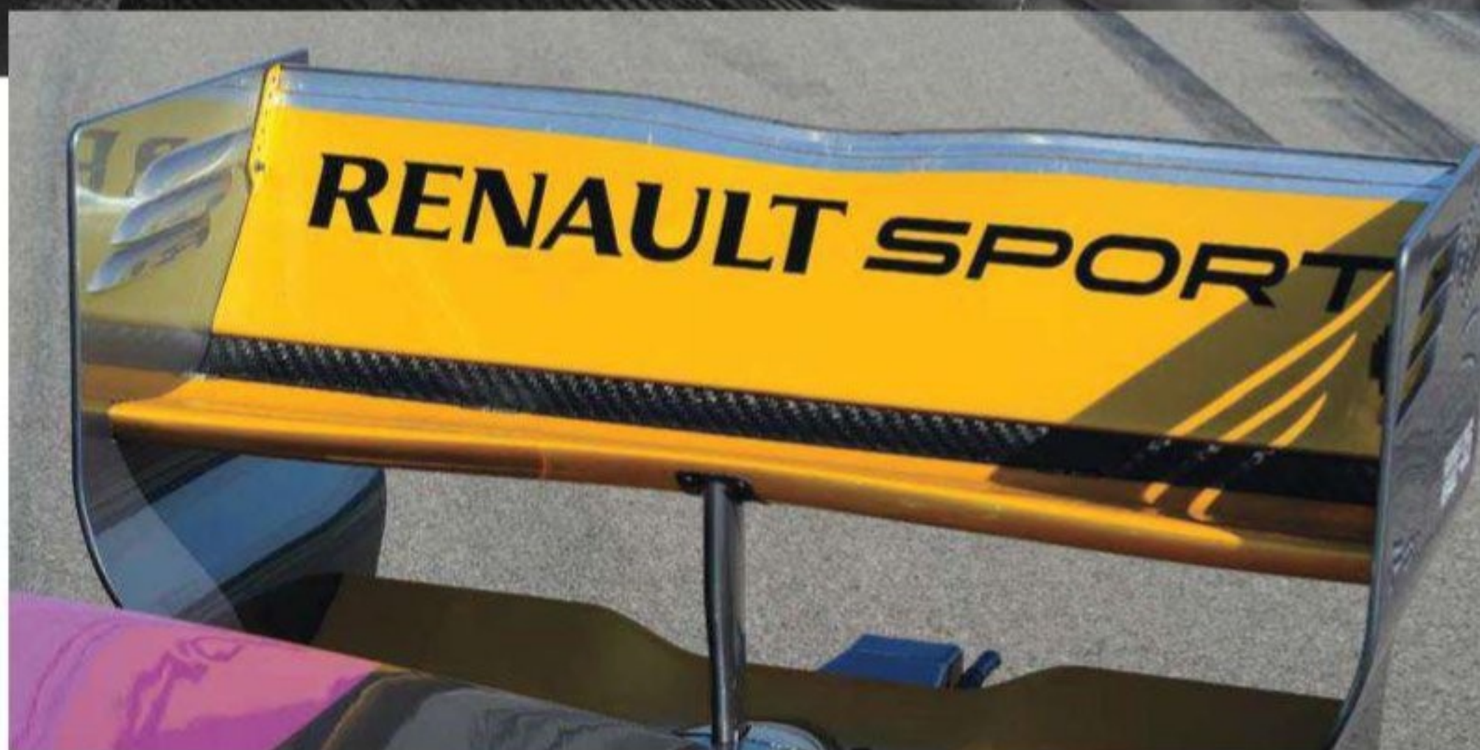
The inclusion of a Formula 1-style, driver-operated drag reduction system (DRS) makes the aero package on the Renault 3.5 unique amongst spec series
