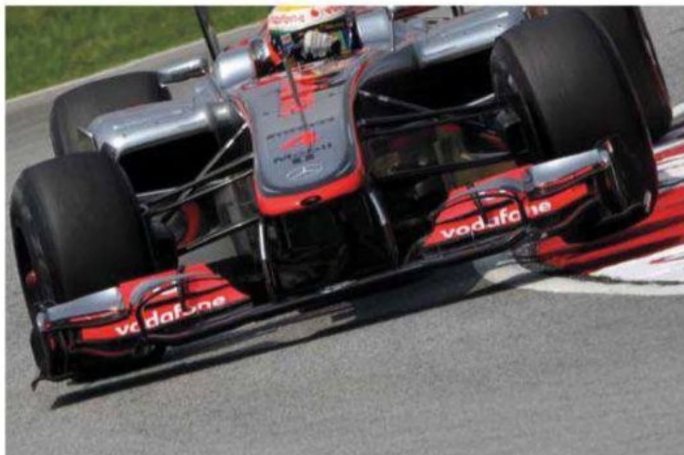
Below the unusual (for 2012) low nose, the McLaren has a radical new wing, constructed from billet aluminium, skinned with carbon, with ballast pockets
