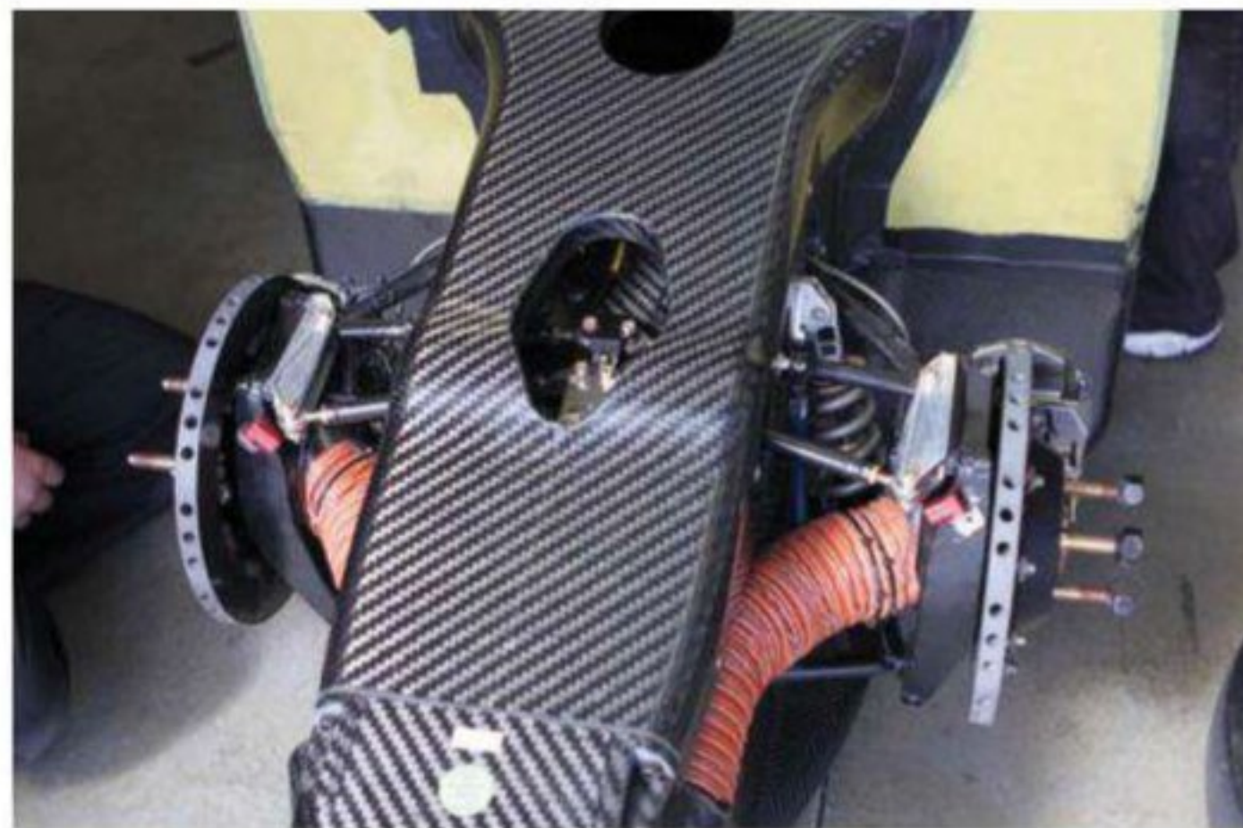
Front suspension has been kept remarkably simple and elegant, with no anti-roll bar, no camber and only 1mm of toe out on each wheel
