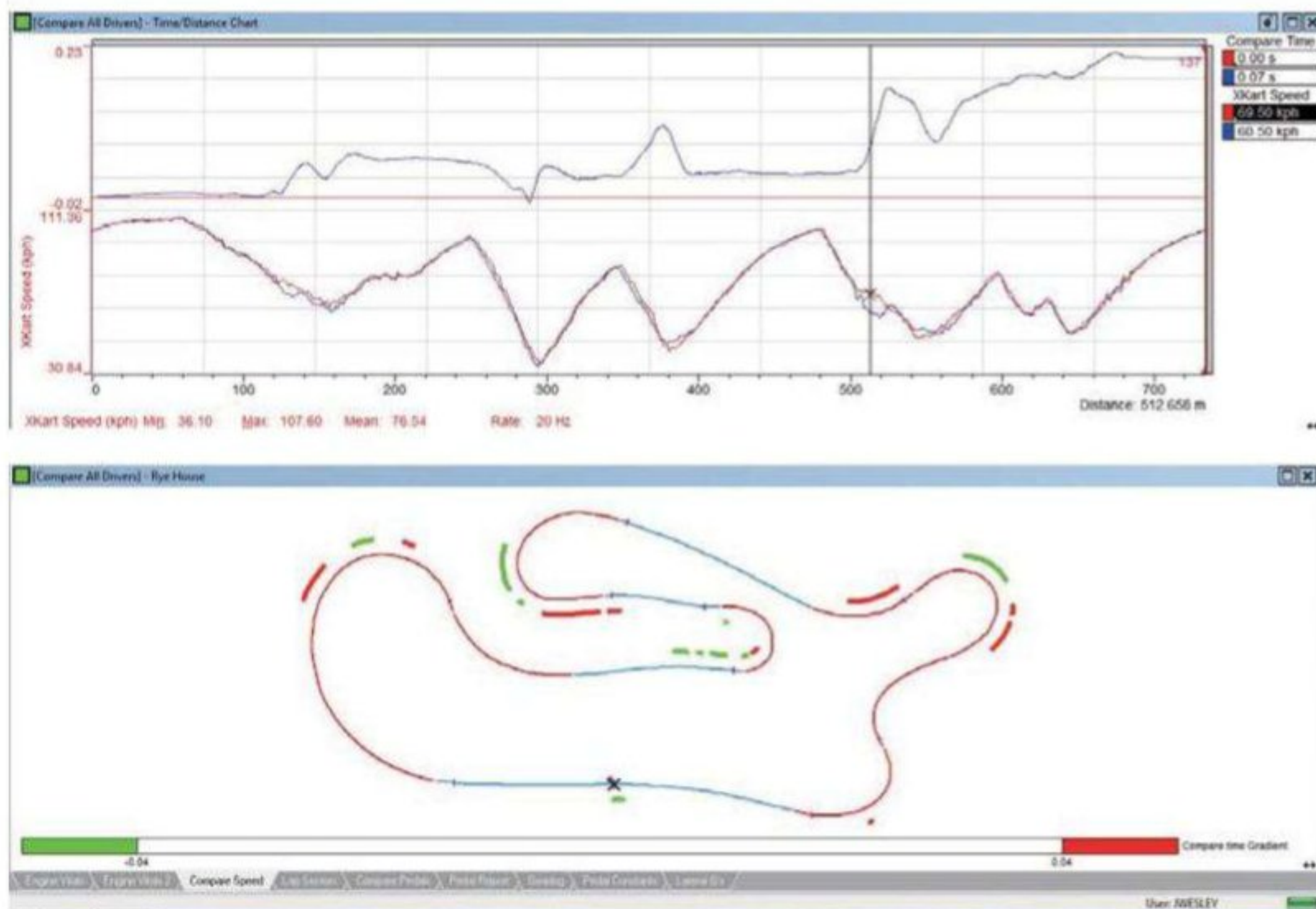
Figure 2: compare time gradient plotted on a track map to highlight main areas for improvement
