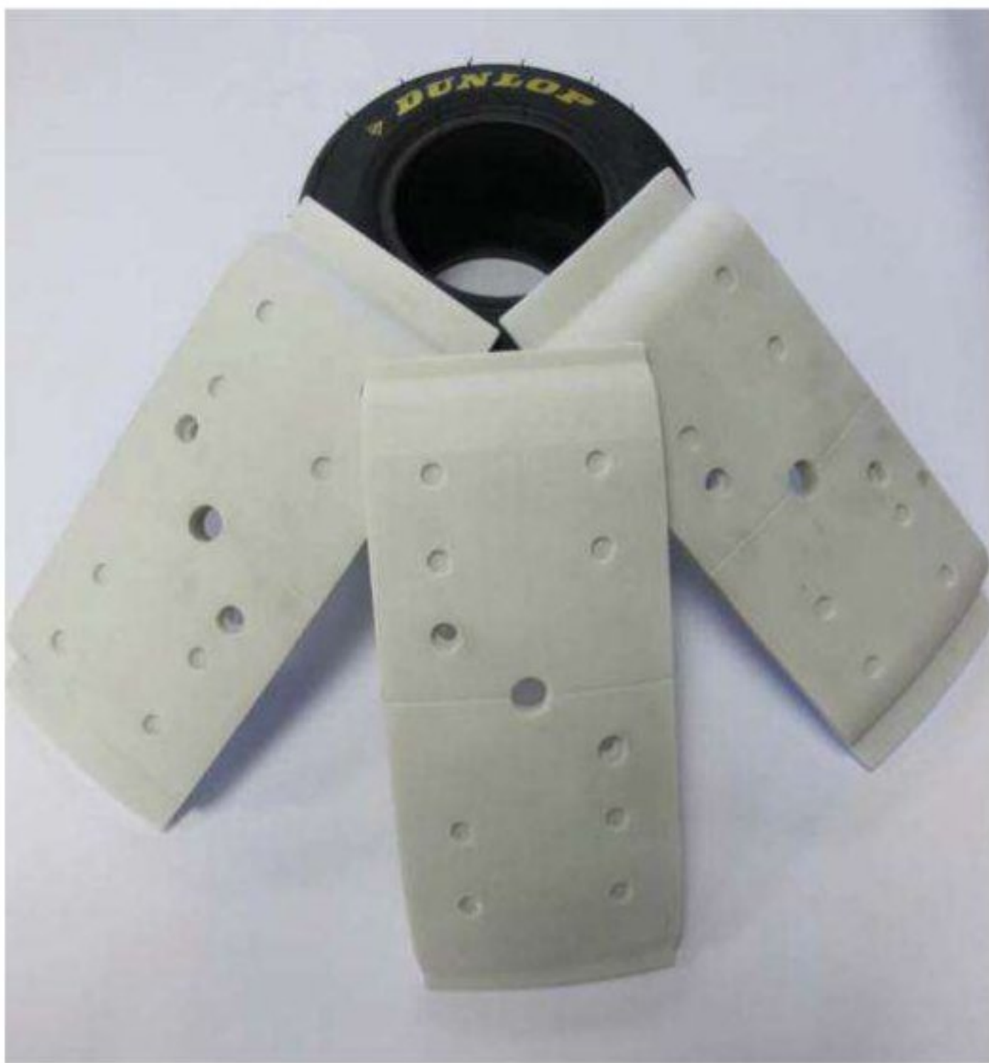
Rapid prototyping allows Dunlop to change the profile of the build machine segments in hours rather than days
