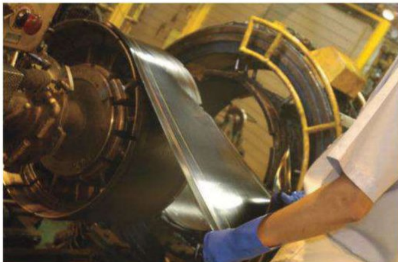
Laying up the carcass layer by layer by hand on the tyre building machine
