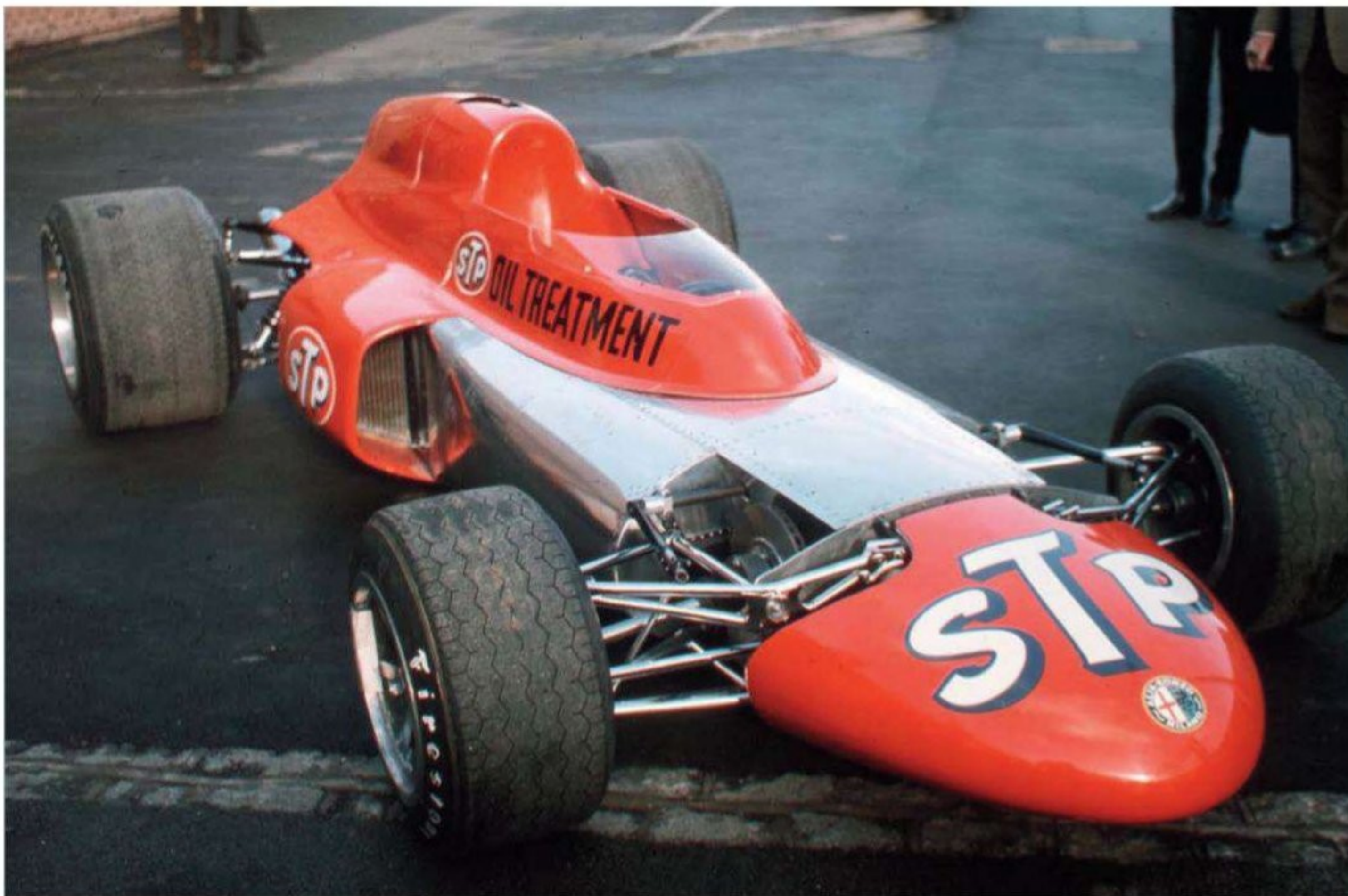
Using inboard brakes, you remove the action of brake torque on the uprights and control arms, with only the retardation forces going through the uprights
