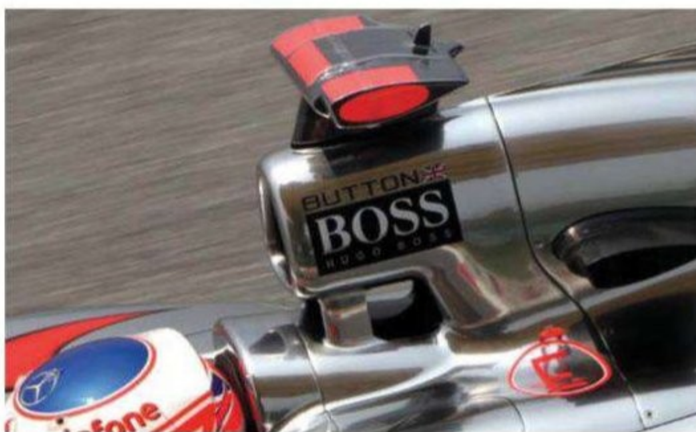
Roll hoop is also machined from billet, and passed the crash test with flying colours, so will be pared down even further for the 2013 car
