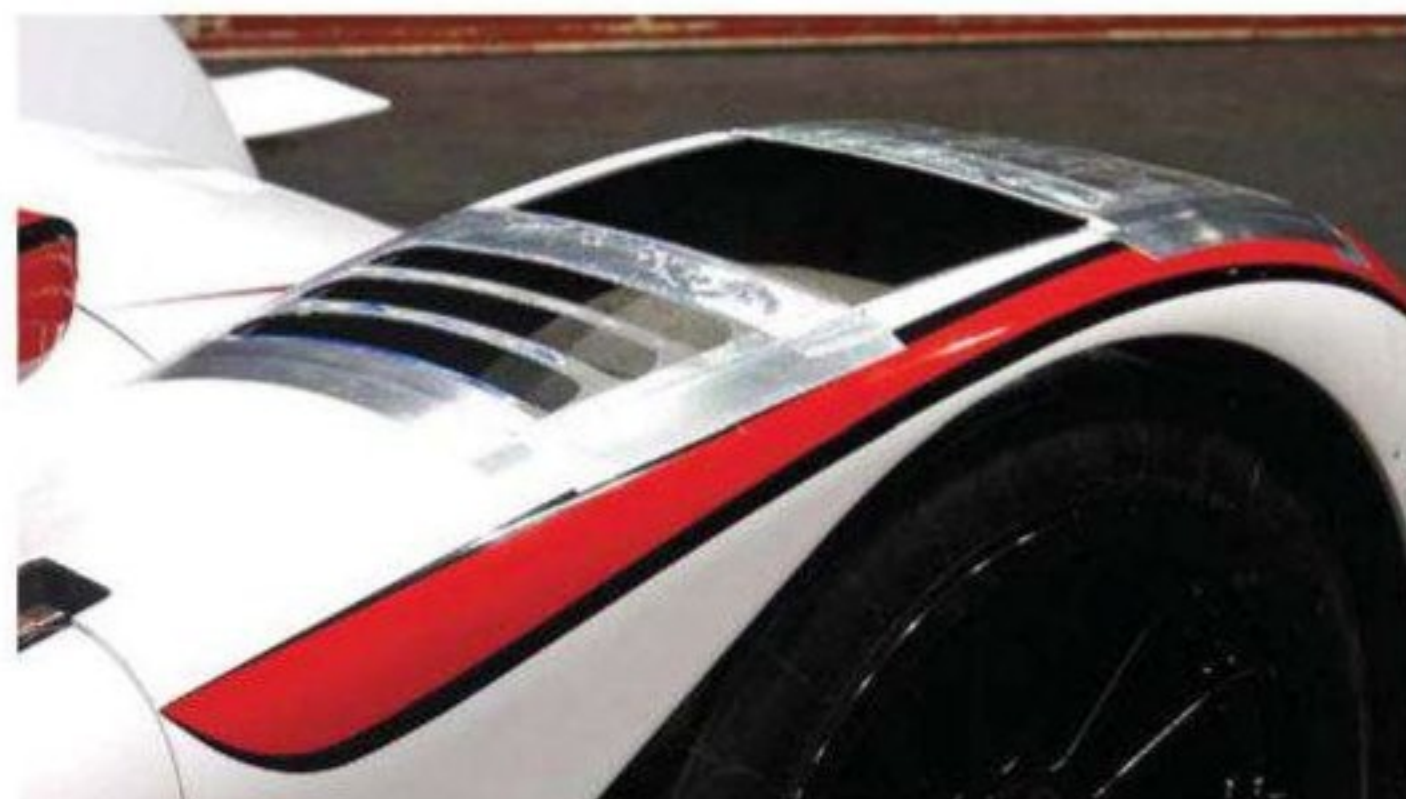
Figure 3: the wheelarch apertures also altered aerodynamic balance
