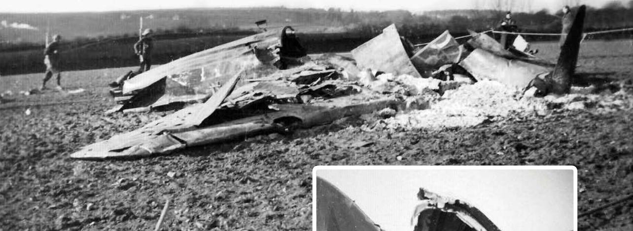
ABOVE & RIGHT The wreckage of DN510 at Meavy, on the south-west edge of Dartmoor in Devon, after its tailplane failed on February 4, 1943; the only instance of such an accident in which the pilot lived to tell the tale. Note the static balance lever still attached to the bracket on the bulkhead in the photograph at right. In some of the earlier tailplane failures the lever had sheared off from the bracket altogether. FAST VIA AUTHOR
