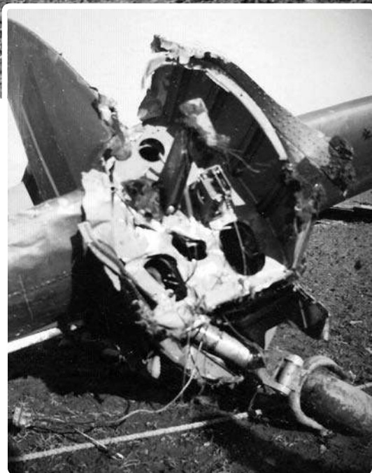
ABOVE & RIGHT The wreckage of DN510 at Meavy, on the south-west edge of Dartmoor in Devon, after its tailplane failed on February 4, 1943; the only instance of such an accident in which the pilot lived to tell the tale. Note the static balance lever still attached to the bracket on the bulkhead in the photograph at right. In some of the earlier tailplane failures the lever had sheared off from the bracket altogether. FAST VIA AUTHOR
