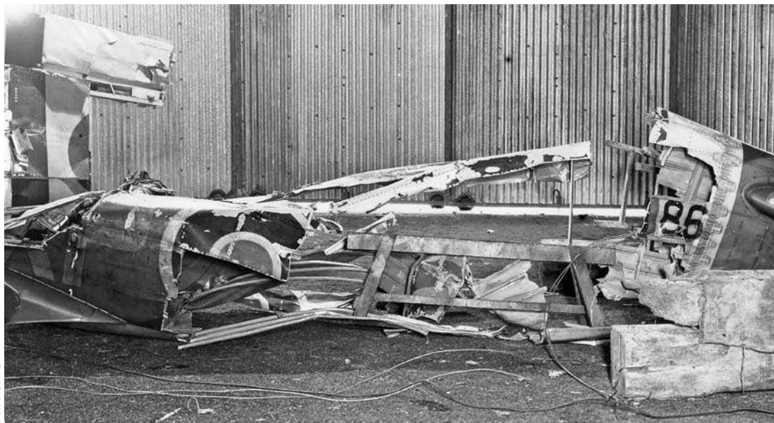
ABOVE With the distinctive fishplates added at the transport joint as per Mod 286 clearly visible immediately aft of the serial, the wreckage of EK186 awaits further inspection after having broken up in mid-air near Redhill on May 4, 1943. The cause of these failures continued to mystify the investigation teams at Hawker and the RAE.
