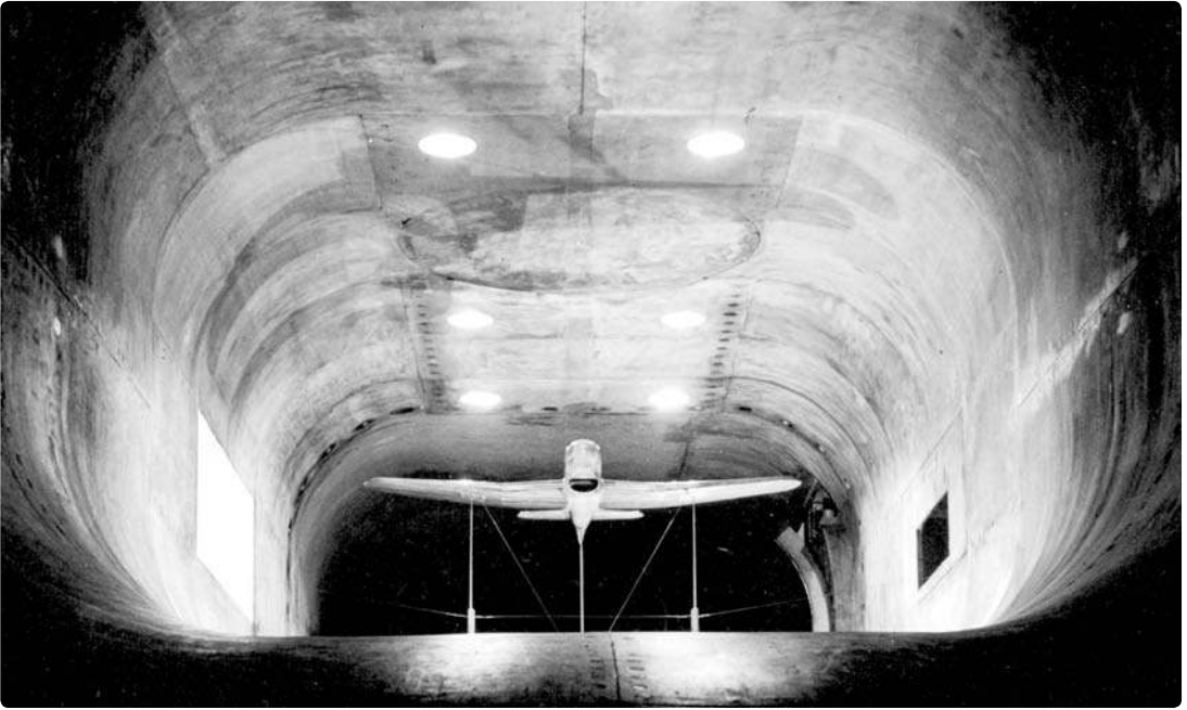
ABOVE A Typhoon model in the high-speed windtunnel at RAE Farnborough. The tunnel was opened in November 1942 and was designed to test scale-models of up to 6ft (1.8m)-span at windspeeds up to 600 m.p.h. (965km/h). BELOW A contemporary schematic showing the circuit-test details for the elevator's mass-balance system.
