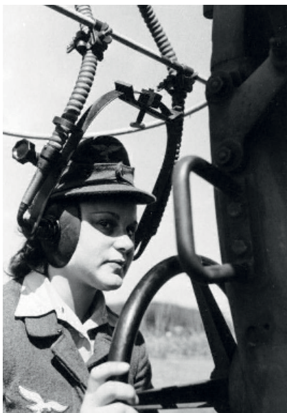
■ A Luftwaffenhelferin attached to the Flugmeldedienst, or aircraft reporting service, operates a sound locator tracking bombers.
