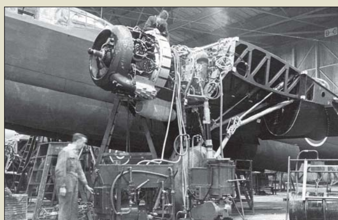
ABOVE: The Bristol Hercules 'power egg' being installed by Armstrong Whitworth engineers. FLIGHT (KEY ARCHIVE)
