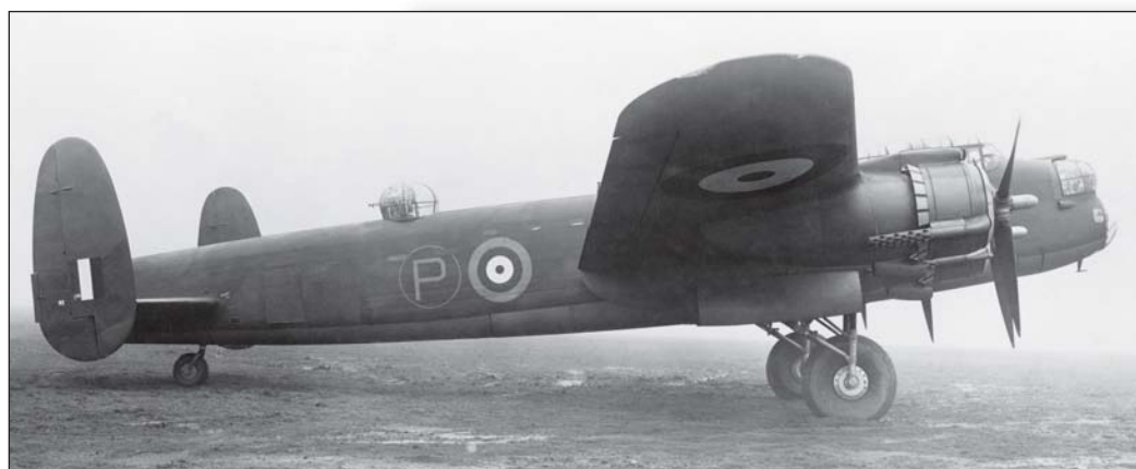
ABOVE: Originally two prototypes were ordered but DT810 was deemed sufficient to prove the theory that a Hercules-powered Lancaster would work. Hand-built at Chadderton, DT810 made its maiden flight from Ringway (Manchester International Airport) on November 26, 1941. AUTHOR'S COLLECTION
