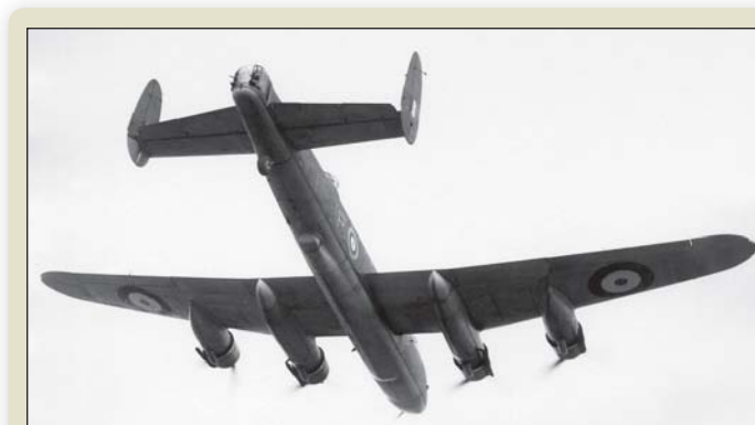
ABOVE: Unusual view of the underbelly of prototype DT810 which shows how well the rear of the modified bomb bay doors have been incorporated into the lower rear fuselage. AUTHOR'S COLLECTION
