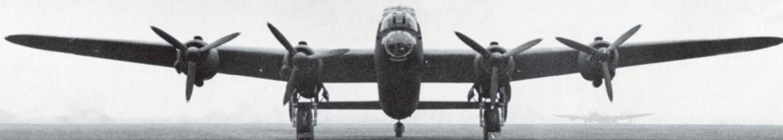
BELOW: The blunt end of a Lancaster Mk II pictured on December 6, 1943. Despite the lack of aerodynamics compared to the more streamlined Merlin, the Hercules engines provided enough grunt to propel the Mk II along at the same speed as its water-cooled counterpart. FLIGHT VIA AUTHOR
