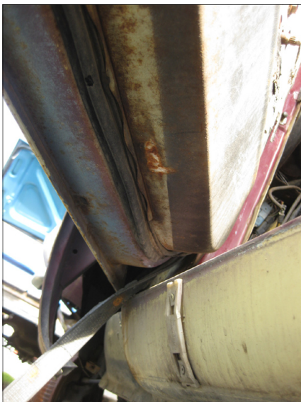
Inner door surface mask left a gap between the lower edge of the mask and the lower door weather-strip channel.
