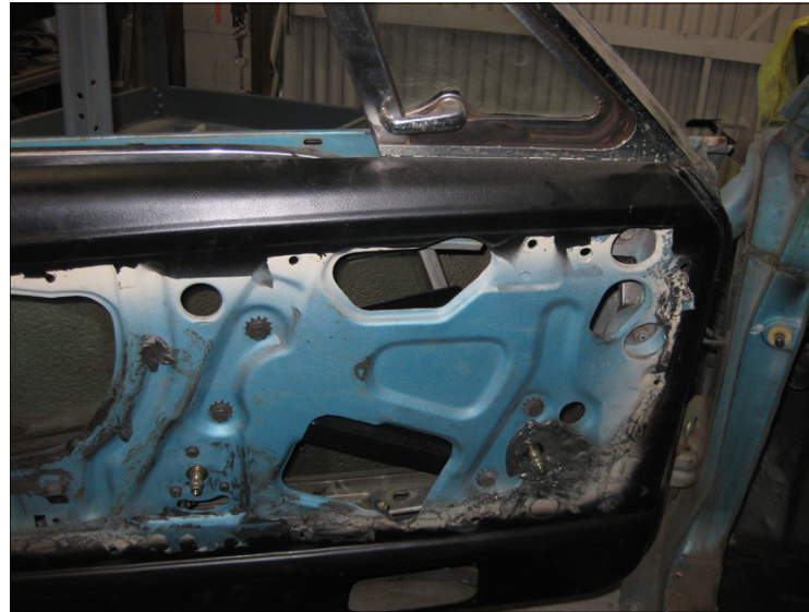
Once the interior of the door was painted a mask was taped over the inner surface of the door leaving the pattern above.
