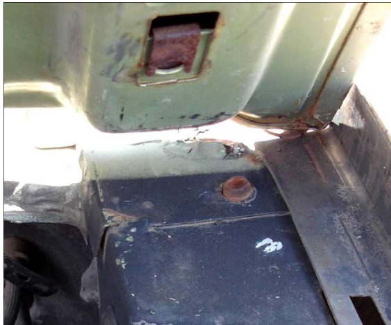
Correct location of black paint to cowl body color
