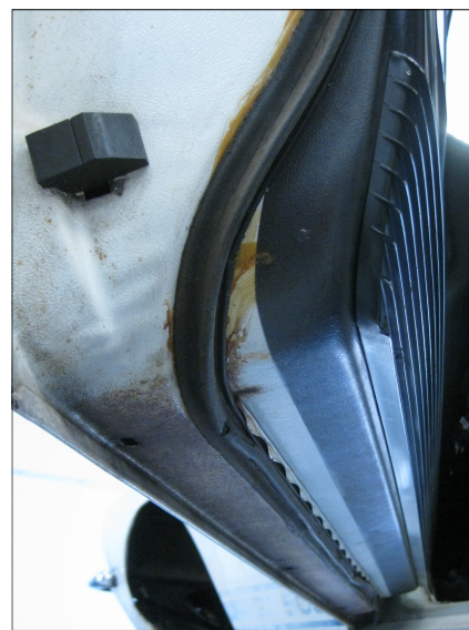
Inner door surface mask left a gap between the lower edge of the mask and the lower door weather-strip channel.
