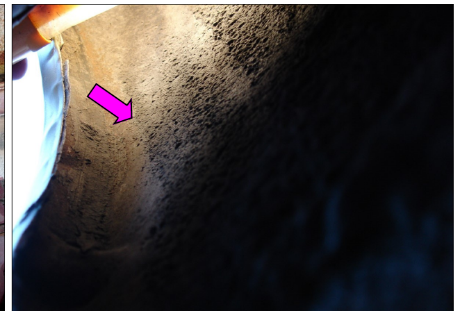
Sound deadener not applied all the way to fender lip.
