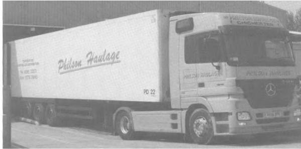
An articulated combination featuring a box trailer, which in this case is refrigerated
