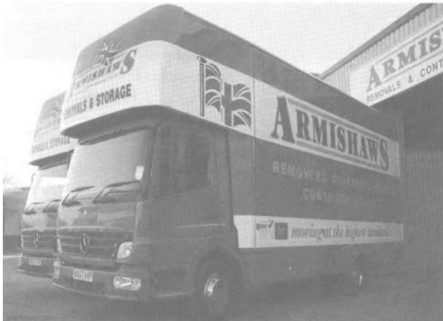
A rigid vehicle fitted with a high cubic capacity body for high volume/low weight cargo, which in this case are household goods
