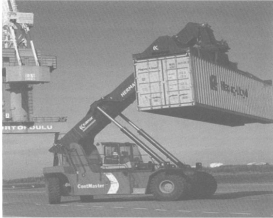
Reach stacker handling an ISO container
