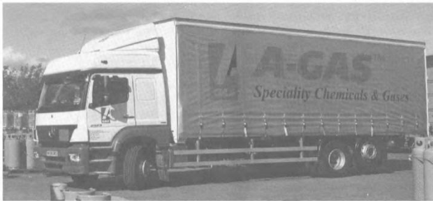
A six-wheeled rigid vehicle fitted with a lifting rear axle
