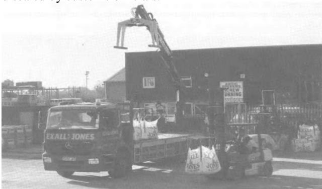
A platform or flat bed rigid vehicle with drop sides, which in this case is fitted with its own crane to assist loading and unloading
