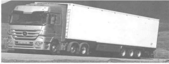
An articulated vehicle comprising a tractor and semi-trailer
