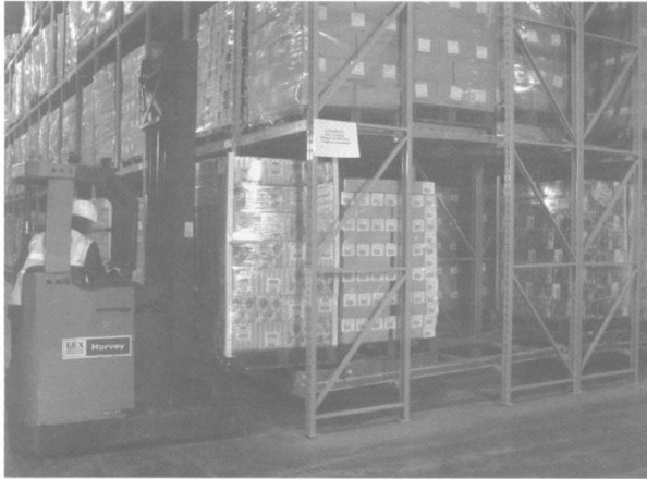
Push-back racking, being served by reach truck
