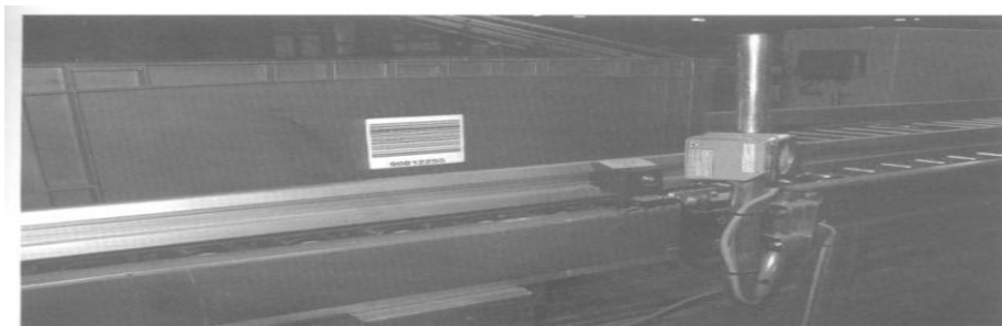
Automatic bar code scanning of plastic tote box
