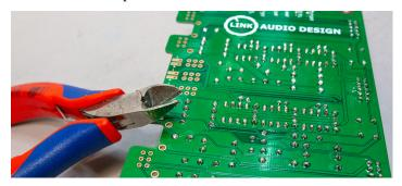
The next step is focusing on the pots and switches of the upper subboard, we can solder all pots and switches. Make sure to press them flush and firm to the poard and fix them with one solder point.
