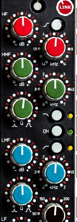
This Button switches from BELL-MODE into SHELF-MODE of the HF-Band
