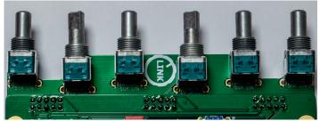
After having one pin of each pot soldered we add the bracket ike shown in the picture above. The direction of the bracket is shown in the picture below. After having all pots screwed to the bracket, we can solder all pins, then we need to cut the pins.
