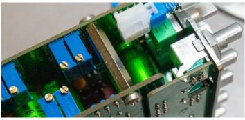
Now it's time to add the Frontpanel to complete the Equalizer. Use the spacers and the M3 Nuts to finish it. The Caps for the Knobs are sorted as following:
