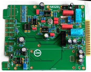
On the LED Meter Board we also add the electrolytics and Wima Capacitors and Board connections, and cut leads after soldering as short as possible. We will do this process later with Potentiometers also, since we need to make sure that this Preamp doesn't touch any neighbour modules of any kind.
