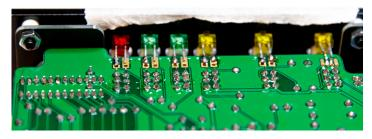
If you choose a yellow LED for Colour Module indication solder the long leg to R/Y and the short leg to the unlabeled Pin. If you want to solder RGB check the picture below.
