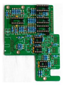
After that Step solder all Wima Capacitors, Electrolytics and Board Connectors as on the pictures.
