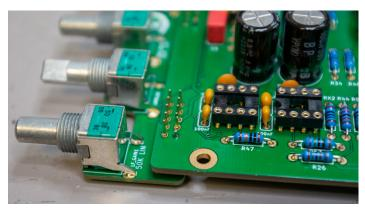
After that we can solder all the other pins and cut the pins also as short as possible. Then you can split our built adapter screws in two parts again.
