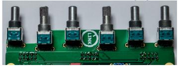
After having one pin of each pot soldered we add the bracket ike shown in the picture above. The direction of the bracket is shown in the picture below. After having all pots screwed to the bracket, we can solder all pins, then we need to cut the pins.
