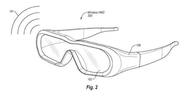
As a wearable device, a smartglass provides a computer screen and a background information system to the wearer. The display can be projected on the glasses lens, or a separate component is brought to the eye. The key feature of a smartglass is its ability to enable users to observe their surroundings without distractions. It also supports voice and gesture recognition. These features are also very useful in remote locations. Its cameras can help you to locate people.
