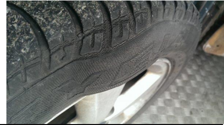
An example of an old tyre with good tread but with signs of cracking and deforming.
