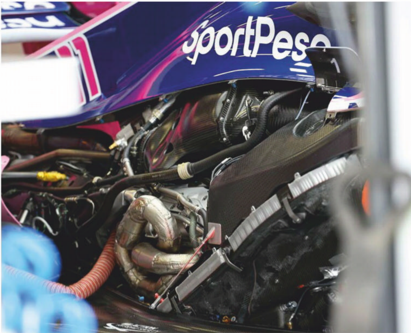
Mercedes power unit in the Racing Point. The team's tech director says that the current F1 PUs are simply 'too incredible'
