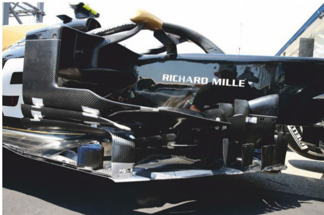
The bargeboard height in F1 was reduced for 2019, but they are still very complicated. Note the reshaped sidepod inlet
