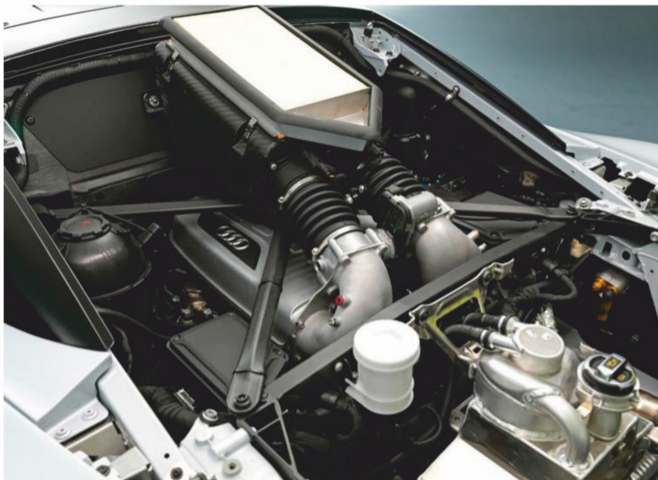
The 640bhp 5.2-litre V10 power unit is lifted from the road car and is not restricted, as it is in the company's GT3 racecar
