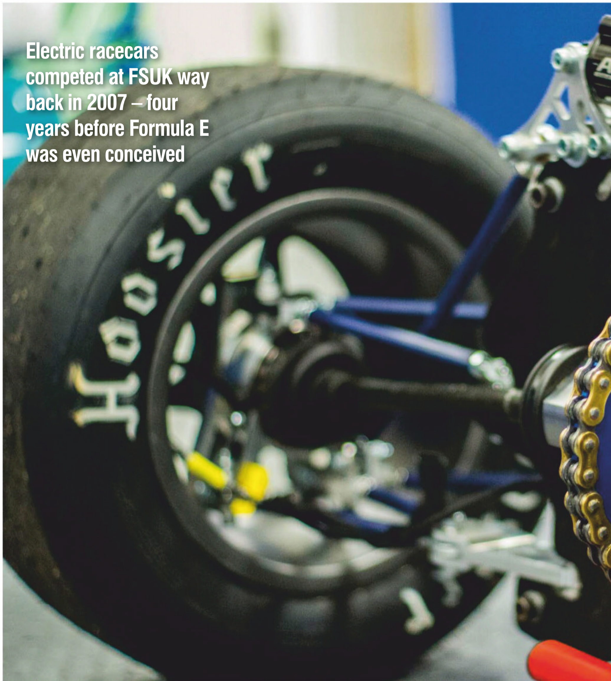
The Team Bath Racing car makes use of a chain drive solid spool axle, which is a common approach on Formula Student designs that are running with a single electric motor
