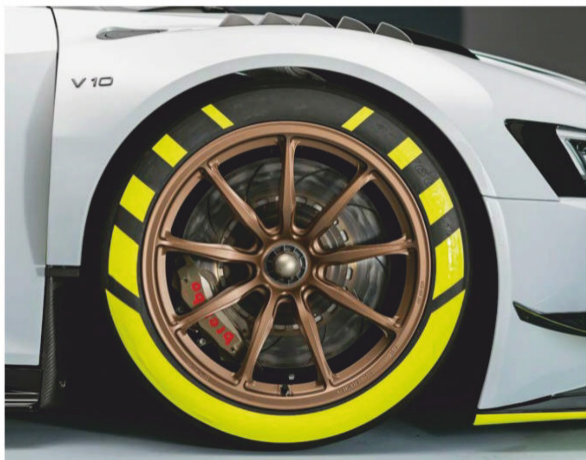
The car sits around 30mm higher than the GT3 R8. The calipers and steel brake discs are supplied by Brembo
