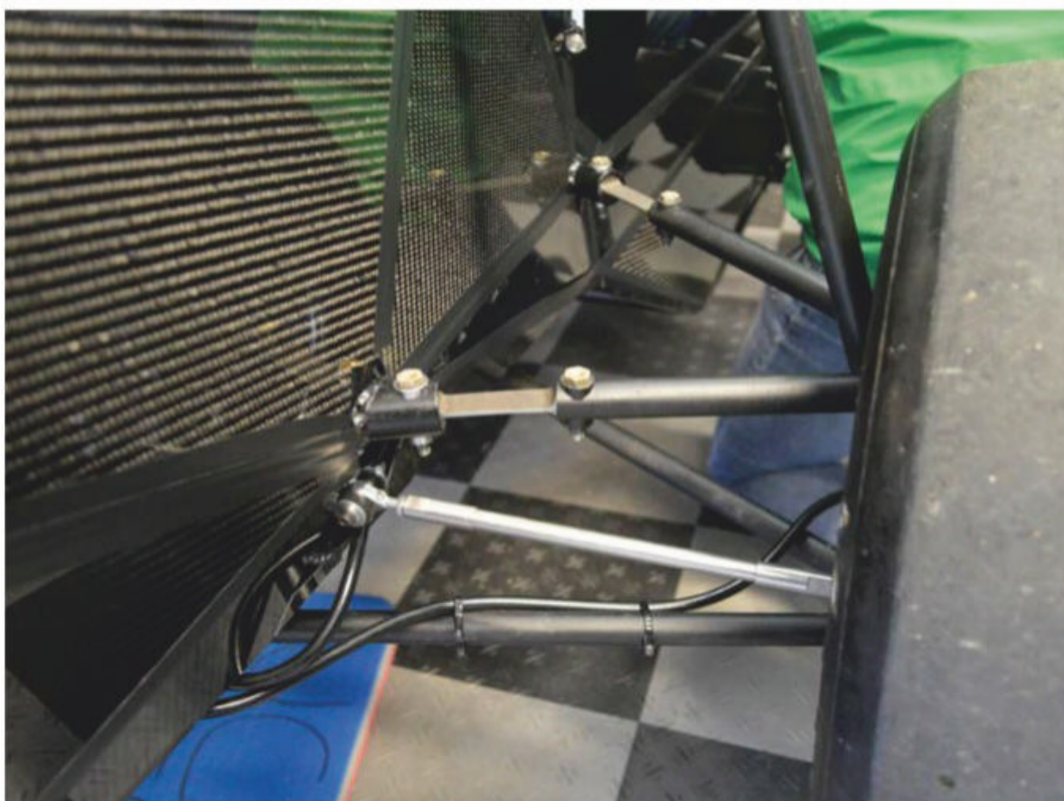
Flexures, seen here on the UCL control arms, are an alternative to the traditional spherical bearing approach
