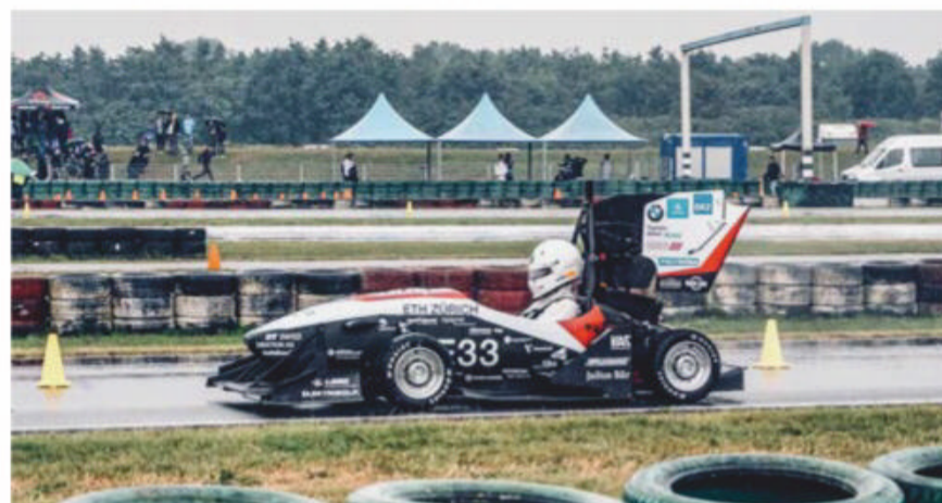
The remarkably light AMZ car features four 37kW wheel-mounted electric motors
