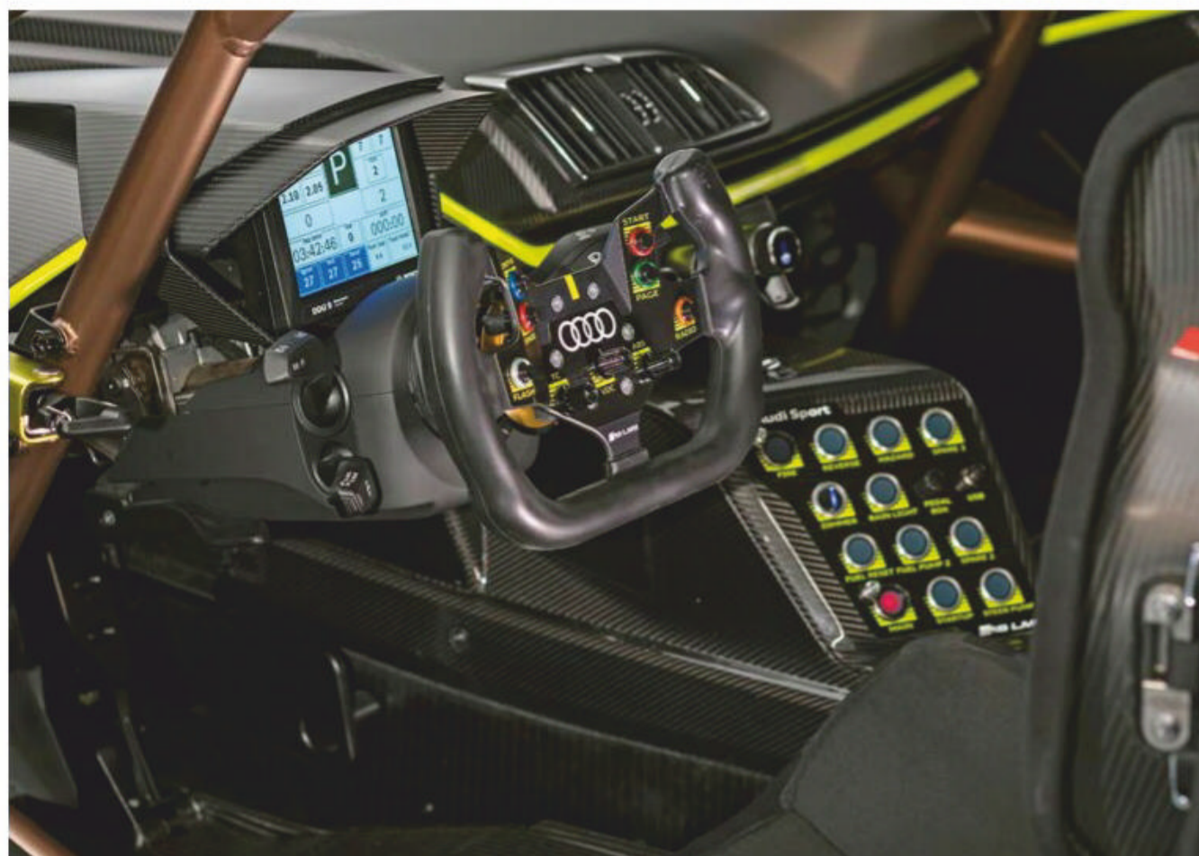
The steering wheel is more complex than the one in the GT4 and is adjustable for traction control, ABS and ESC stability
