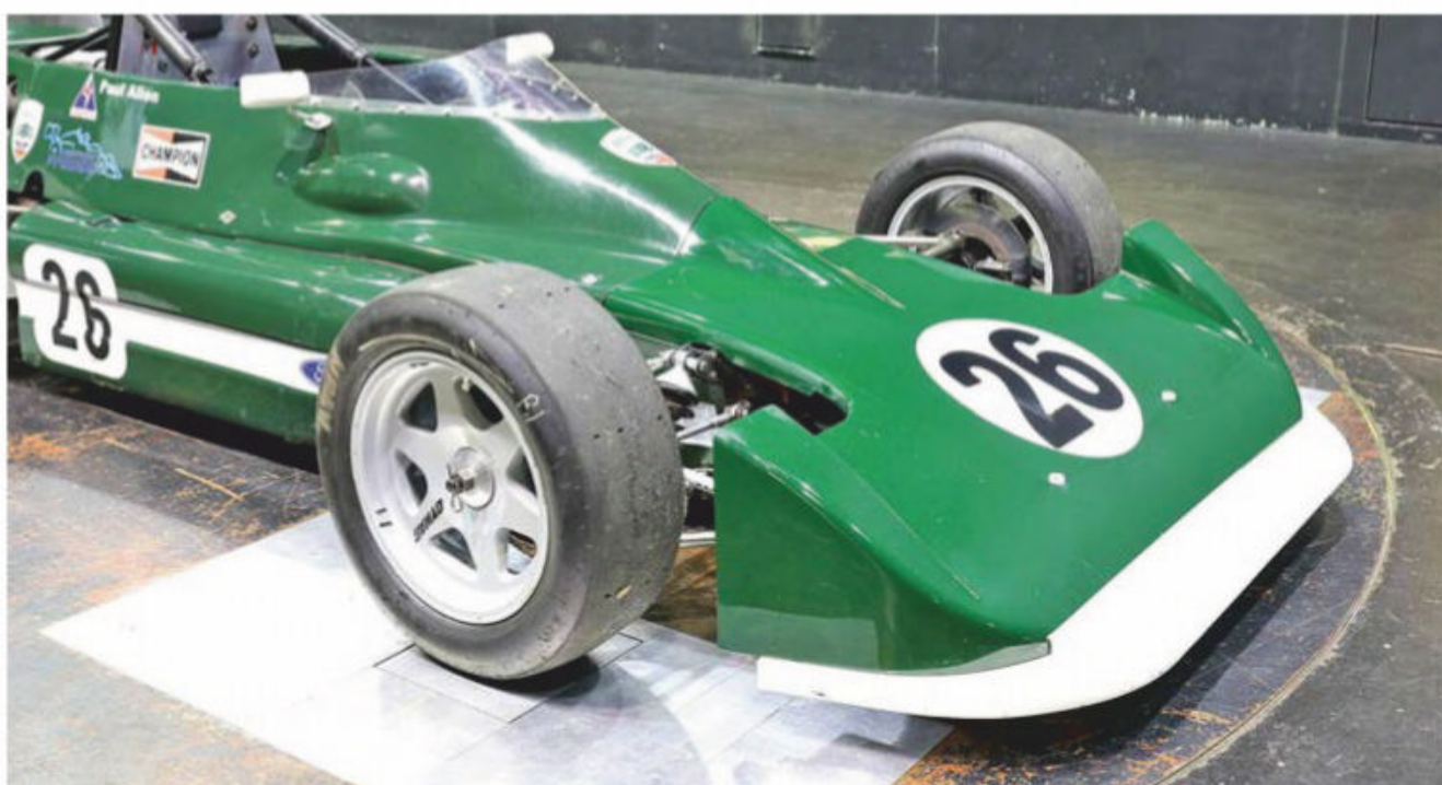
Wide, shallow nose with adjustable splitter. Narrow noses with single-plane wings were used on some other FF2000 racers
