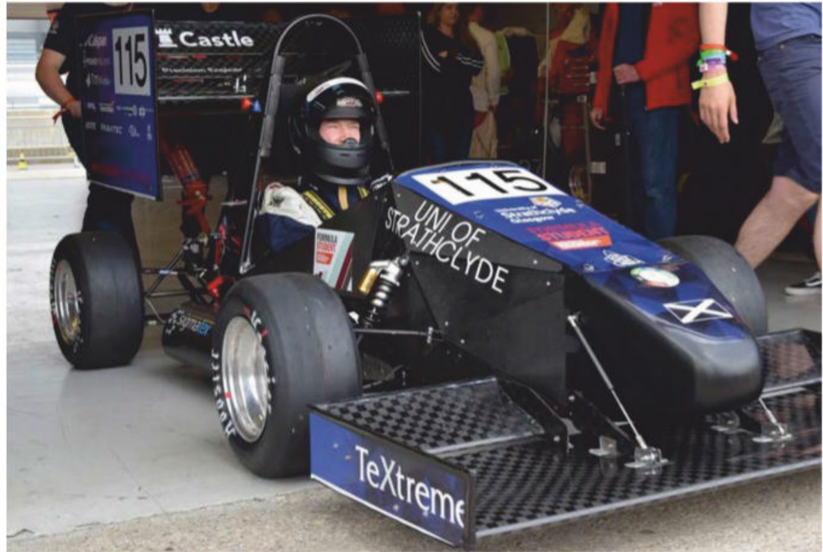
The ingenious use of gas struts on the Strathclyde FSUK entry allowed the front wing to run in ground effect
