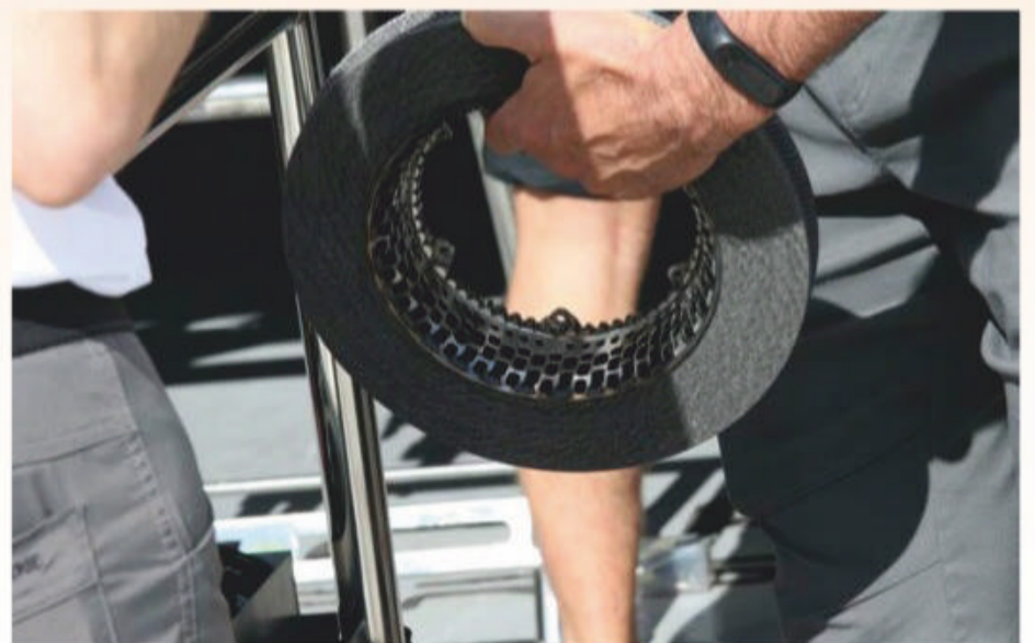
A rare shot of a Brembo F1 disc, as used by Haas, showing internal cooling channels
