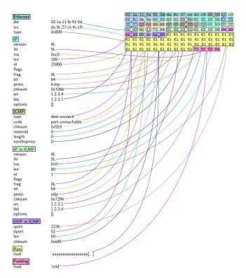
Figure 5. f\_usbnet's Leak (the 'Padding' field)
