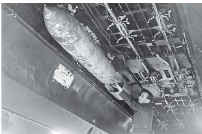
A feature of the Manchester that continued into later Avro 'heavies' was the huge, uninterrupted bomb bay that gave the design great strength. The 2,000lb AP bomb sits in a No 83 Squadron aeroplane. KEY COLLECTION
