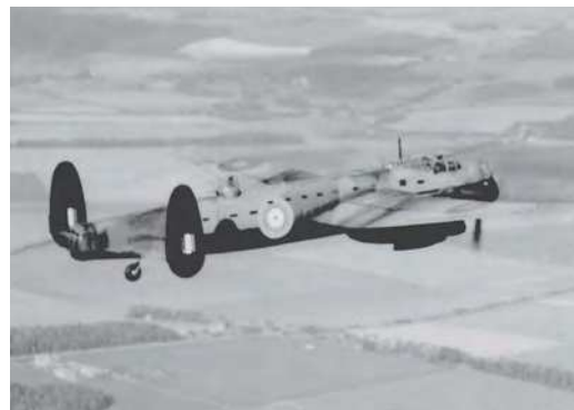
TOP: Second prototype L7247 was fitted with nose, tail and ventral turrets, the latter of which is in its extended position. It was retracted for take-off and landing. KEY COLLECTION
