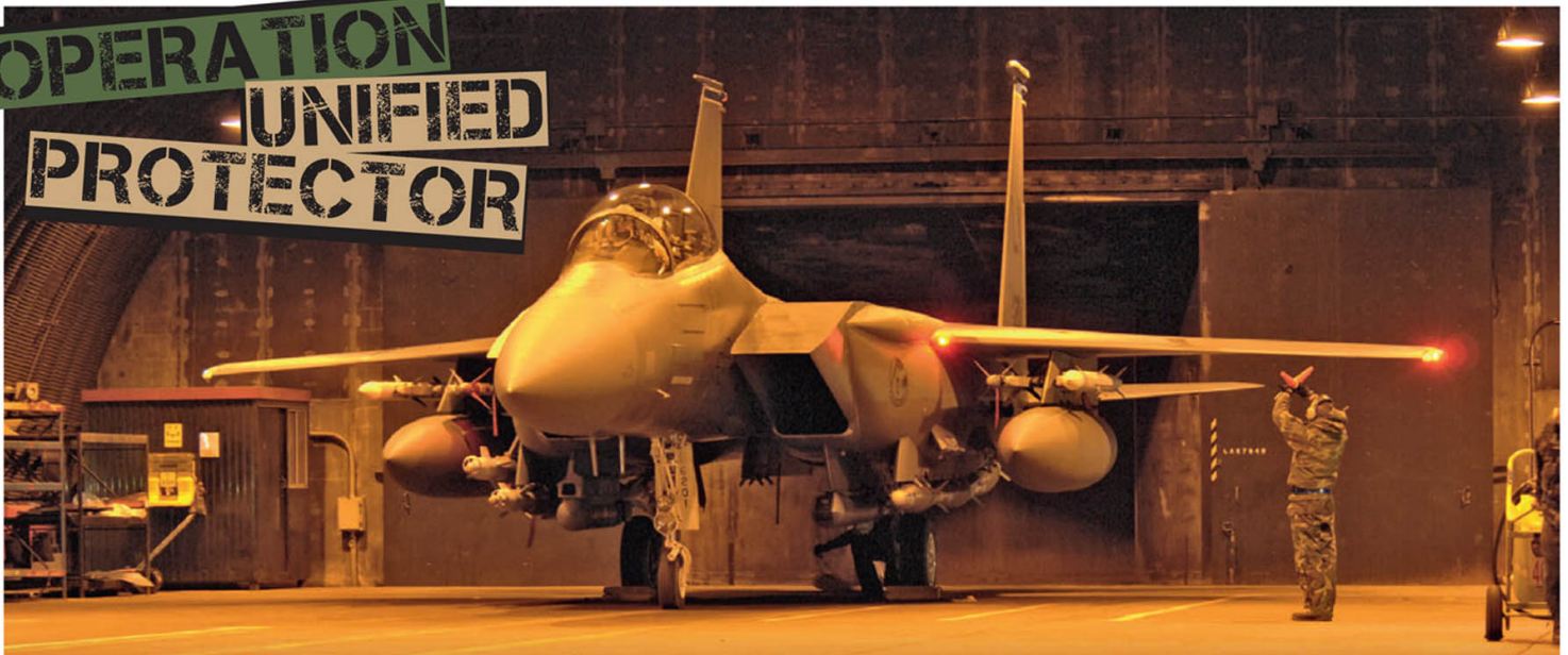
Above: A 48th Fighter Wing F-15E Strike Eagle, loaded with precision-guided munitions and AMRAAM missiles, prepares to taxi from a hardened aircraft shelter at Aviano AB, Italy. The 48th FW lost an F-15E in Libya on March 21 reportedly because of mechanical failure.
