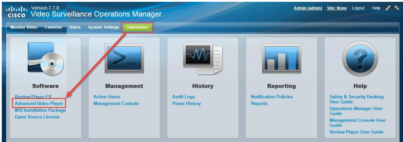
Figure 2 Downloading the Cisco SASD Advanced Video Player Installer from the Operations Manager
