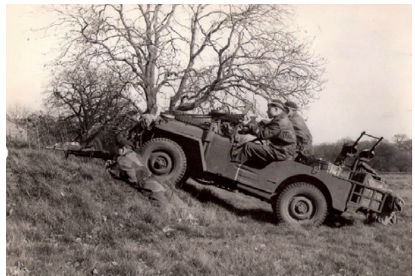
A jeep in an ambush position with the rear gunner in the ditch manning a Bren, during a 2SAS training exercise in England, August 1944. The half-moon armour plating is visible in front of the Vickers and the spare tyre is strapped to the bonnet. On active operations, the SAS tied the front wheel to the radiator and attached spare Vickers magazines to the bonnet (one of which can be seen here). The pannier at the back of the jeep is where the men kept their personal kit. (Gavin Mortimer)
