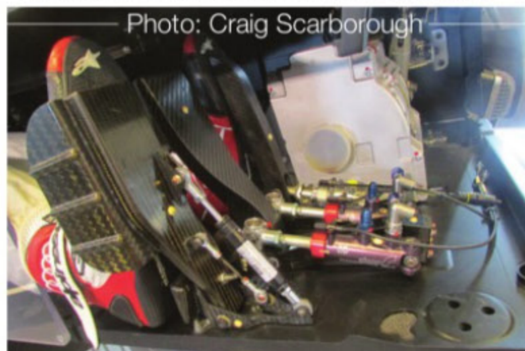
ABOVE & BELOW Audi has worked hard on the cockpit ergonomics, moving important controls such as the clutch to the steering wheel (above), where the older car featured a three-pedal setup (below)
