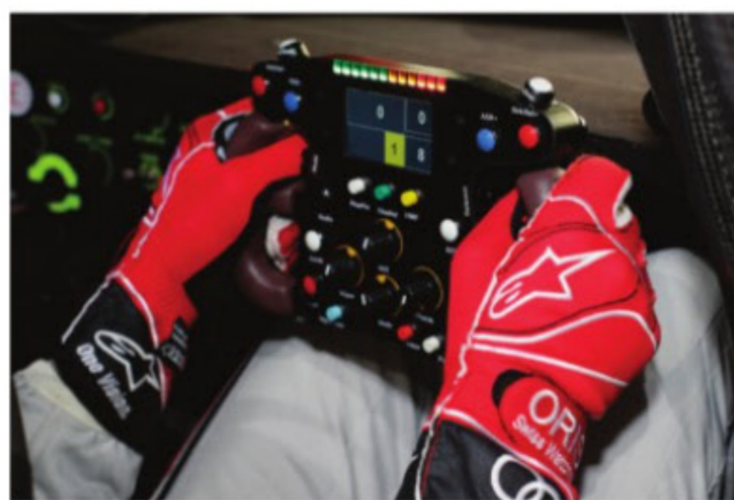
ABOVE & BELOW Audi has worked hard on the cockpit ergonomics, moving important controls such as the clutch to the steering wheel (above), where the older car featured a three-pedal setup (below)
