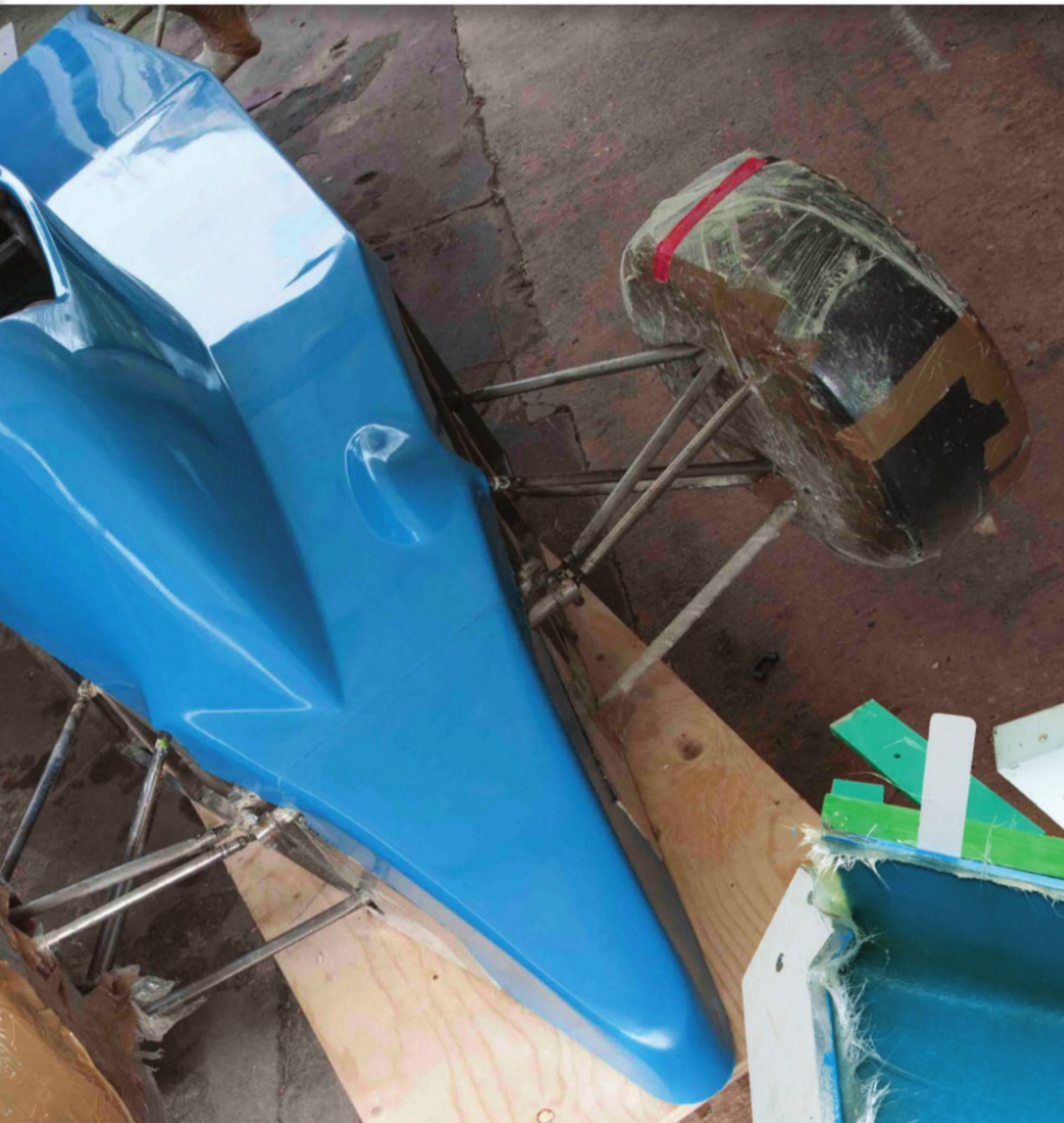
BELOW The main mould after the careful application of the gel-coat. Space is at a bit of a premium!
