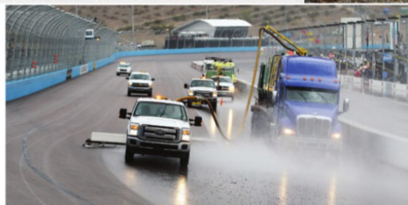
BELOW Dry line: the Mk1 version of the Air Titan was a great advance over the previous kerosene jet driers, graphically illustrated here at Phoenix earlier this season. Note the lorry carrying the compressed air generators at right
