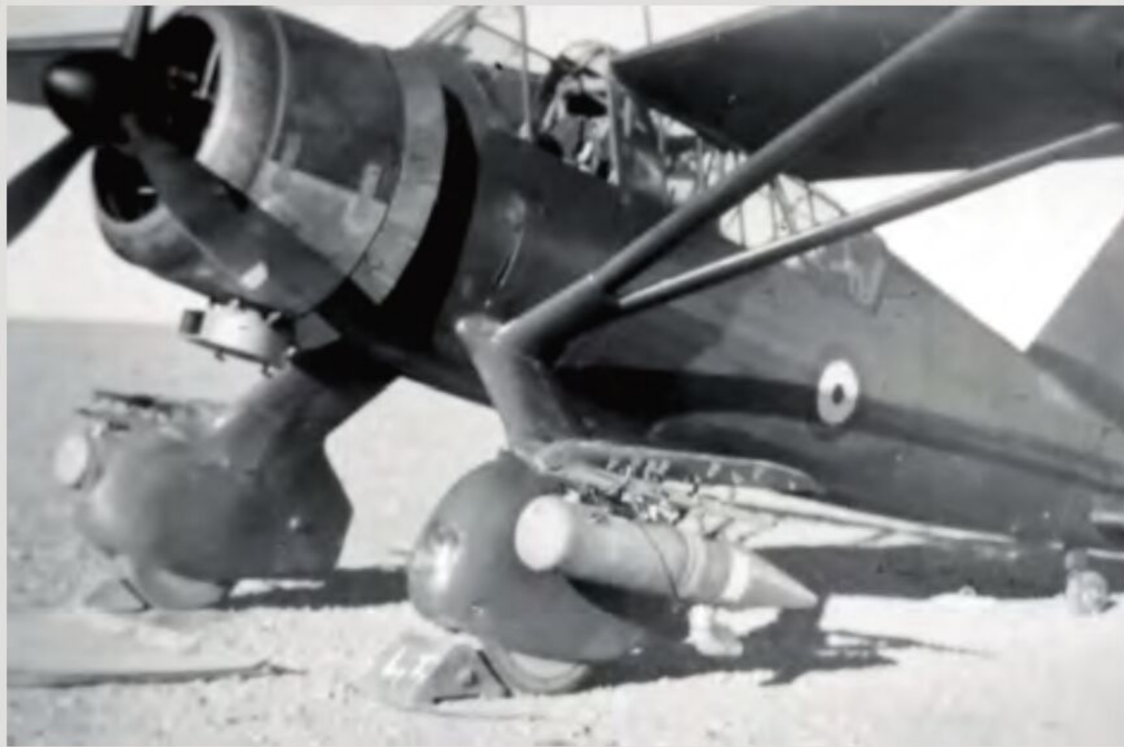
ABOVE THE LYSANDER WAS A VERSATILE AIRCRAFT MADE FAMOUS BY ITS CLANDESTINE MISSIONS INTO OCCUPIED EUROPE. HOWEVER, THIS AIRCRAFT HAS BEEN FITTED WITH GAS SPRAYING EQUIPMENT FOR TESTING IN 1940. ANOTHER WAS TRIALLED WITH TWO 20MM CANNON FOR ATTACKING INVASION BARGES THE NATIONAL ARCHIVES AVIA15/254
