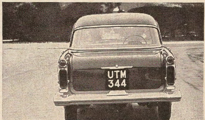
CLEAN, smooth boot lid and wrap-round bumpers give a new look to the Victor back.
