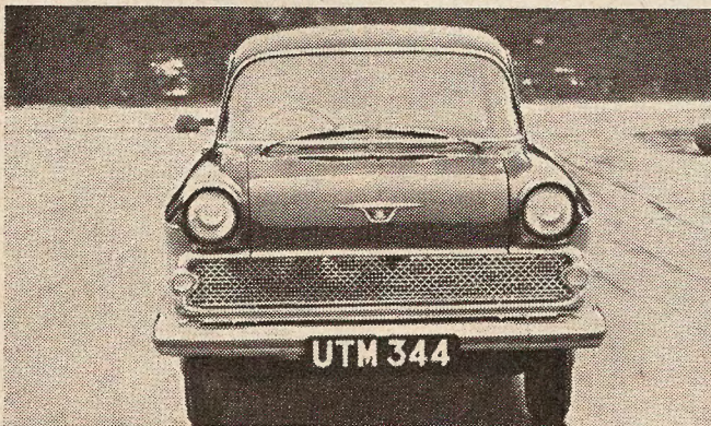
NEW front end treatment on the Victor includes new grille and grille surround.
