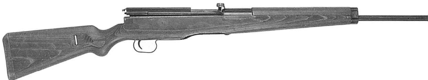
37. Right side view of an incomplete Gerät 07, von Lossnitzer's "final solution", known at the factory as the G44(M). This arm was looted from the Mauser factory by the French, and is now held in a French military museum.
