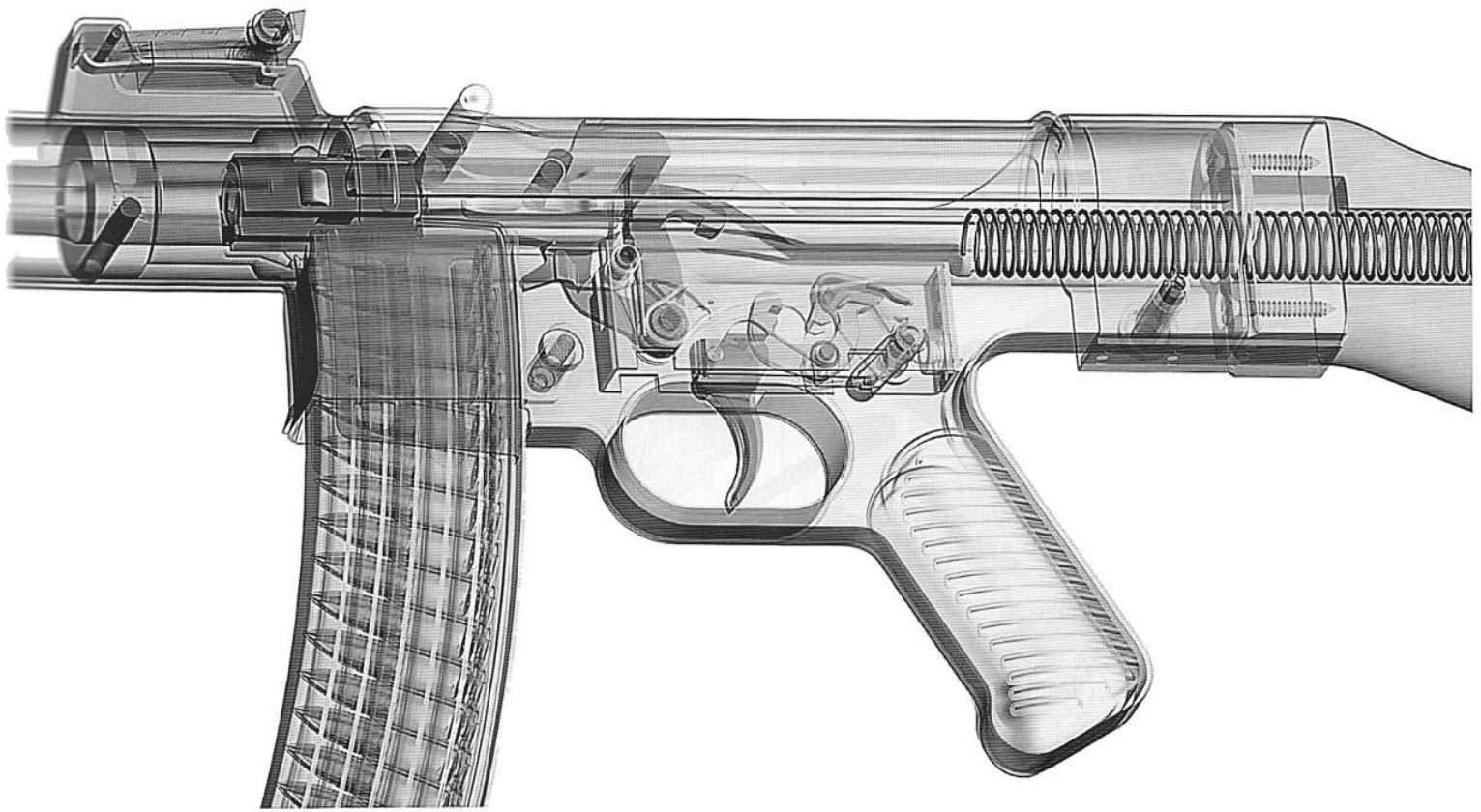
68. An enlargement of the central portion of the phantom view in fig 67 shows the action components of the Gerät 06H/StG45(M) in greater detail.
