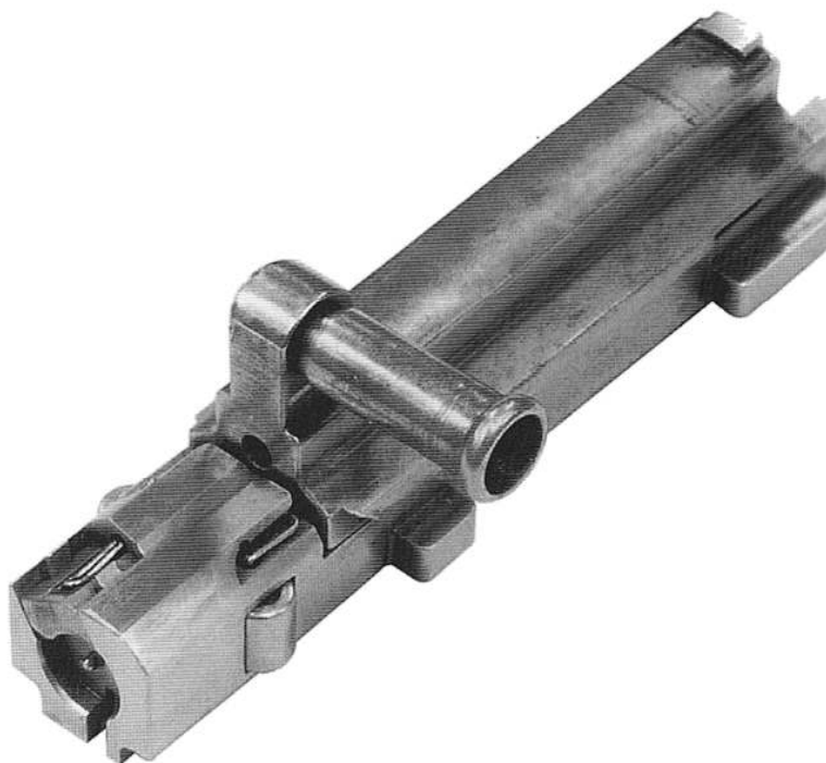
13. Left front three-quarter view of the Gerät 03 bolt assembly, shown in the fired position with the rollers extended and the firing pin forward.
