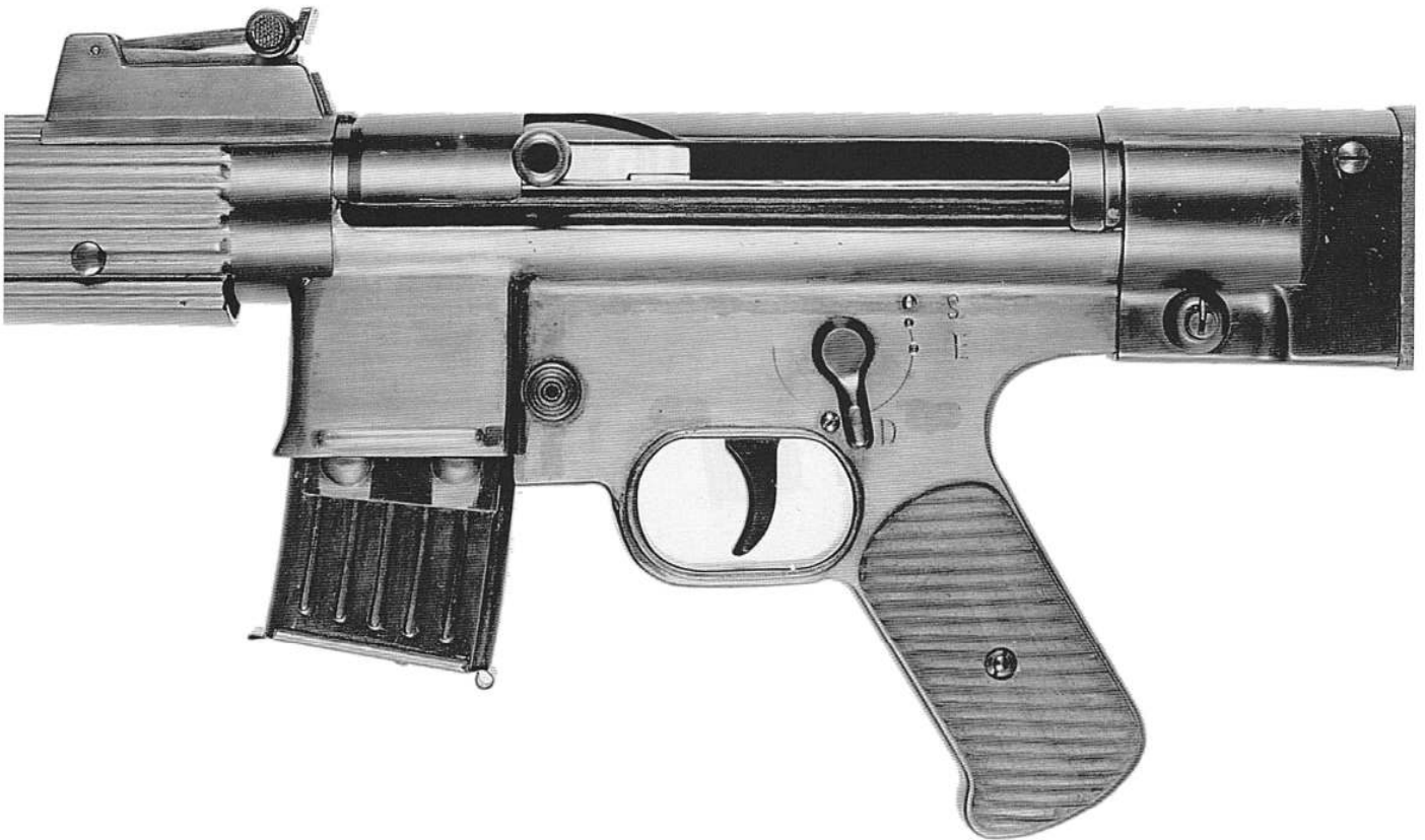
80. Left side closeup of the action of one of the two Vollmer "Gerät 06H" rifles.
