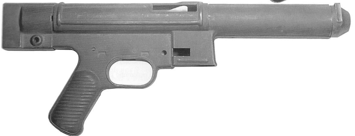
66. Left and right side views of all that remains of a further Gerät 06H parts set, consisting only of a receiver casing, dust cover and butt ferrule.
