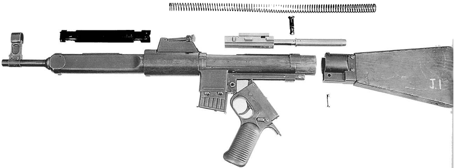
21. Left side view of Gerät 06 serial no 3, shown partially stripped. Note the stamped metal gas system cover plate, at top left. MoD Pattern Room collection,
