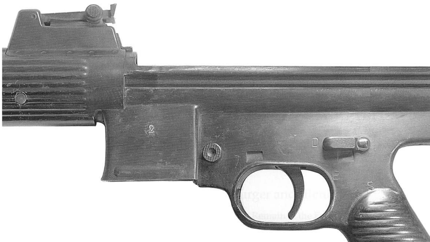
59. Left side closeup of Gerät 06H/StG45(M) serial no 2, showing number "2" stamped on magazine housing. The only other markings are to indicate the selector positions "D" ( Dauerfeuer ; automatic fire) "E" ( Einzelfeuer ; single fire) and "S" ( Sichert ; safe).
