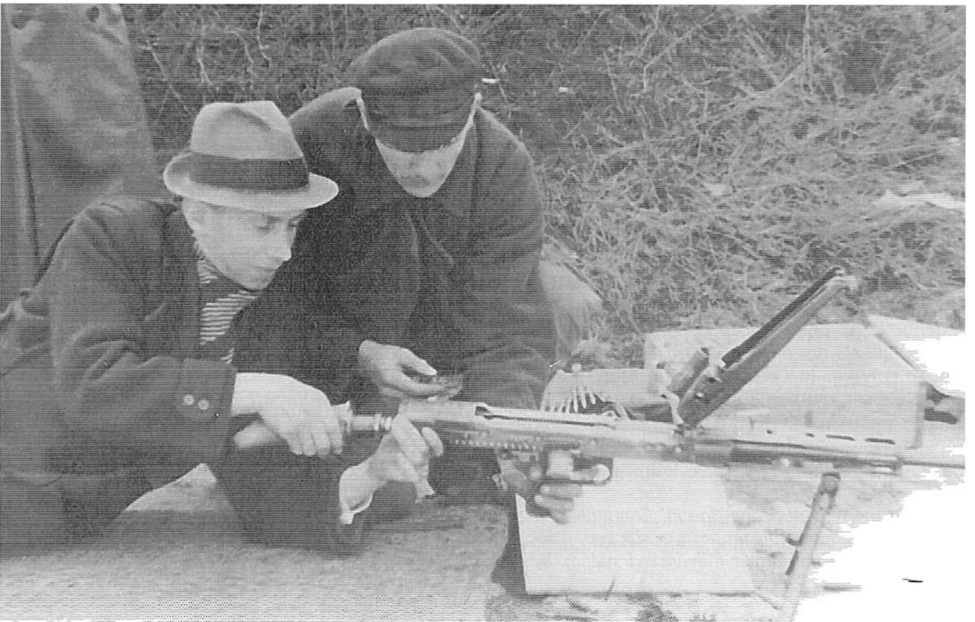
101. Another historic photo showing Dr Gruner firing his roller-locked MG42V prototype assisted by a labourer named Laube. It is posited that the observer at top left is Colonel Otto Morawietz.
