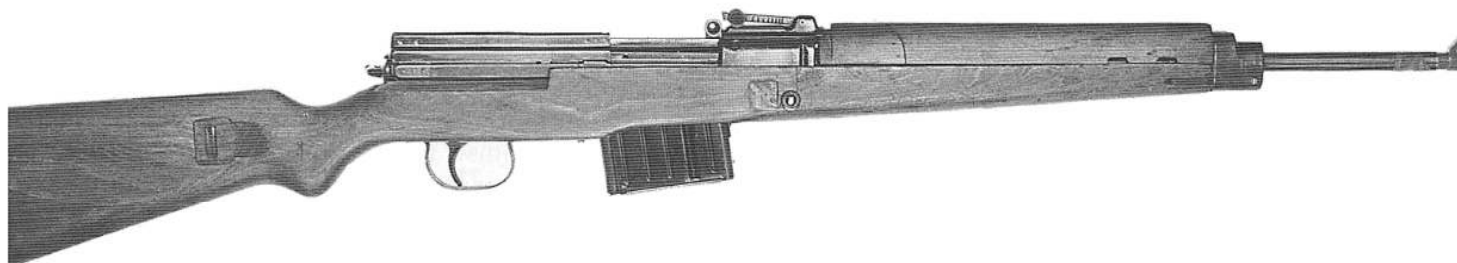
12. Right side view of a Gerät 03, a gas-operated Walther G43 fitted with the Mauser roller lock.
