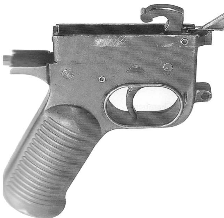
24. Left side closeup of Gerät 06 serial no 3. The buttstock assembly and its locking pin have been removed. The selector is set to "E" (Einzelfeuer; single fire). MoD Pattern Room collection, photo by Richard Jones
