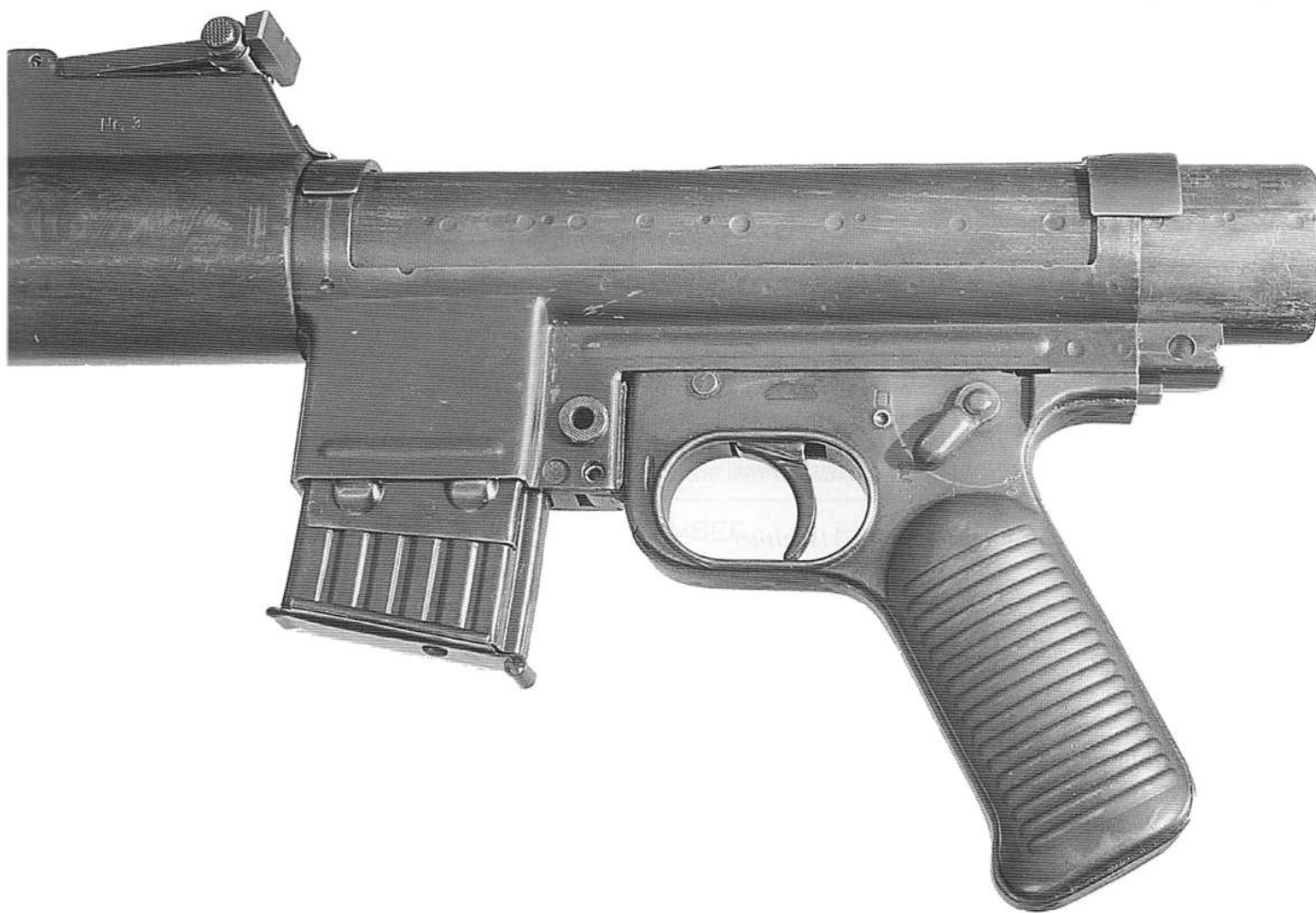
24. Left side closeup of Gerät 06 serial no 3. The buttstock assembly and its locking pin have been removed. The selector is set to "E" (Einzelfeuer; single fire). MoD Pattern Room collection, photo by Richard Jones
