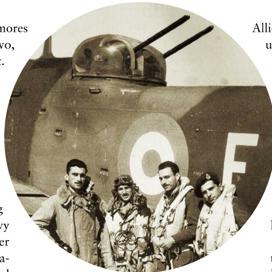
Greek flyers of Royal Air Force Squadron 13—part of Greece’s Royal Hellenic Air Force serving in exile with the Brits—stand beside their Baltimore V, with a Martin-built electric dorsal machine-gun turret.
