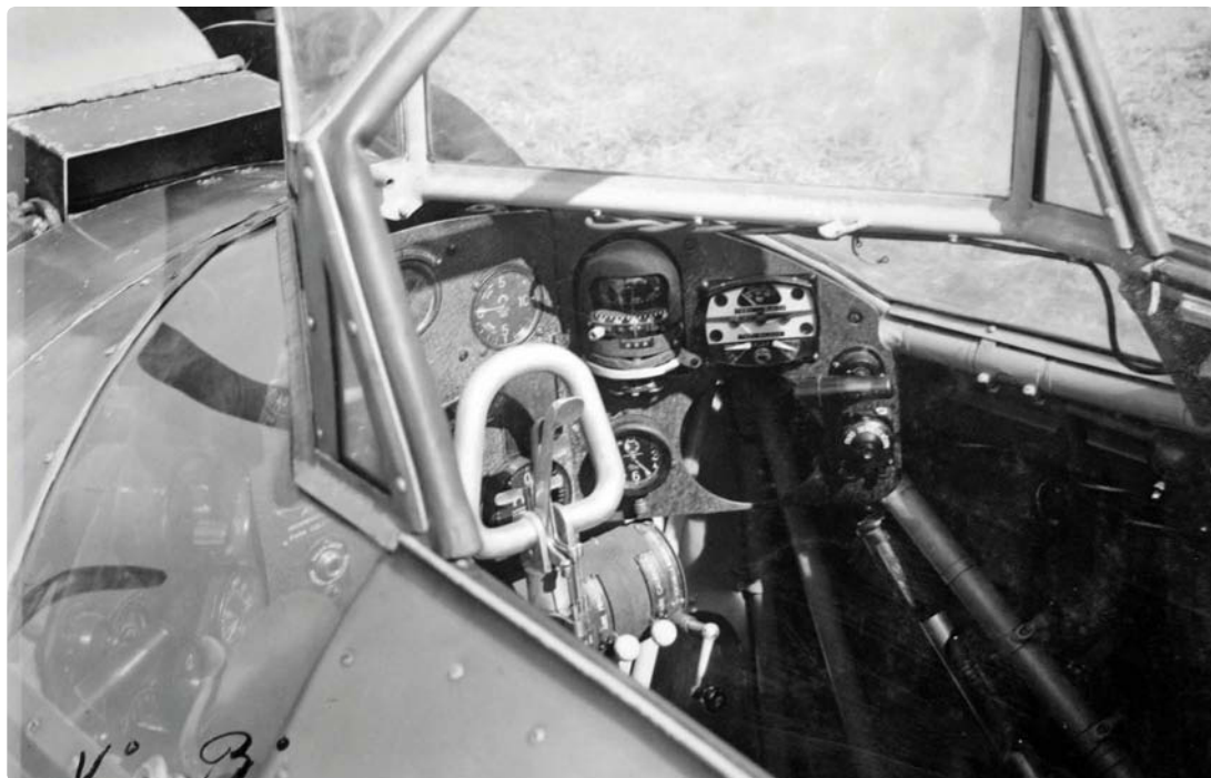
ABOVE The somewhat cramped cockpit of the Ba.65. The control column, fitted with a spade grip, was equipped with a central lever for the compressed-air system that operated the undercarriage and weapons bay doors, and the smaller levers placed either side of the central lever were the firing buttons for the four wing-mounted guns.
