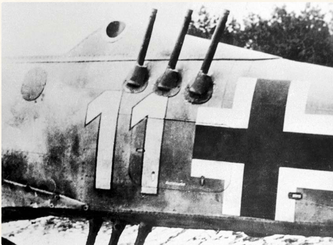
ABOVE The three 1.6m (5ft 3in)-long 30mm cannon barrels of an SG 116 Zellendusche automatic recoilless anti-bomber device installed in the fuselage of Fw 190 "White 11" in mid-1944. If a mass is discharged to the rear of a gun at the same instant that a shell is fired forward from the barrel, the reaction of one will balance out the other.
