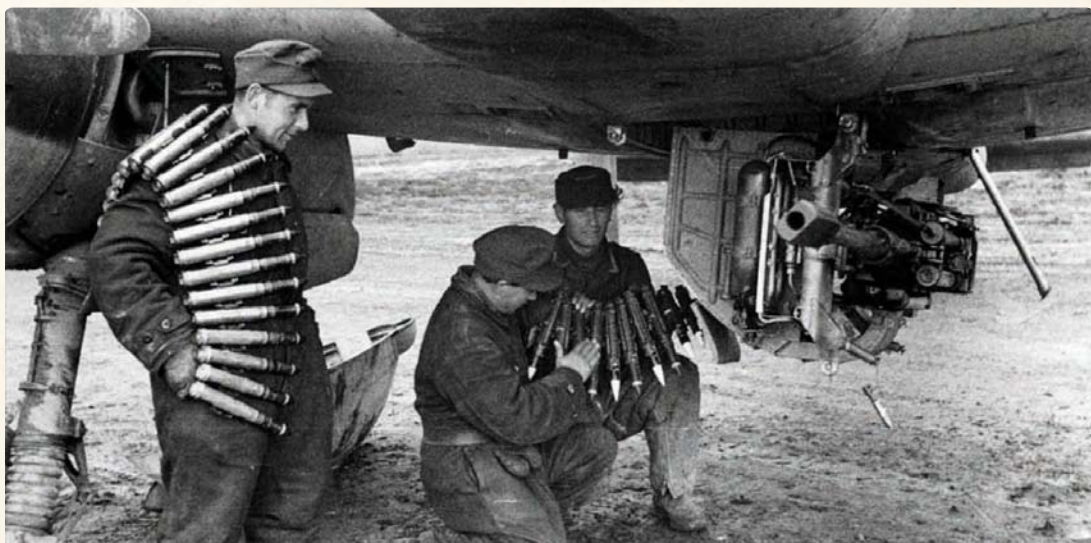
ABOVE Luftwaffe armoureders load the ammunition for an MK 103 cannon fitted to a Henschel Hs 129. The MK 103 was intended principally for combat at ranges beyond 1,000m (3,300ft) and was considered good for operations against enemy bombers. It was the most sophisticated of the 30mm range of weapons used by the Germans.
