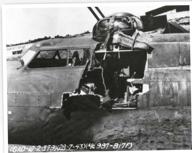
ABOVE A pair of Messerschmitt Bf 110G-2s of ZG 76 fitted with twin mortar sets on each wing head off in search of prey. LEFT The damage inflicted on B-17F 42-29997 The Sack of the Eighth Air Force's 379th Bomb Group, by a W.Gr.21 during a raid on Kassel and Oschersleben on July 28, 1943. The blast from the mortar caused the bomber's oxygen bottles to explode, but the Fortress managed to return to the UK safely.
