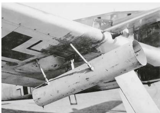
TOP Focke-Wulf Fw 190A-5 WNr 1372, "White 4", was used extensively for static firing trials, and is seen here with its tail jacked up and a W.Gr.21 mortar attached to the starboard wing. ABOVE LEFT & RIGHT The aerial mortar was a relatively simple device that could propel a projectile at a comparatively low velocity over a short range.
