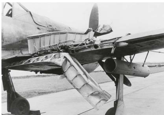
TOP A dramatic photo capturing the moment a mortar is launched from “White 4” during a static test at Barth in early 1944. ABOVE LEFT The results — “White 4” suffered major blast damage to the trailing edge of its wing and control surfaces, although it was repaired and used again. ABOVE RIGHT A close-up of a “twin-stovepipe” fitted to an Me 410. The primary objective was to break up bomber formations rather than destroy individual aircraft.
