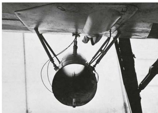
TOP Focke-Wulf Fw 190A-5 WNr 1372, "White 4", was used extensively for static firing trials, and is seen here with its tail jacked up and a W.Gr.21 mortar attached to the starboard wing. ABOVE LEFT & RIGHT The aerial mortar was a relatively simple device that could propel a projectile at a comparatively low velocity over a short range.
