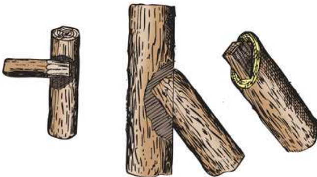
▲ Join the rails of the footbridge to the posts as shown here.
