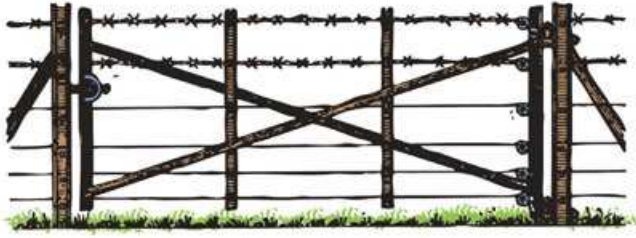
▲ This wire gate is hung on ordinary iron posts. The heel of the gate, made of angle iron, is fitted with winding brackets for tightening the wire bars.
