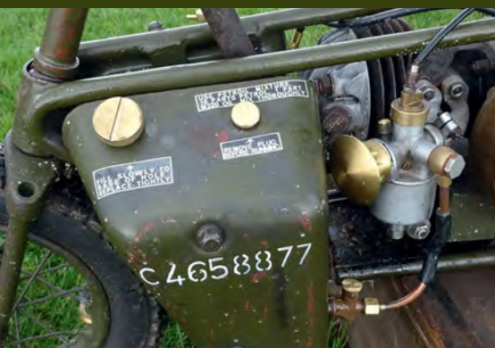
The pressurised tanks hold just under a gallon of petrol giving a maximum range of 90 miles
