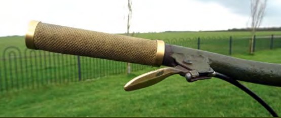
Original brass and canvas twist grip handlebars and clutch lever. The clutch plate itself is made from cork
