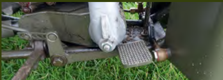
As there is only a foot-operated rear brake and no lights, these motorbikes are not road legal
