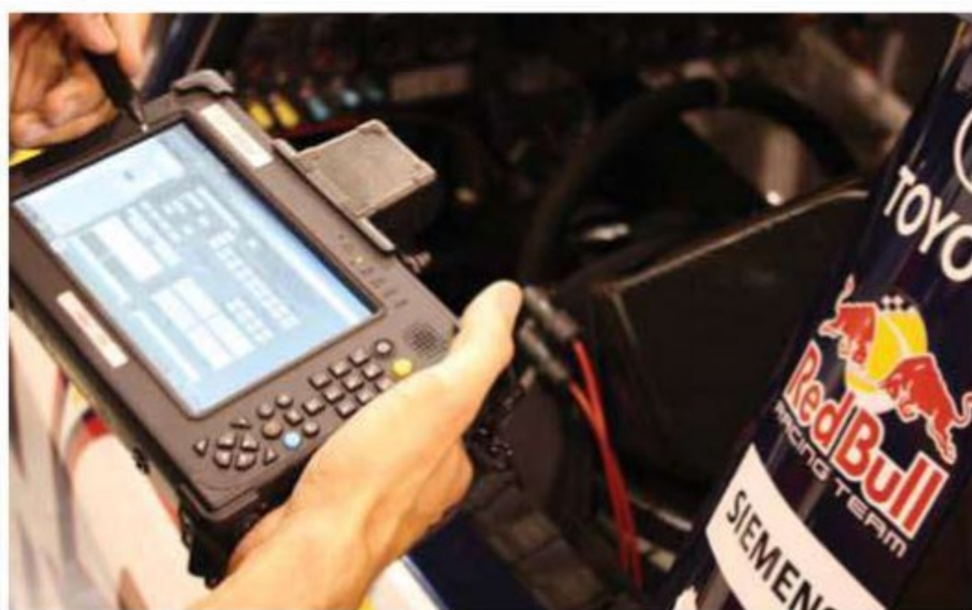
Data can be downloaded directly from the racecar and immediately sent to the servers in the race transporters, and to component manufacturers
