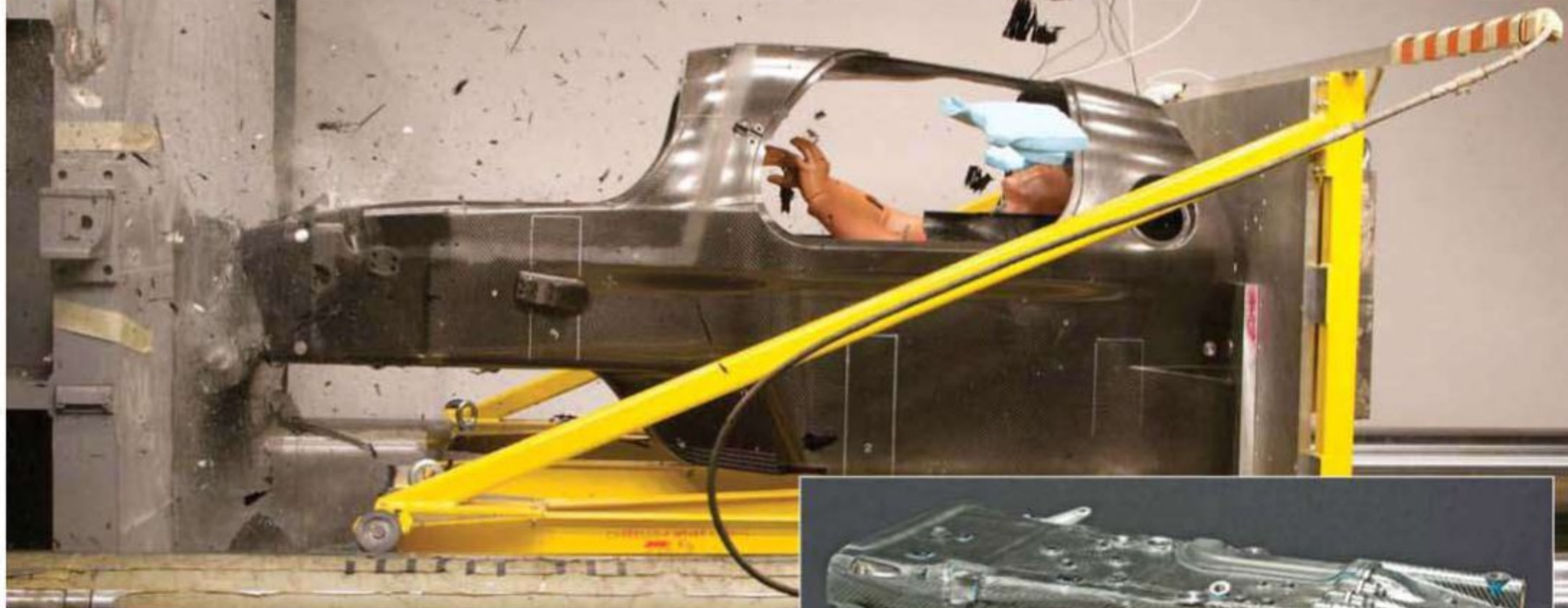
Weight saving was a critical part of the new R18's design, which went as far as a new lighter and stiffer monocoque than in 2011
