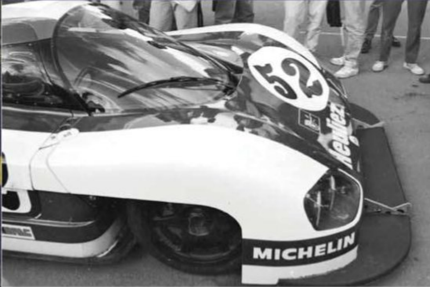
With the front bodywork 70mm wider than the front track, the WM's steered wheels were able to turn inside the overhanging body
