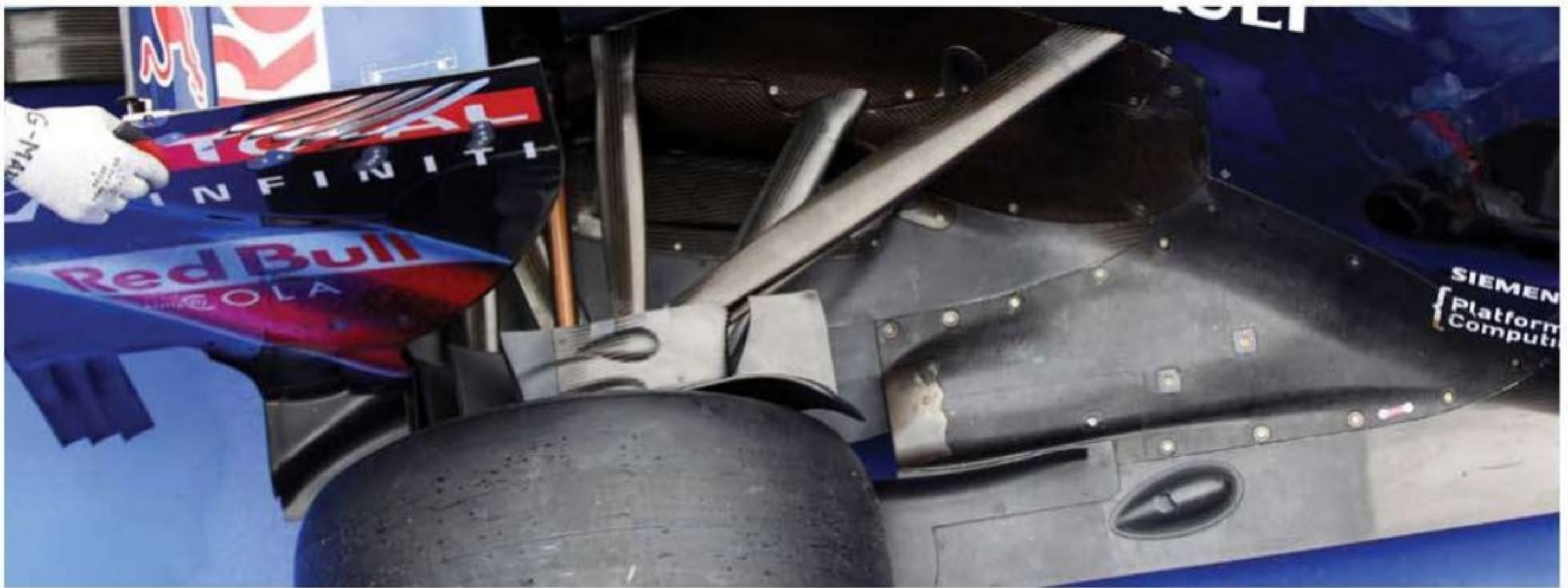
This close-up of the Red Bull exhaust outlet shows how the floor is being blown directly ahead of the rear wheel with the exhaust pointing to the inside edge of the rear tyre to stop the vortex interfering with the flow through the diffuser. Note the cut out just ahead of the wheel where the flow will go down
