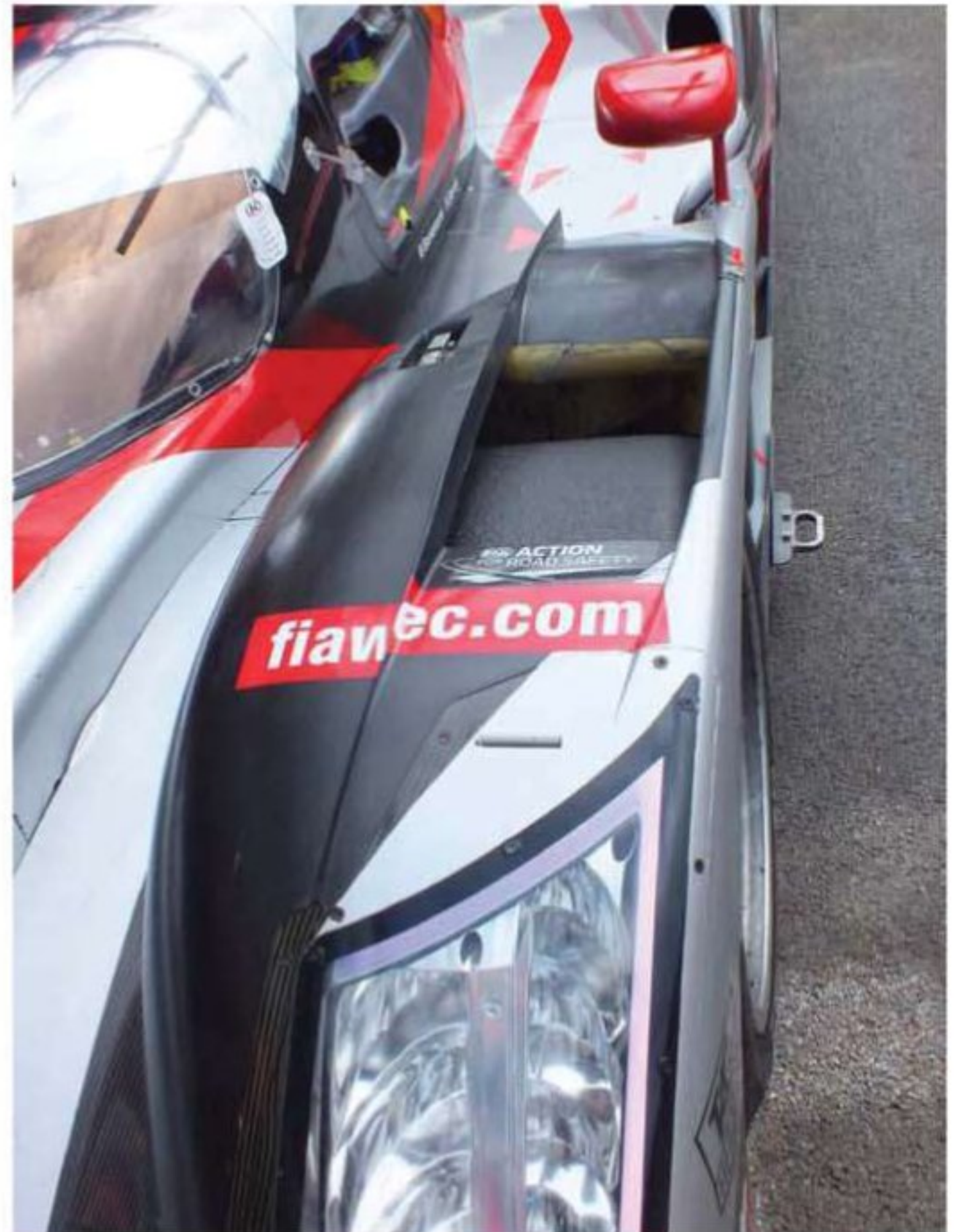
Audi utilises lips both upstream and downstream of the holes to prevent the dirty air from impacting other flow structures across the car
