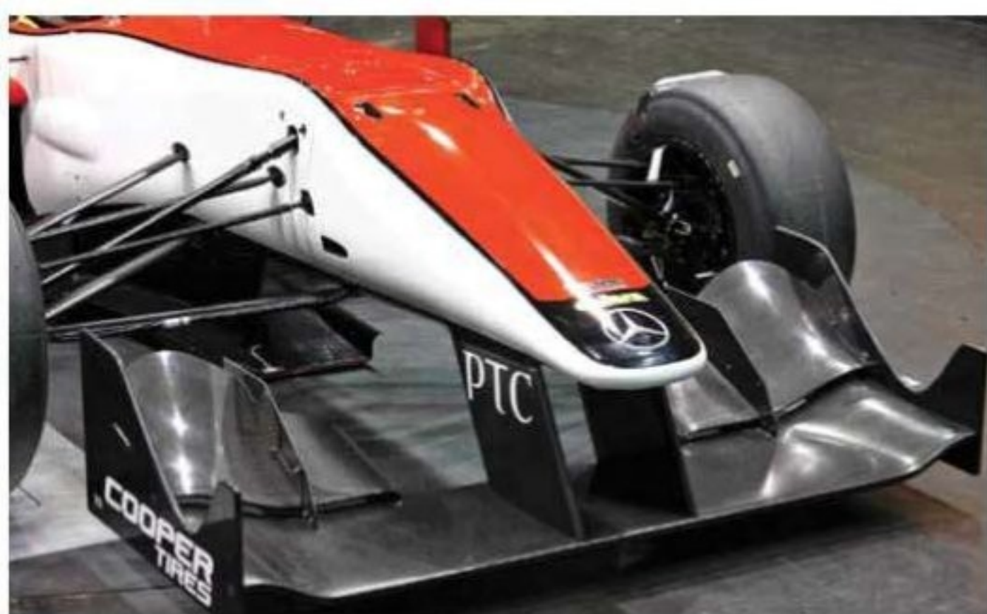
The F312's front wing features a larger main element chord and larger flap area than the previous car's
