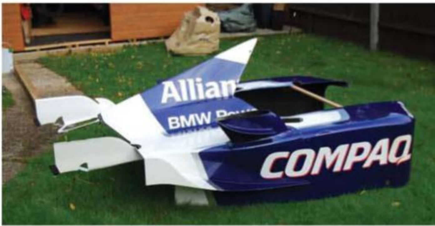
Williams BMW engine cover and sidepods were cut up to make the sidepods
