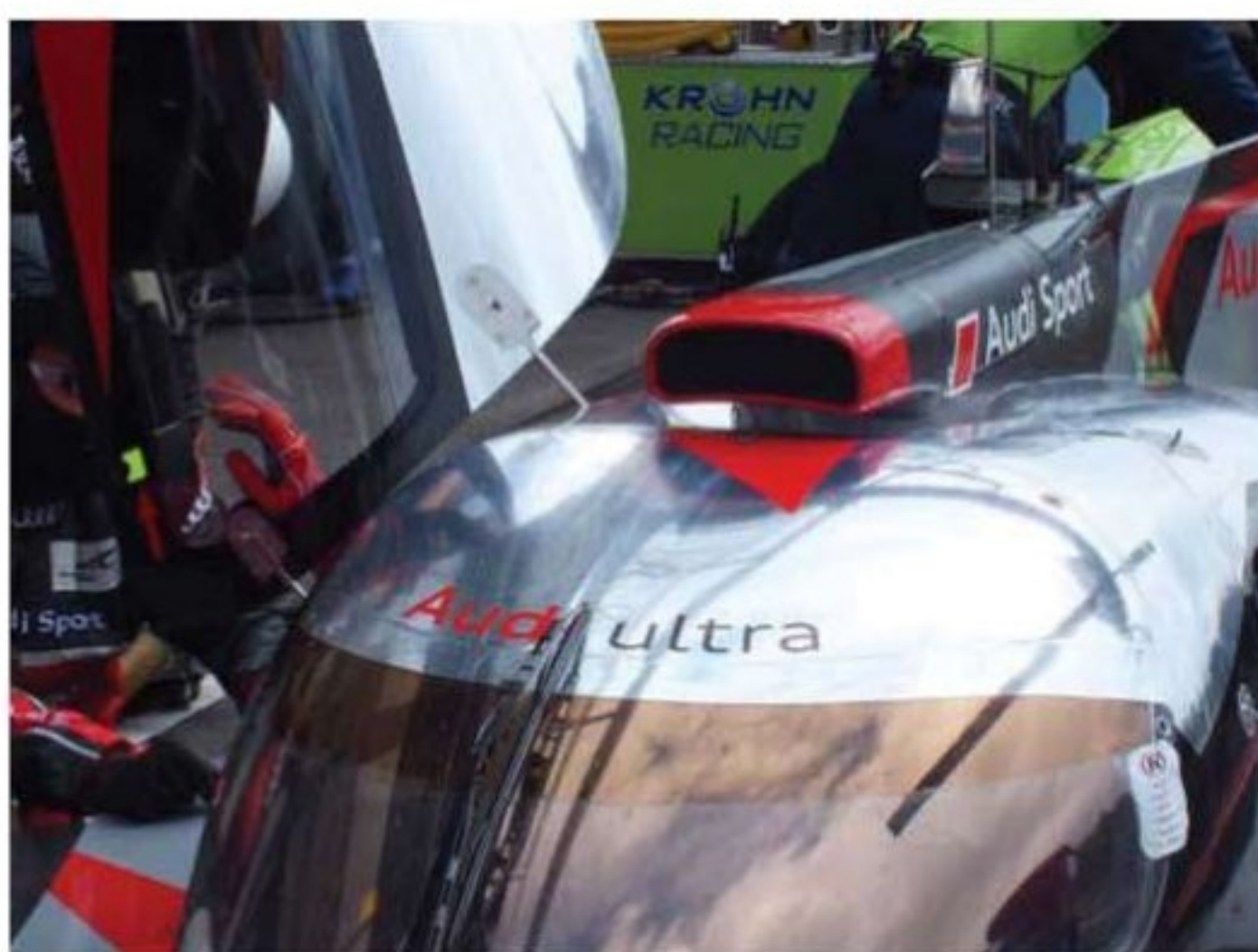
A dimple in the R18's roof is the result of a regulatory change and allows for cleaner airflow to the plenum chamber
