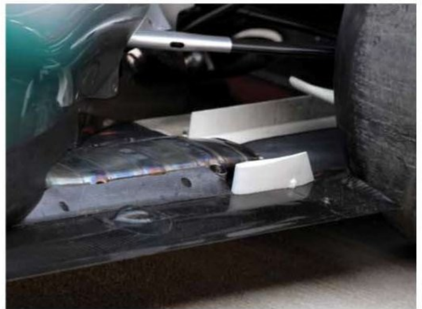
A further iteration of the exhaust blown floor, as seen on the Mercedes, showing the attachments to channel airflow through the diffuser
