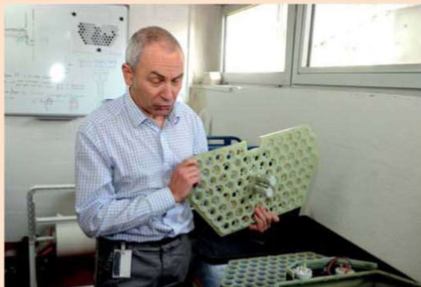
The 90 individual cells in the 350V battery are contained within different layers with aluminium bars connecting them. Peugeot developed a warning light system that informs whether the car is live and / or safe to touch
