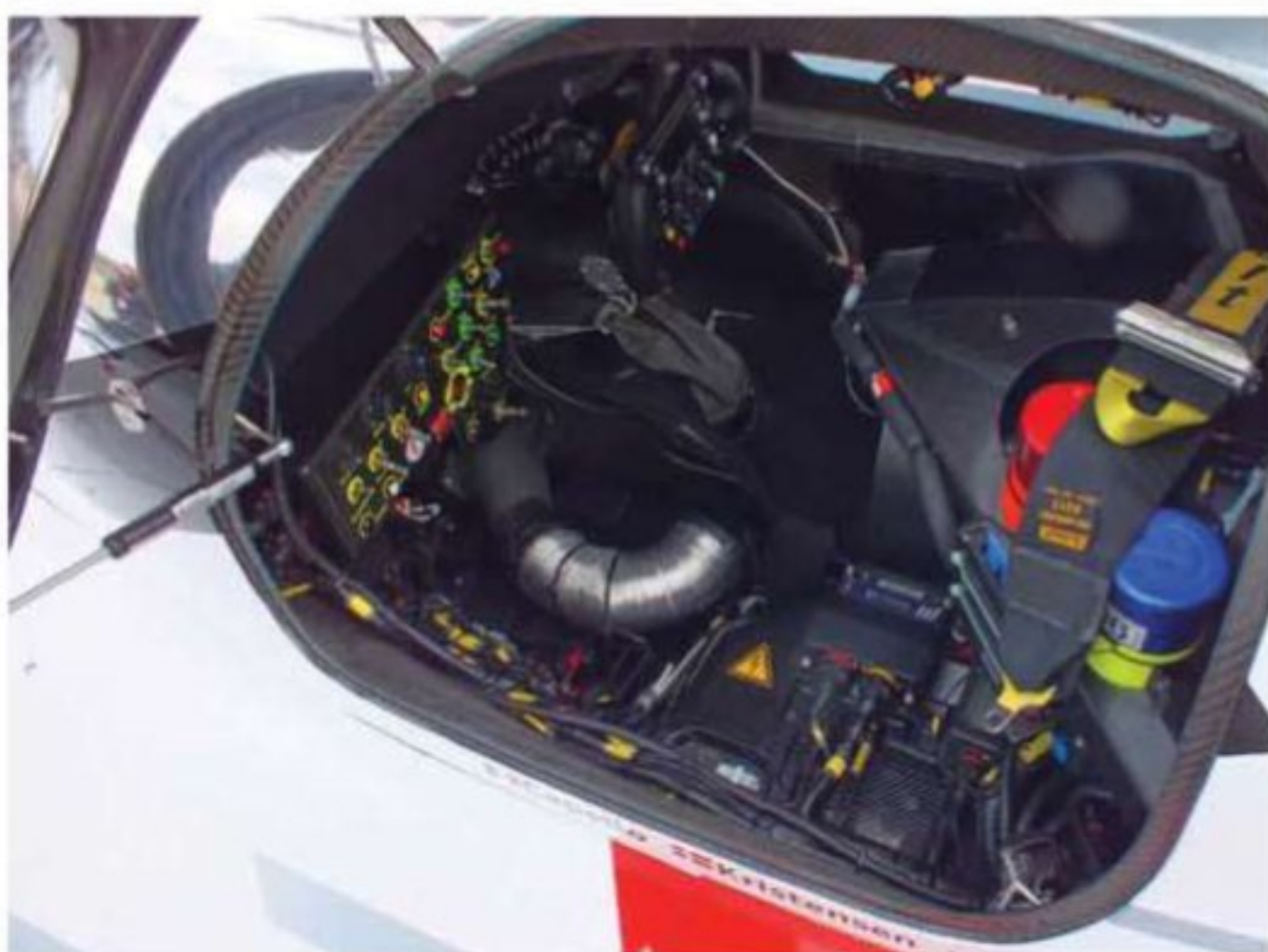
Both Audi (above) and Toyota mount the energy storage systems in the passenger seat area of the cockpit
