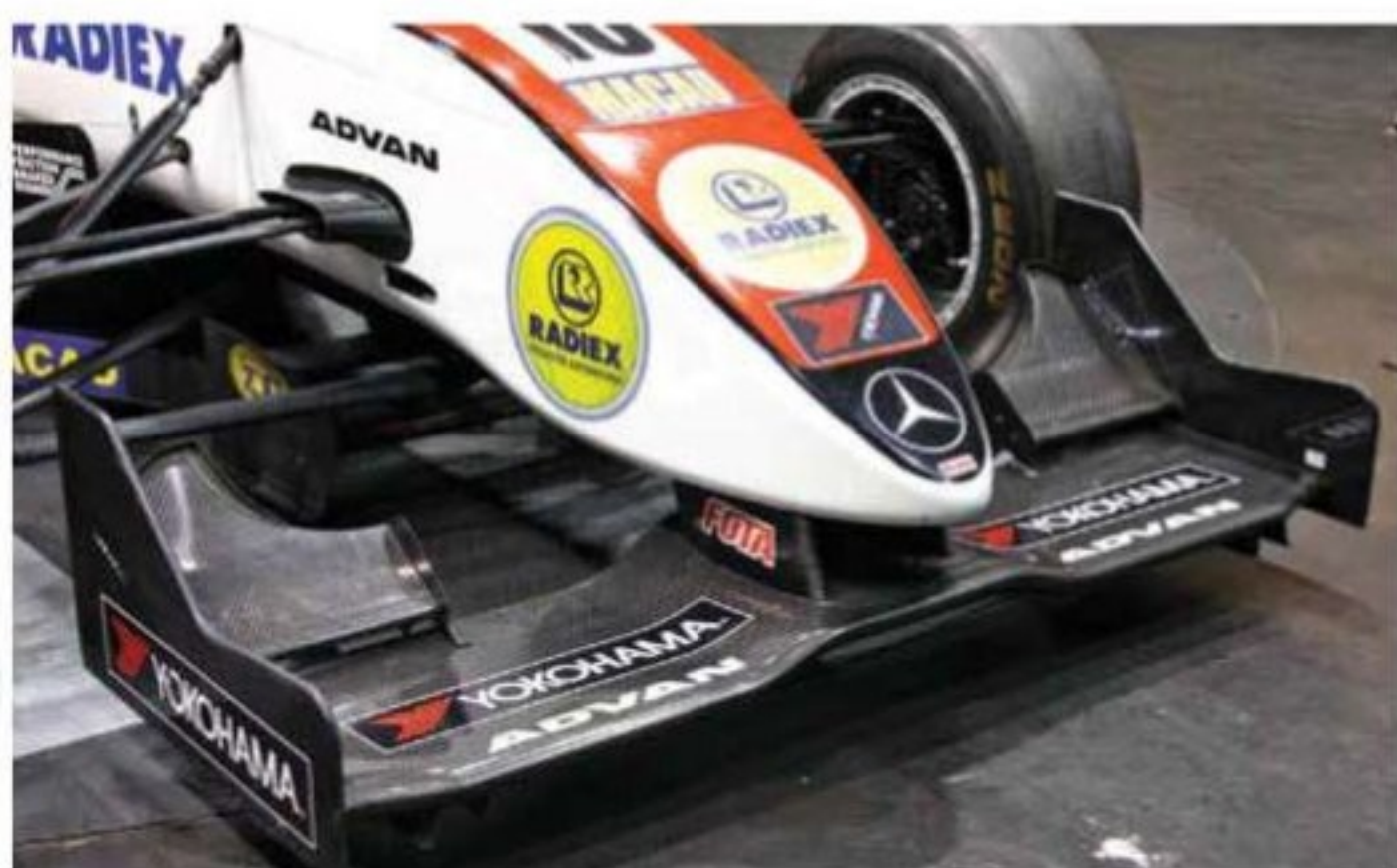
The F308 wing dates back several years, although some teams did add additional flaps inboard and 'bridge' flaps
