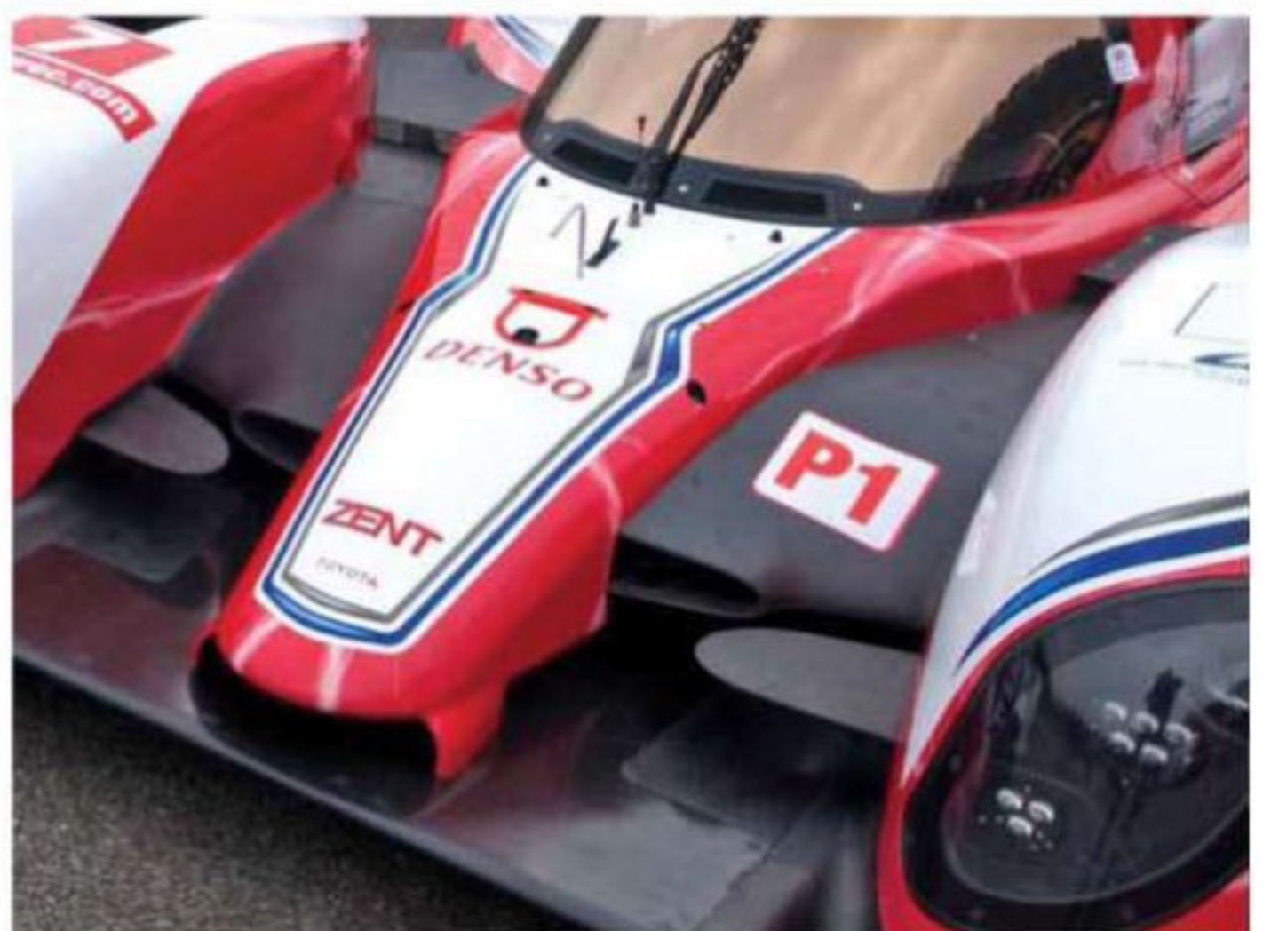
Toyota has heavily revised the front of its TS030, with an F1-inspired nose. LED headlights have also been added to increase brightness
