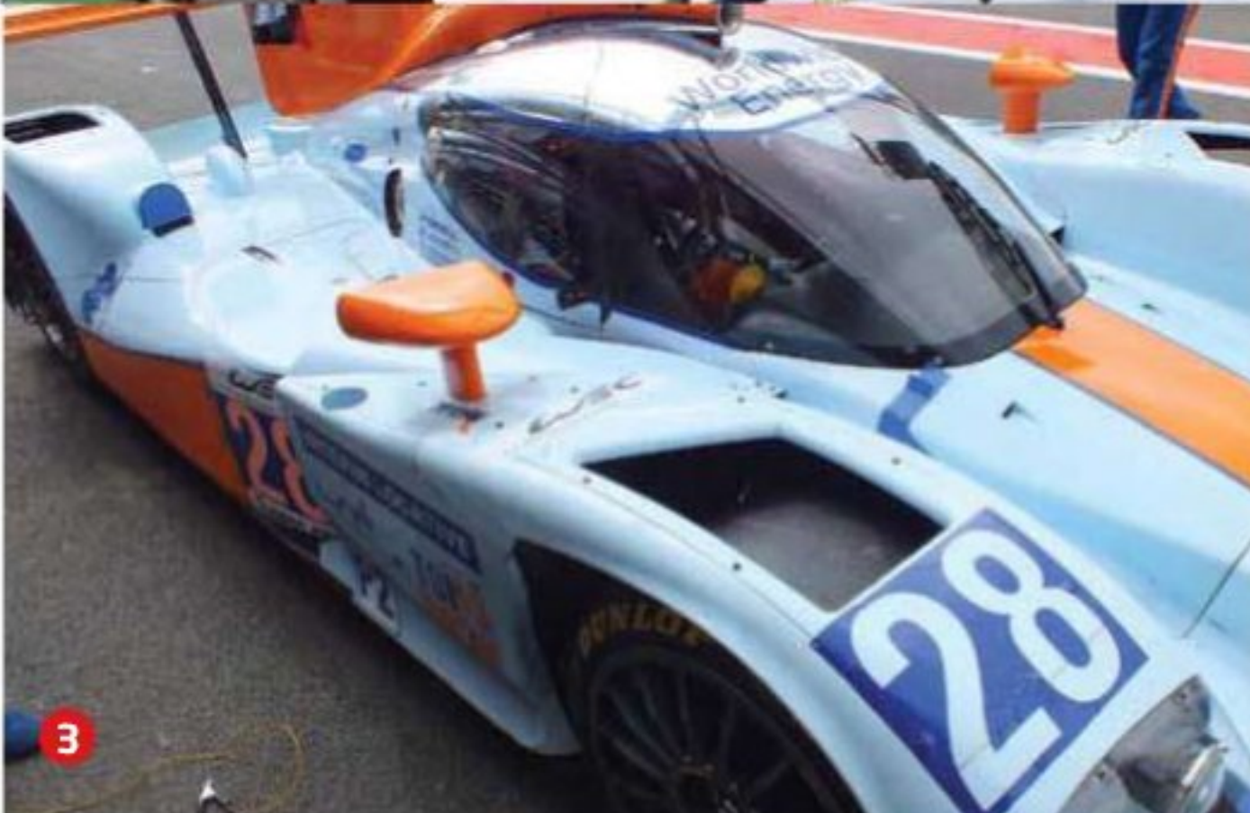
1. Zytek retained some louvres on its air extractors, and added a split exit to smooth the flow 2. Dome ran with an interim solution at Spa similar to the Lola solution 3. The curved tail of the hole is likely to encourage
