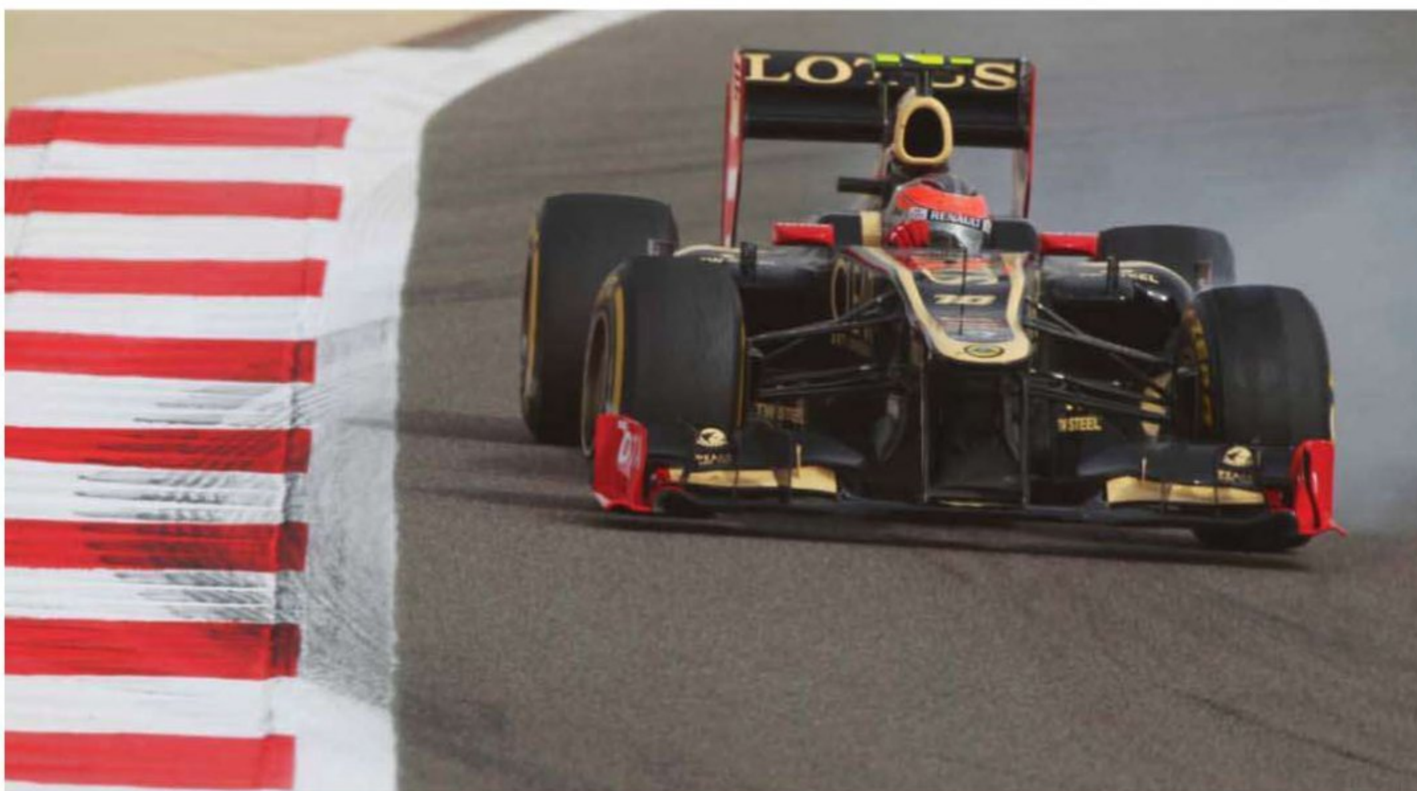
Some Formula 1 cars raise the nose under braking, but 100 per cent anti dive only results in zero pitch if there is also 100 per cent anti lift at the rear
