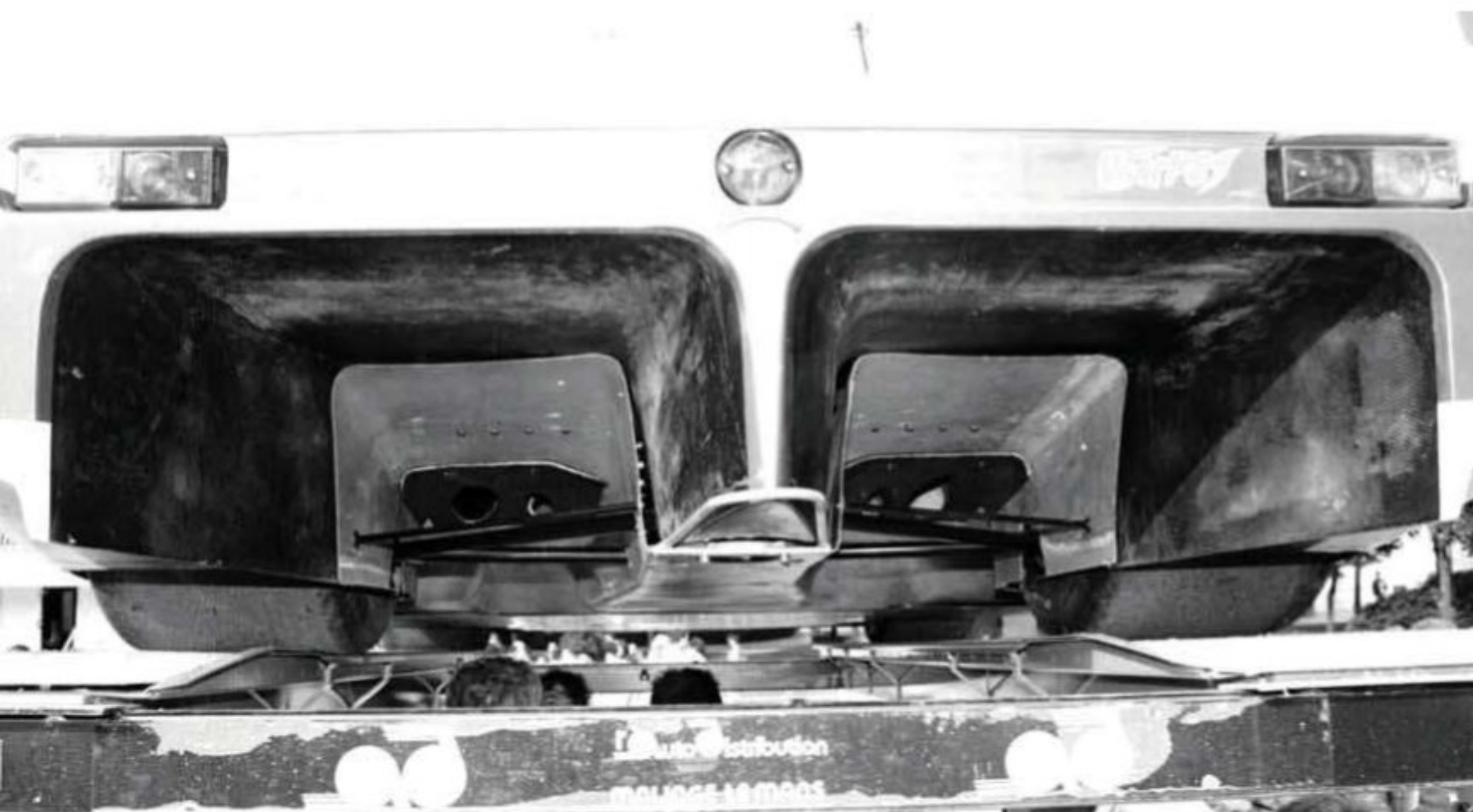
The Le Mans scrutineering hoist reveals the WM's blown, low drag, low downforce underwing
