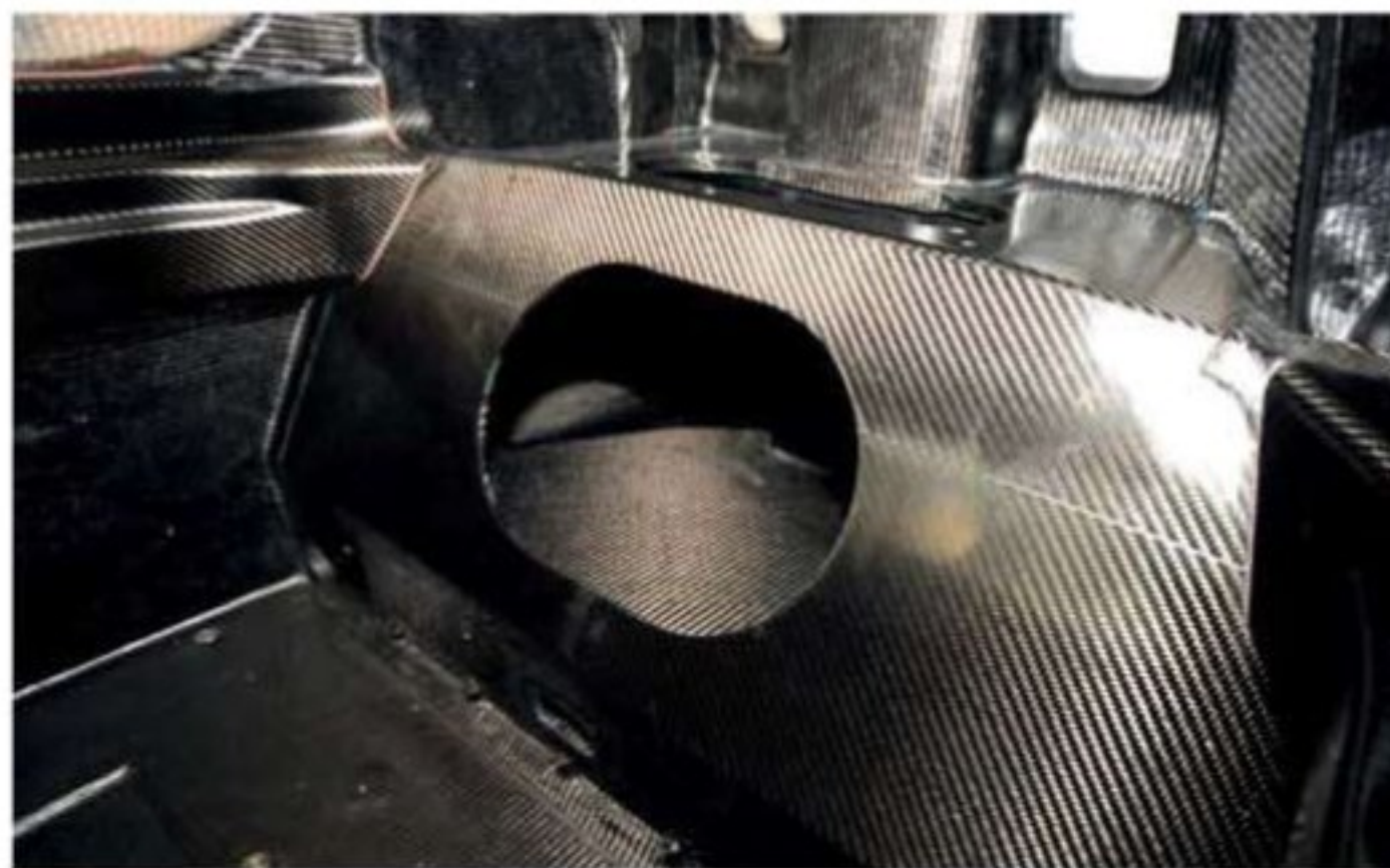
The carbon tub was built by Capricorn to Peugeot's specific design, and here housed the triangular battery
