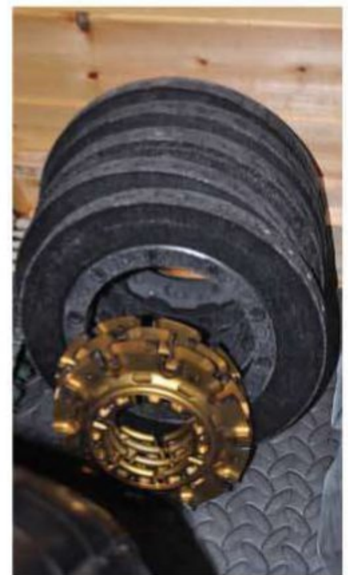
Though a full set of carbon /carbon brakes have been sourced, driver ability dictates the use of steel
