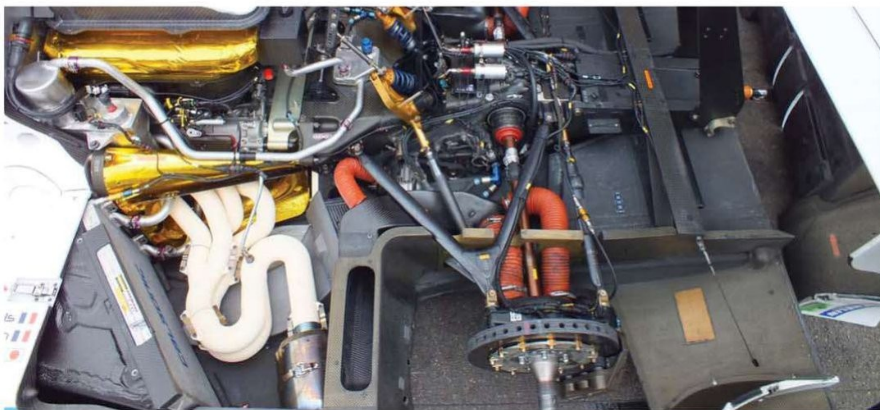
The aerodynamically efficient Dome S102. Current ACO regulations state the floor must be continuous but it does leave scope for exhausts to be exited into the wheelarch, which could increase downforce, even in a cold-blown situation
