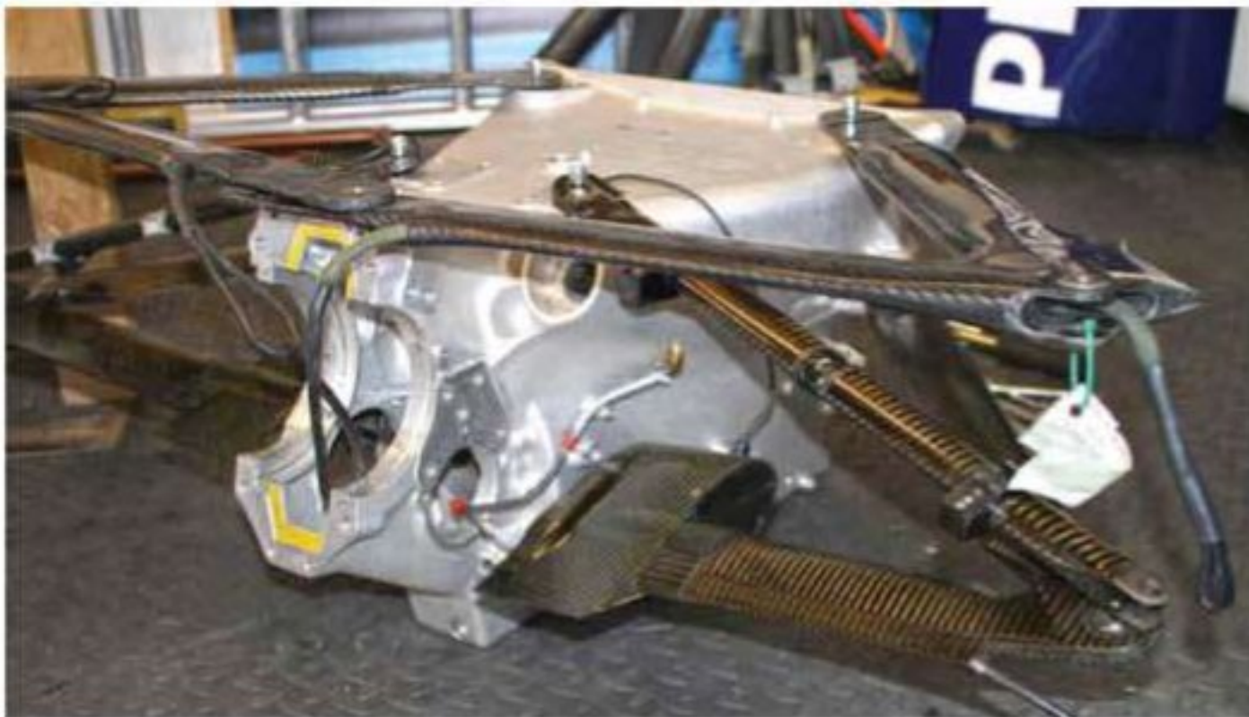
Thomas has amassed a number of suspension components, and plans to use a set of wishbones from a Honda RA107, along with a Hewland FTR gearbox
