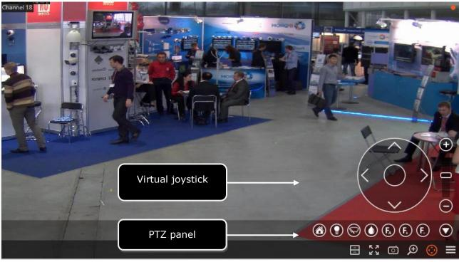
The controls may differ depending on the available camera features. The following elements of the PTZ camera management interface were implemented in Eocortex: virtual joystick, zoom in / out, focus control (+/-/AF), transition to the "home" position, infra-red light control, wiper control.
