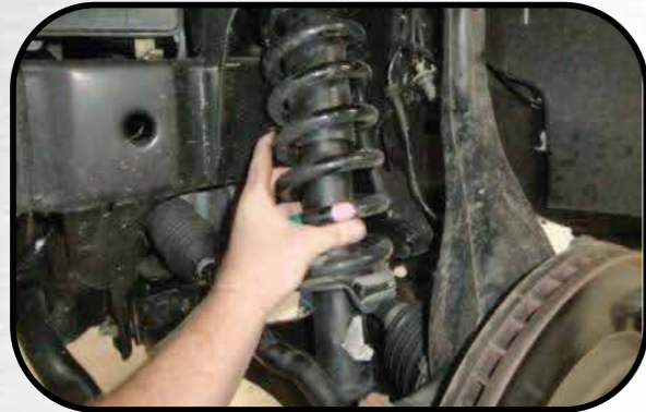
10. Remove strut assembly from vehicle
