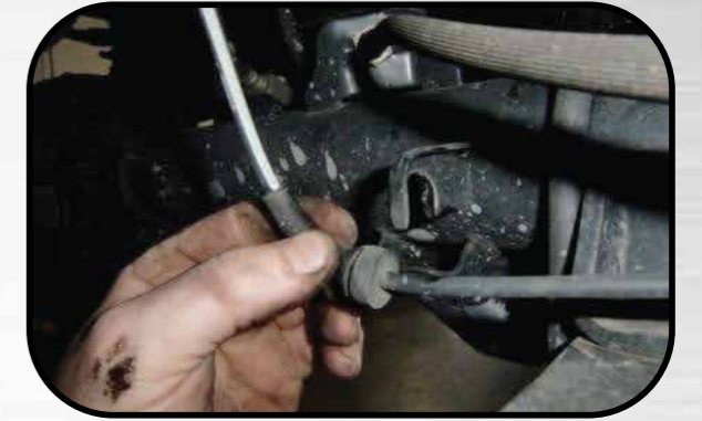
20. Remove ABS lines from attachments on axle
