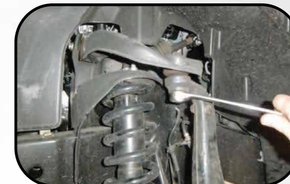
6. Loosen upper ball joint nut, do not remove
