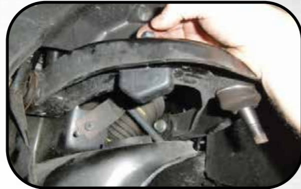
14. Attach bump stop as shown, note bumpstop orientation
