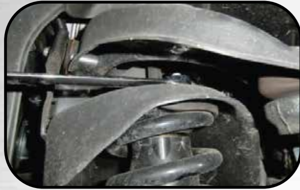
9. Remove upper strut mounting hardware
