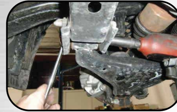
16. Loosen the lower control arm mounting hardware
