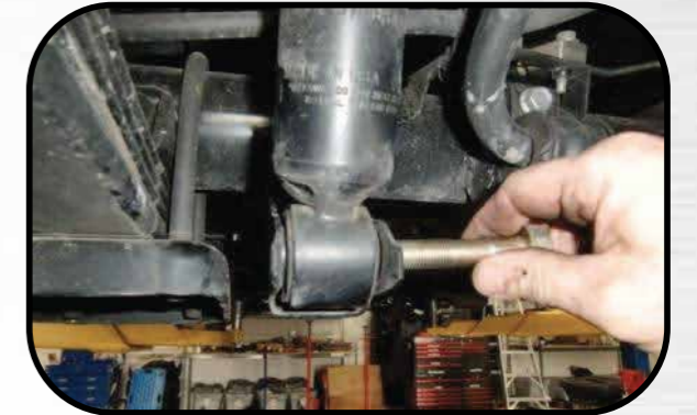
21. Remove lower shock mounting hardware
