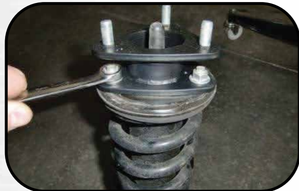
11. Attach strut extension with OEM hardware
