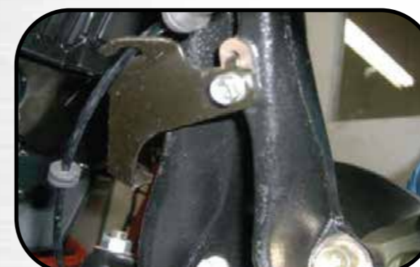
3. Disconnect ABS line bracket behind spindle
