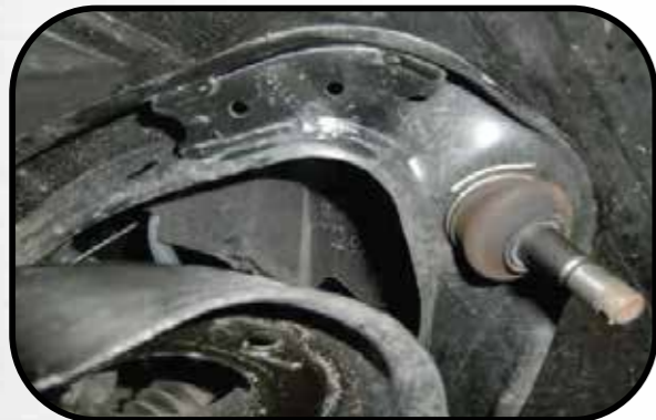
12. Drill 5/16 hole in upper control arm existing hole
