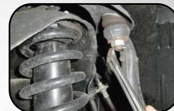
5. Remove cotter pin and upper ball joint
