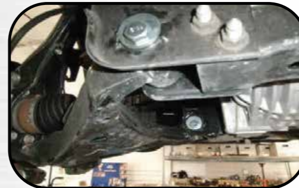
18. Orient cams in the upright/neutral position and tighten
