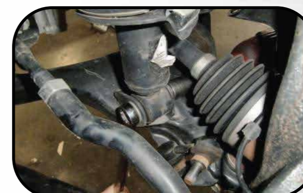
8. Remove lower shock mounting hardware
