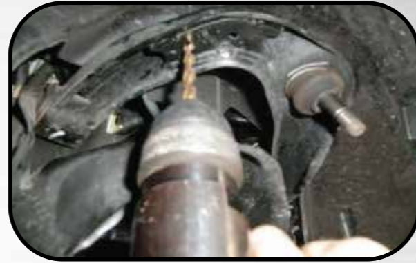
13. Note Drilling Hole
