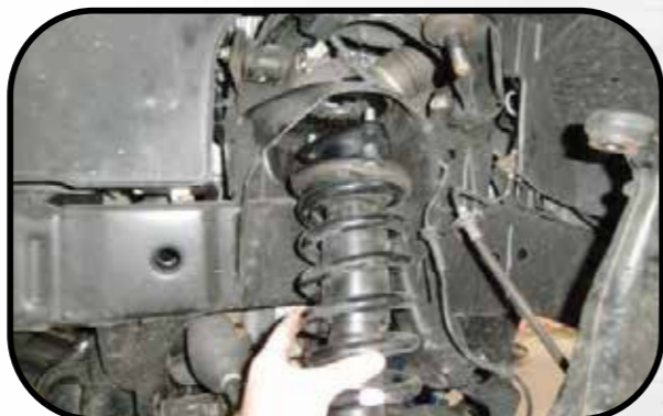
15. Reinstall strut assembly into vehicle with new upper hardware
