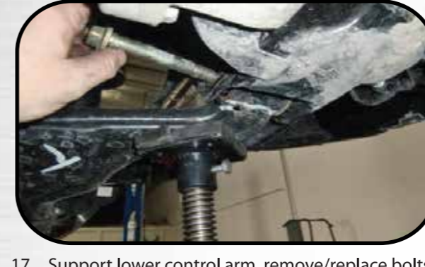
17. Support lower control arm, remove/replace bolts one at a time
