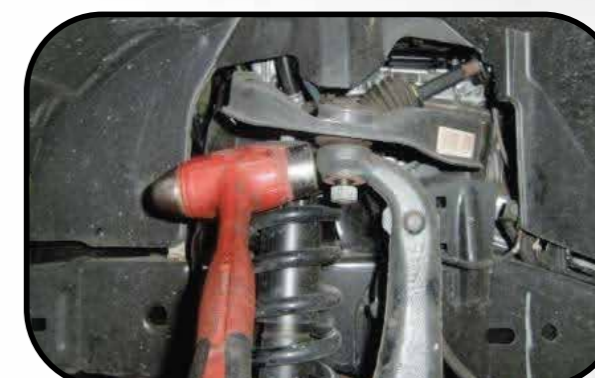
7. Strike spindle to break loose connection
