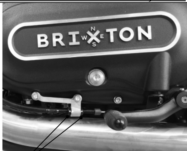
Loosen the nuts and adjust the length of clutch cable
