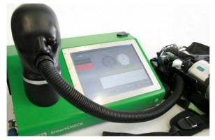
Fig. 44 Connecting adapter hose to test head.
