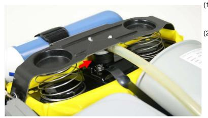
(1) Put the open side of the sealing cap R 22 086 over the plunger.
