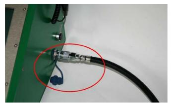
(1) Supply test device with medium pressure 6 - 10 bar.
