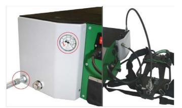
Fig. 32 Connecting high pressure lines
