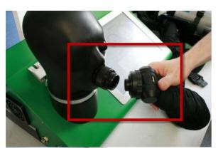
Fig. 47 Connecting breathing hose assembly to test head
