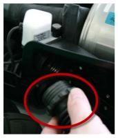
Fig. 46 Screwing adapter into exhalation side
