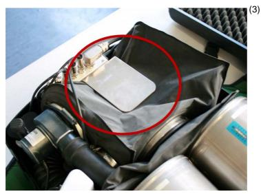
Fig. 48 Blocking surplus valve on exhalation bag
