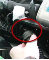
Fig. 45 Screwing adapter into inhalation side
