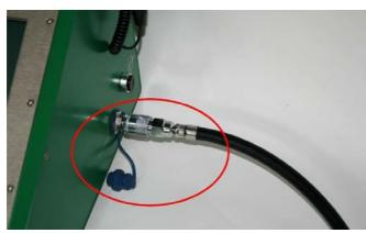
(1) Supply test device with medium pressure 6 - 10 bar.
