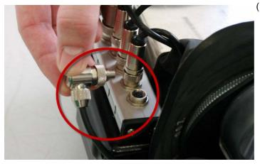
Fig. 43 Disconnecting battery of closed circuit breathing apparatus
