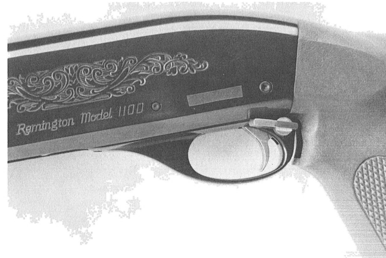
View showing selector at "full auto" position.
