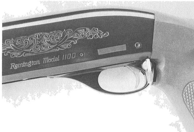
Another left side view showing selector lever on "semiauto" position.
