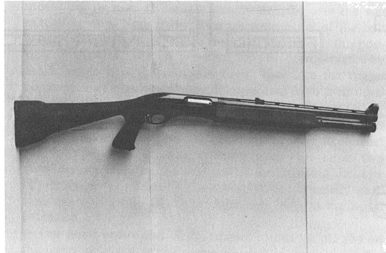
A left side view of the same weapon with its side-mounted sling removed. Note that this still has the original wooden foregrip. The buttstock is an indestructible FN-type plastic material.
