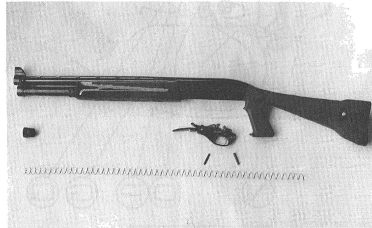
View showing the weapon partially disassembled with the trigger plate assembly and the long magazine spring removed. Note the magazine tube end cap unscrewed for removal of the spring. The original magazine extension was modified so that a custom front sight and end cap can be installed for more sophisticated and faster field stripping.
