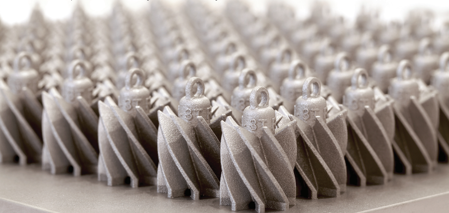
BELOW A build platform of titanium swirlers using metal Additive Manufacturing
