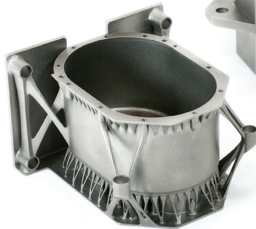
ABOVE & LEFT A metal AM gearbox housing optimised for stress and low mass
