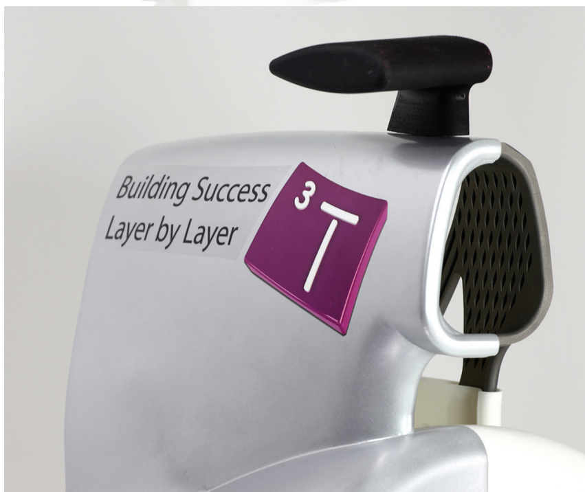
ABOVE & BELOW Even safety-critical, structurally demanding components like this titanium alloy roll hoop can now be 3D printed
