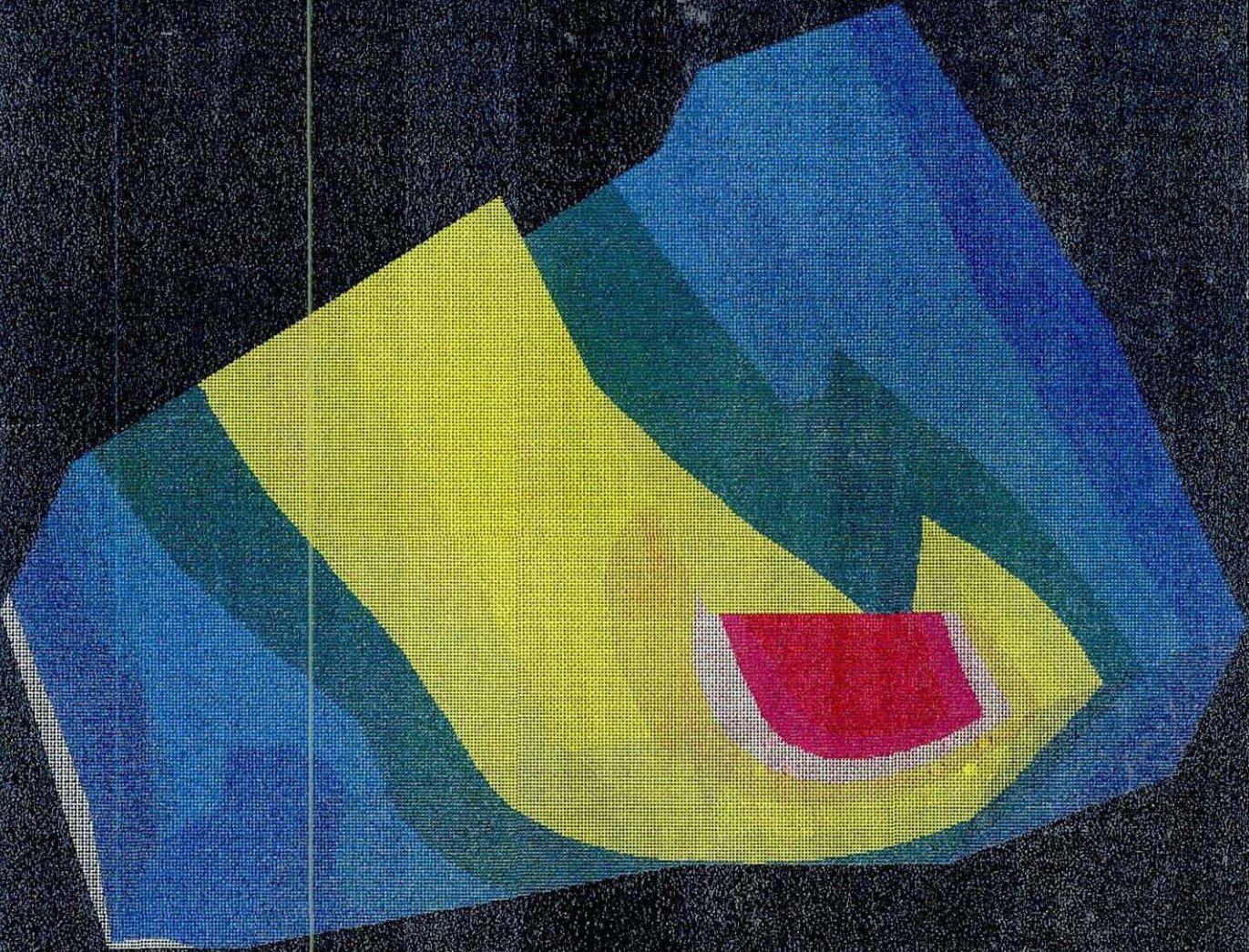
FIG 33 - TRUNNION DEFLECTION RESULTS (FIRING LOAD)
