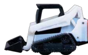
*T590 Compact Track Loader w/bucket
