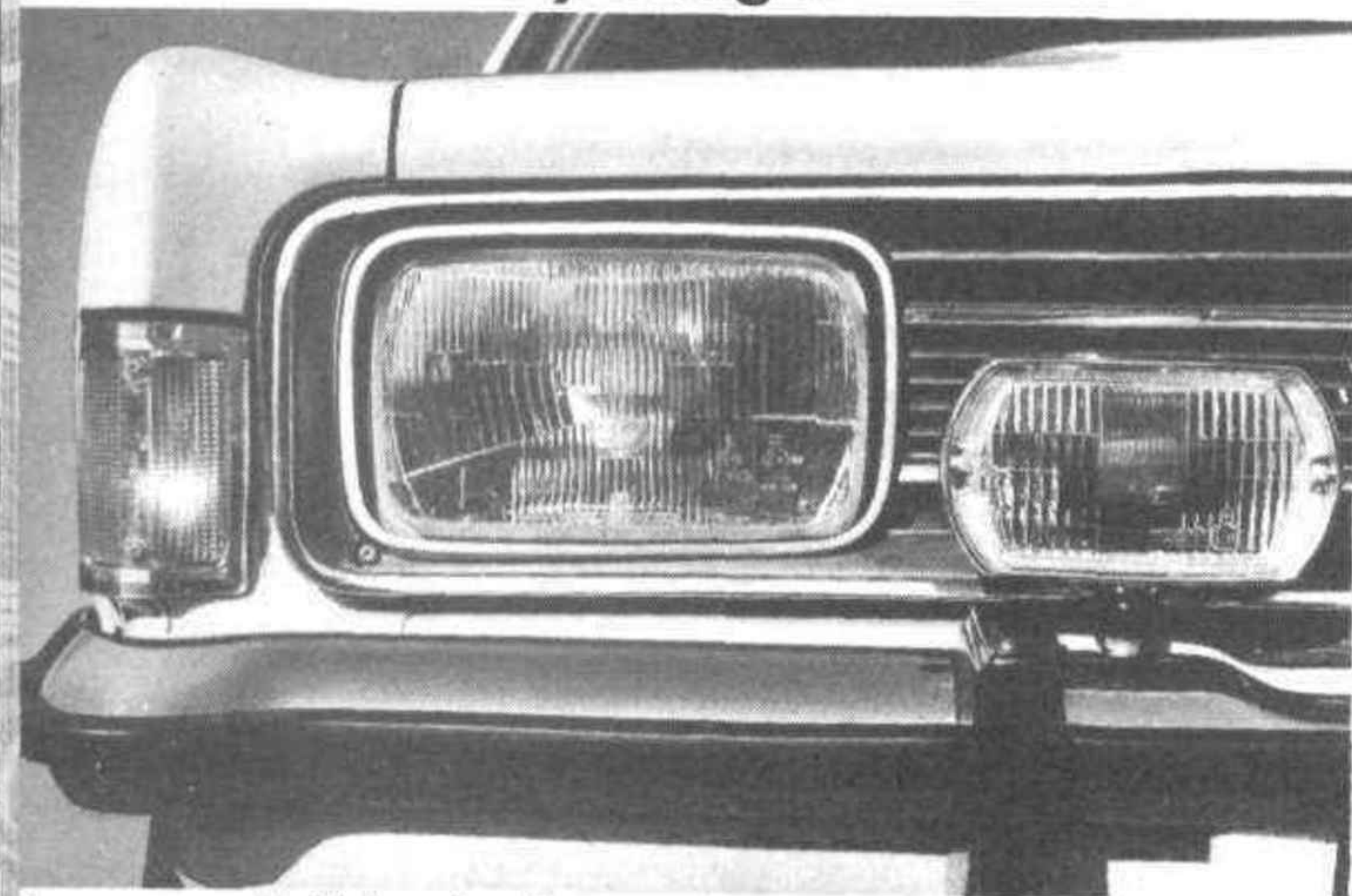
Lucas rectangular Halogen headlamp unit. Lucas Square 8 Halogen spotlamp.
