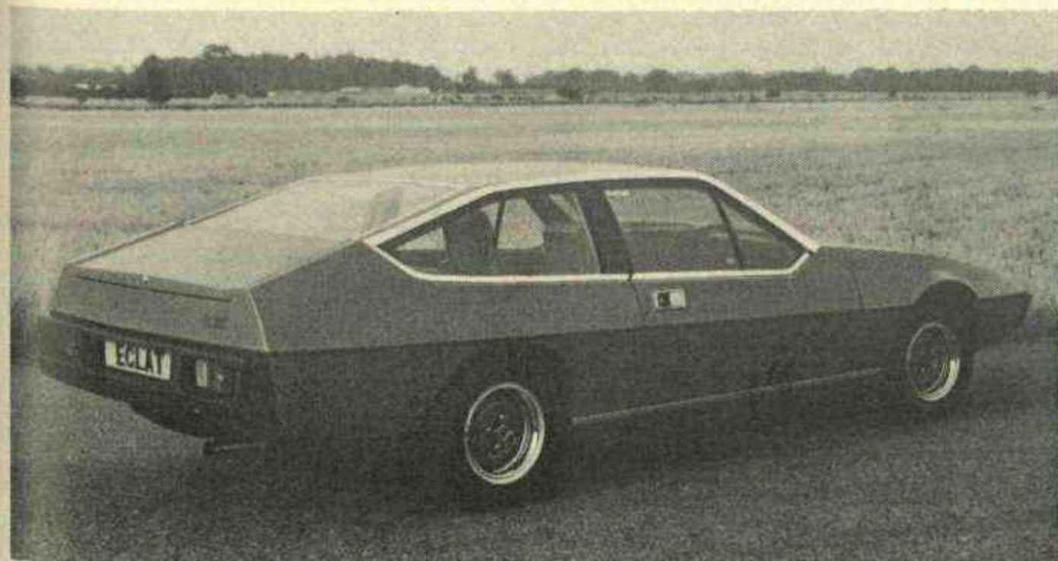
The Eclat's conventional boot has more room than the Elite's "glass-house". Less rear-seat space results from tilting the seats to increase boot volume.
