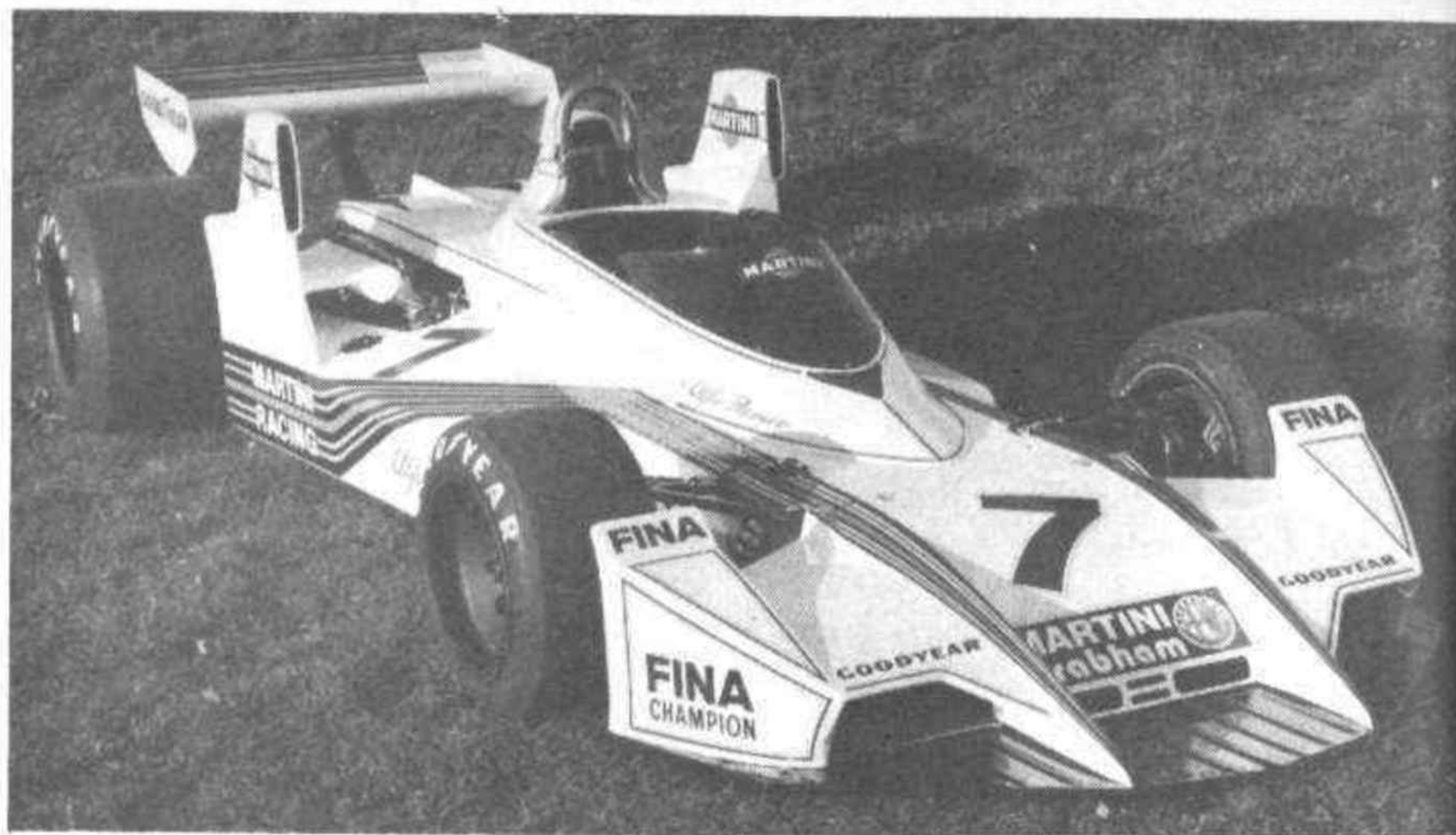
Martini Racing have announced the Martini Brabham BT45 Formula One car powered by a 3-litre Alfa Romeo flat-12 engine. This brand-new car, designed by Gordon Murray, with close co-operation on the engine side from Ing. Carlo Chiti, head of Autodelta S.p.a., uses front and rear hubs and front upright castings from the Cosworth-engined BT44B. Carlos Reutemann has tried the car briefly at Silverstone. We hope to give full details next month after further testing in Italy.
