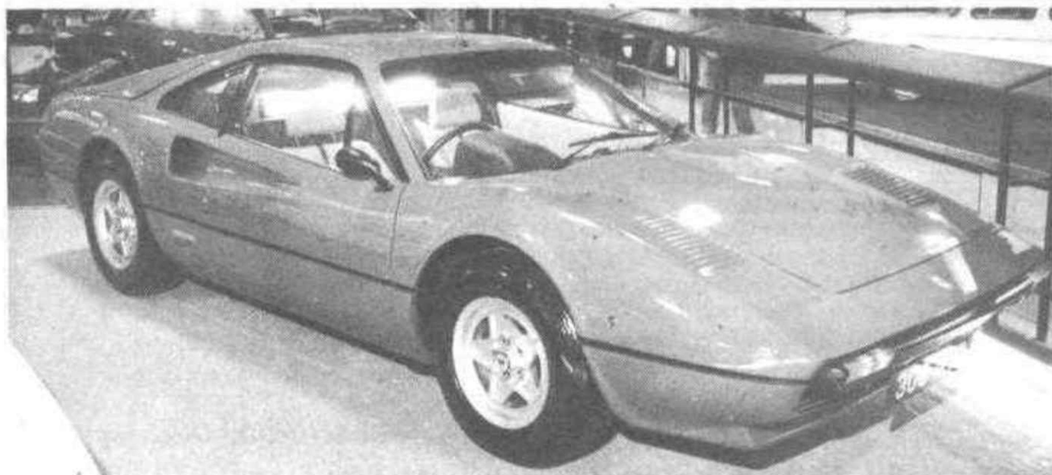
A new classic Ferrari. Taking over from the Dino 246GT as "the most beautiful dream machine" is the two-seater 308GTB, bodied in glass-fibre—the first time on a production Ferrari—by Scaglietti. Chassis (shortened by 3 in.) and running gear is from the 308GT4 2+2. The mid-mounted 2,926 c.c. V8 develops 255 b.h.p. and the quoted maximum speed is 156.6 m.p.h. It costs £11,992.
