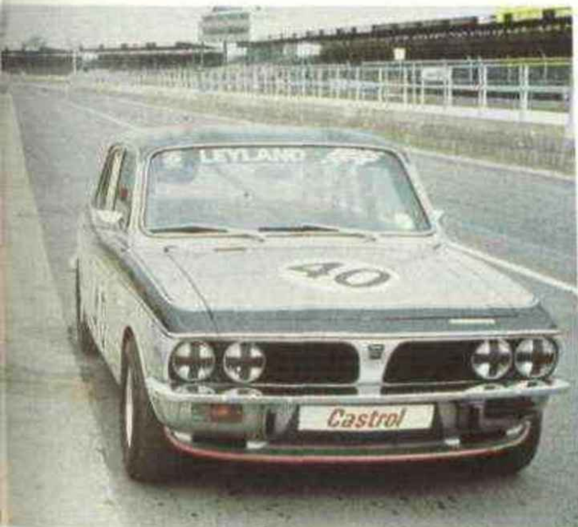
ABOVE: NORMAL RAC Championship Sprint lacks the L'Avenir car's big wheel arches and some 45 b.h.p.
