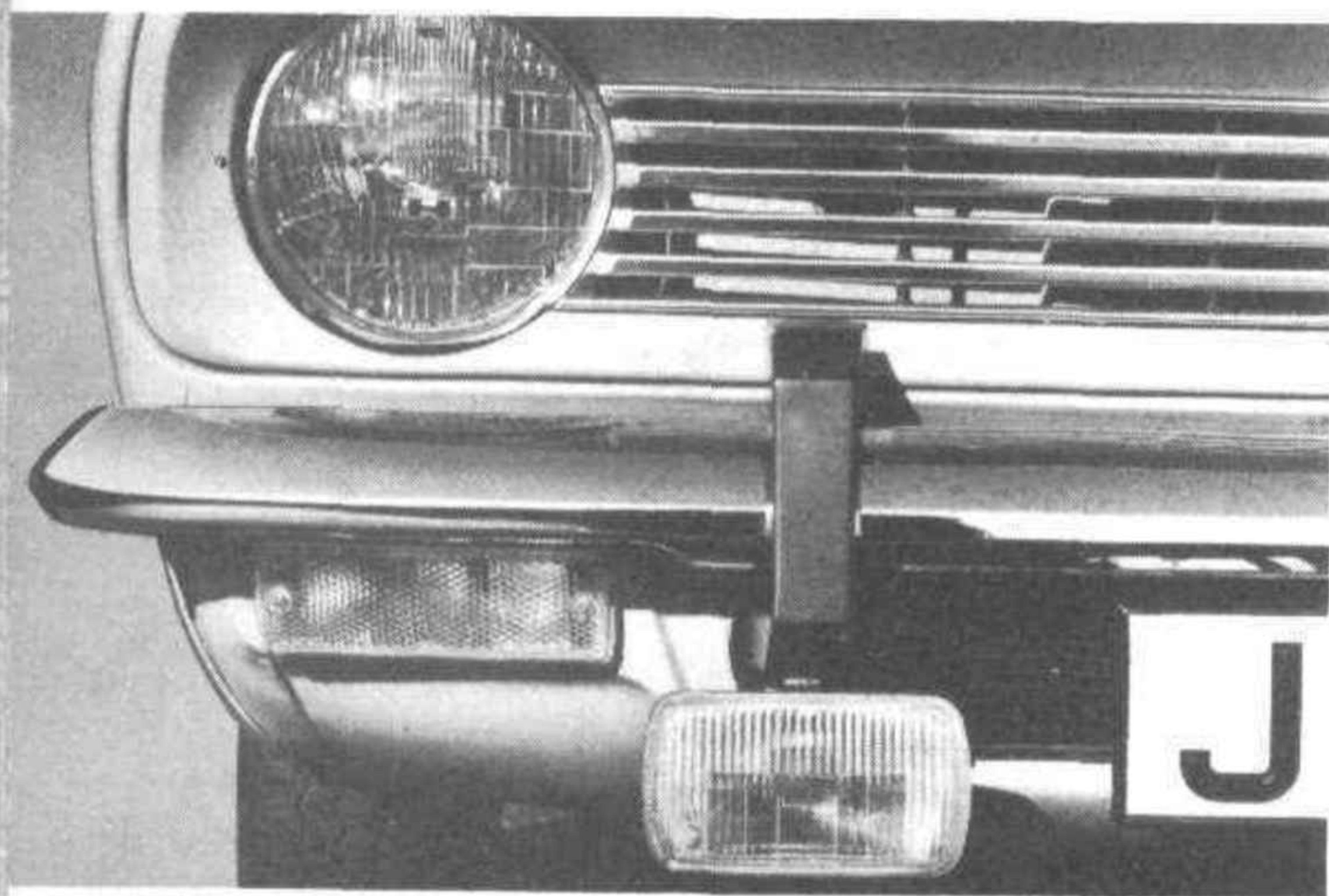
Lucas 7" Halogen headlamp unit. Lucas "Overrider" lamp bracket with Lucas Spectre Halogen foglamp.
