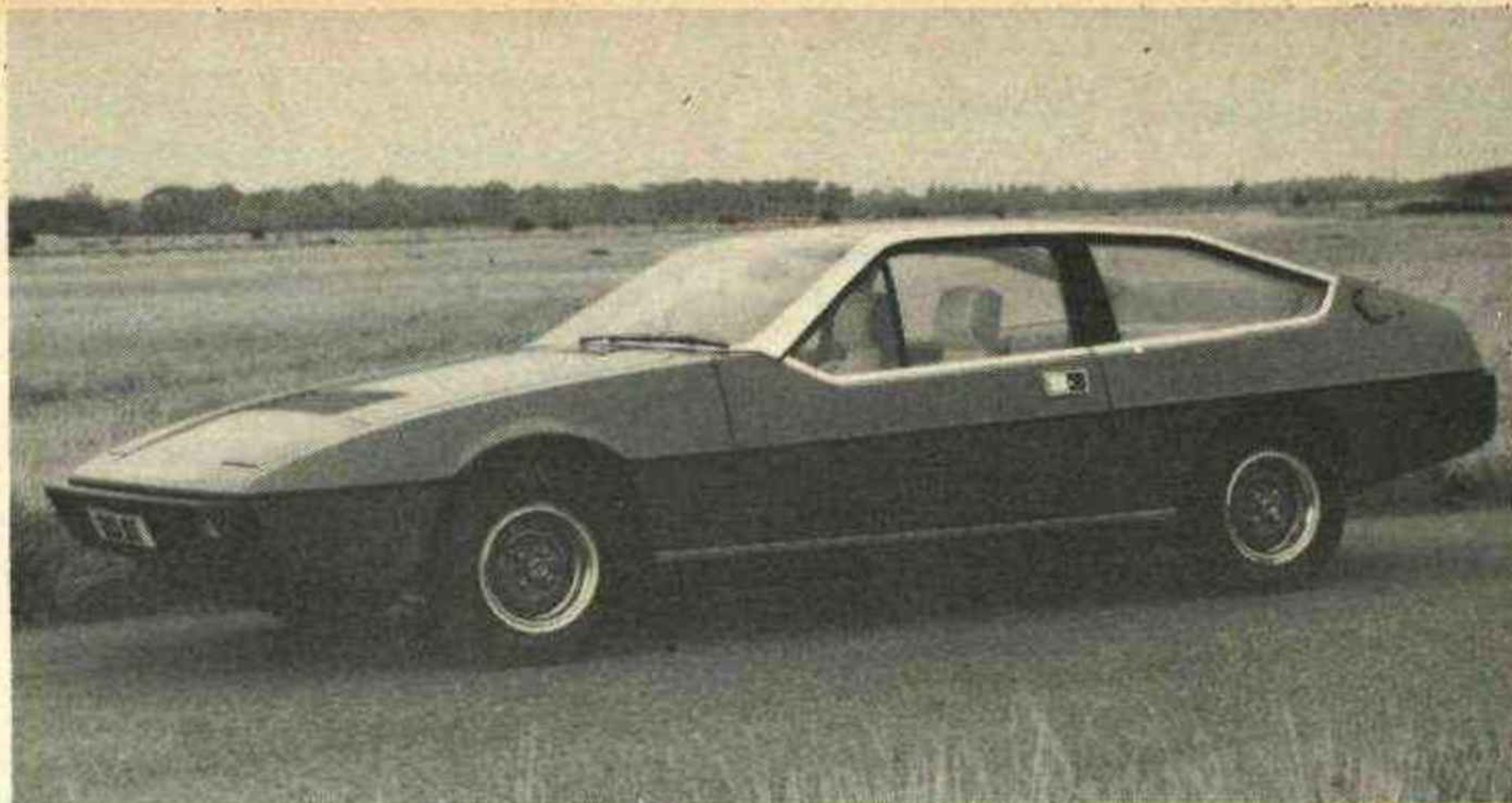
The new Lotus Eclat, an Elite-based 2+2 coupé. This is the basic 520 model, with 4-speed gearbox and narrow-rim wheels. Sportier performance and handling is said to result from some 300 lb. reduction in weight.
