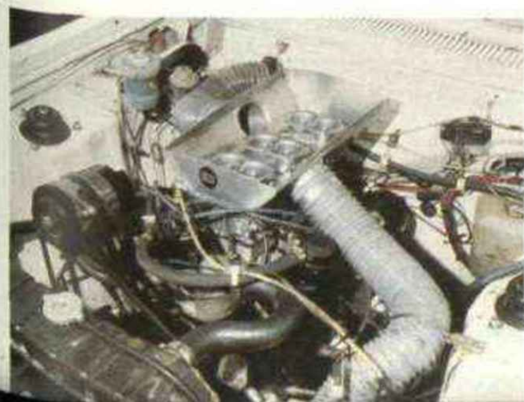
LEFT: Three downdraught Webers feed the Racing Services-modified 3-litre Capri II V6. RIGHT: Oof! British series is full of moments like these, which is why sponsorship is so important!
