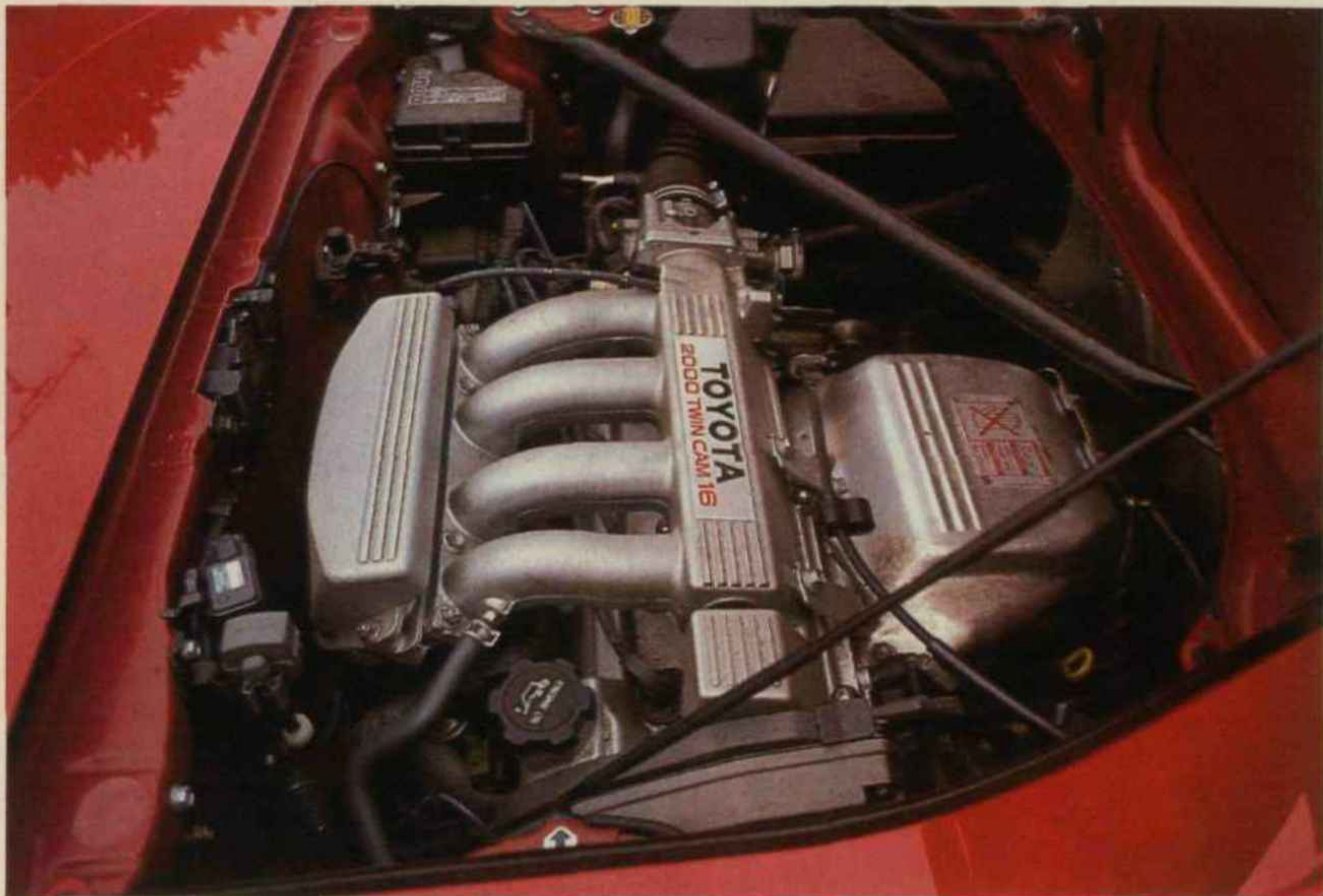
The 158 bhp 2-litre engine which powers the GT and T-bar versions.
