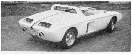
Suspension is all-independent, by helical springs and wishbones controlled by telescopic dampers. An anti-roll bar is fitted at the rear. Rack-and-pinion steering is used, in conjunction with a telescopic column. A unique feature is that the seats are fixed, but the pedals and hydraulic units are adjustable fore-and-aft.
