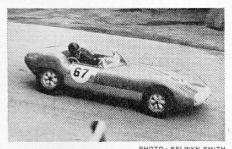
This body, as used on he very successful Rejo' 1172 Formula cars, is supplied as two separate units to fit any wheel base and up to 3' 11" track. It is therefore, suitable for re-bodying most sports racing cars and
