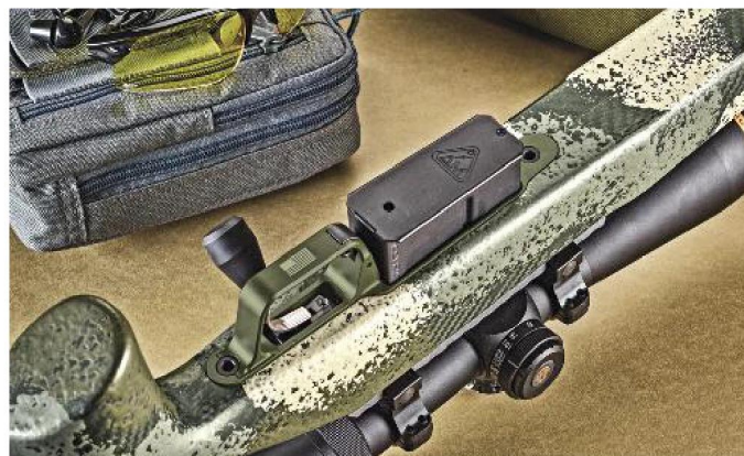
The receiver and bottom metal are dimensionally similar to the Remington 700, meaning stock changes are possible, if necessary. Center-feed AICS magazines facilitate reliable loading.
