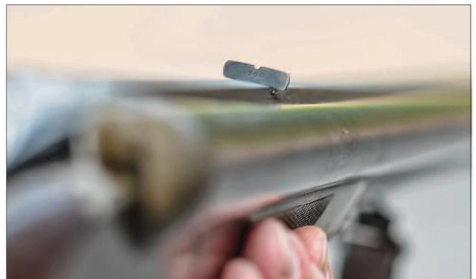
When the rifle barrel is selected, a rear sight automatically rises up from the rib for aiming.
