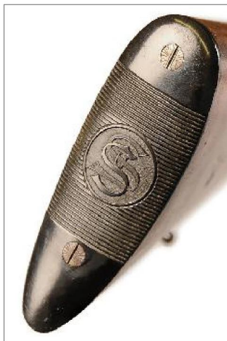
Sauer employed the firm's standard hard-rubber buttplate on the M30.
