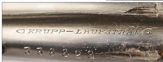
Traditionally, the barrels were identified with caliber and gauges. The Eagle 2 Luftwaffe ordnance inspection stamp can be seen on the forward locking lug. Barrels of high-grade Krupp-Laufstahl steel were so marked.
