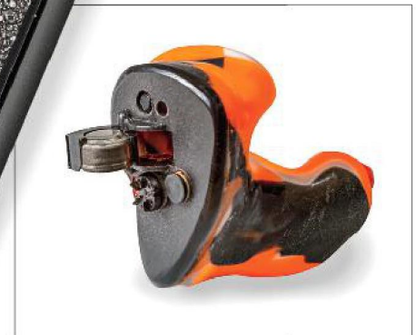
Each unit is powered by a common size 10 hearing aid battery.
