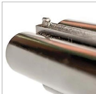
The drilling's front sight was designed for use with the rear rifle sight, or it could stand alone as a shotgun bead.
