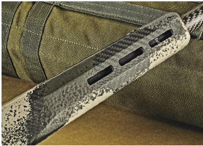
Three M-Lok accessory slots are built into the forend of the AG Composites stock. Compared to the usual sling stud, they offer a more secure mounting point for bipods and rails.
