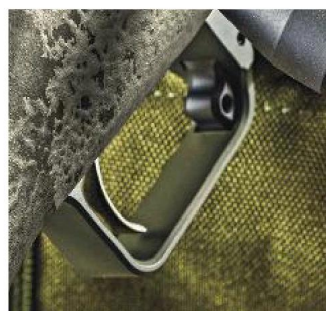
A magazine release is located in the lower front corner of the triggerguard.
