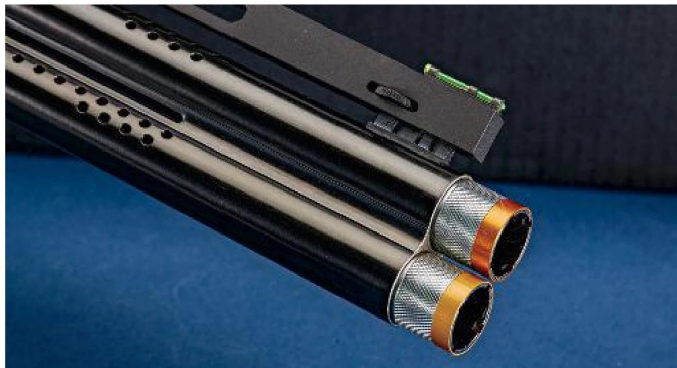
Sight picture is adjustable at the front as well as the rear. Turn the knurled thumbwheel at the front of the rib to adjust it up or down. Moving the rib down raises the shot charge point of impact.
