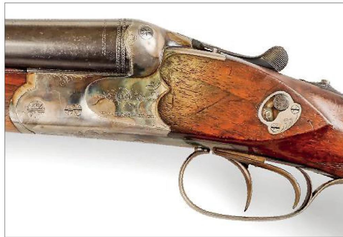
The M30's safety was a handy knurled button located on the left side of the stock just ahead of the wrist. This same feature was seen on German sporting arms.
