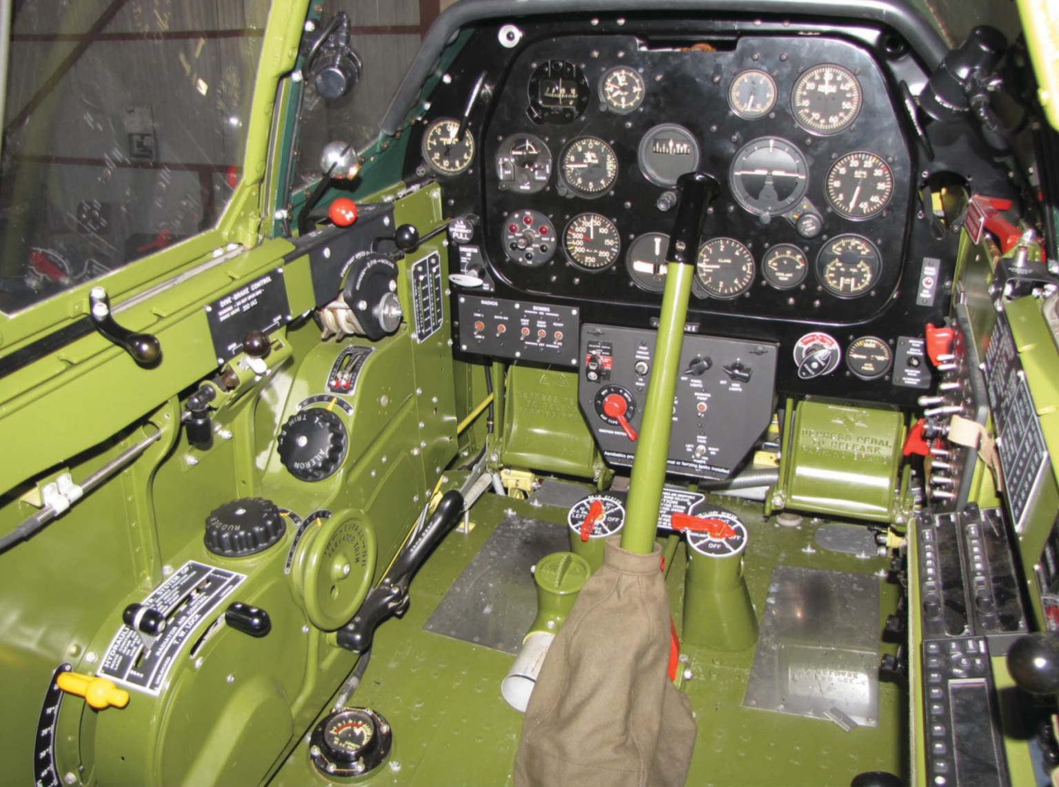
Above: The basic cockpit layout didn't change in any of the models. The gear handle is down by the left foot, trim wheel and knobs are under the left arm, fuel selectors are between the legs, and so on. (Photo by Frank Mormillo) Left: The "birdcage" canopy of the Allison airplanes didn't change when the Merlin-powered 51B/Cs were developed, but the Malcolm Hood replaced the center part. The 51D introduced the bubble canopy. (Photo by Frank Mormillo)
