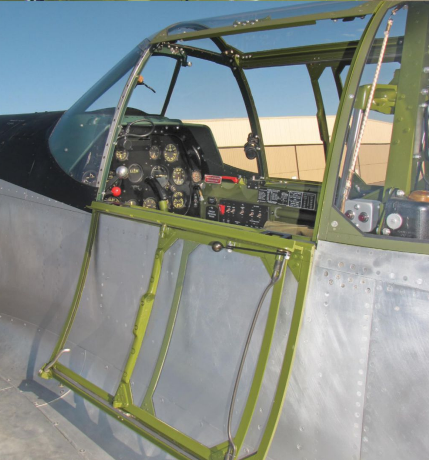
Above: The basic cockpit layout didn't change in any of the models. The gear handle is down by the left foot, trim wheel and knobs are under the left arm, fuel selectors are between the legs, and so on. (Photo by Frank Mormillo) Left: The "birdcage" canopy of the Allison airplanes didn't change when the Merlin-powered 51B/Cs were developed, but the Malcolm Hood replaced the center part. The 51D introduced the bubble canopy. (Photo by Frank Mormillo)
