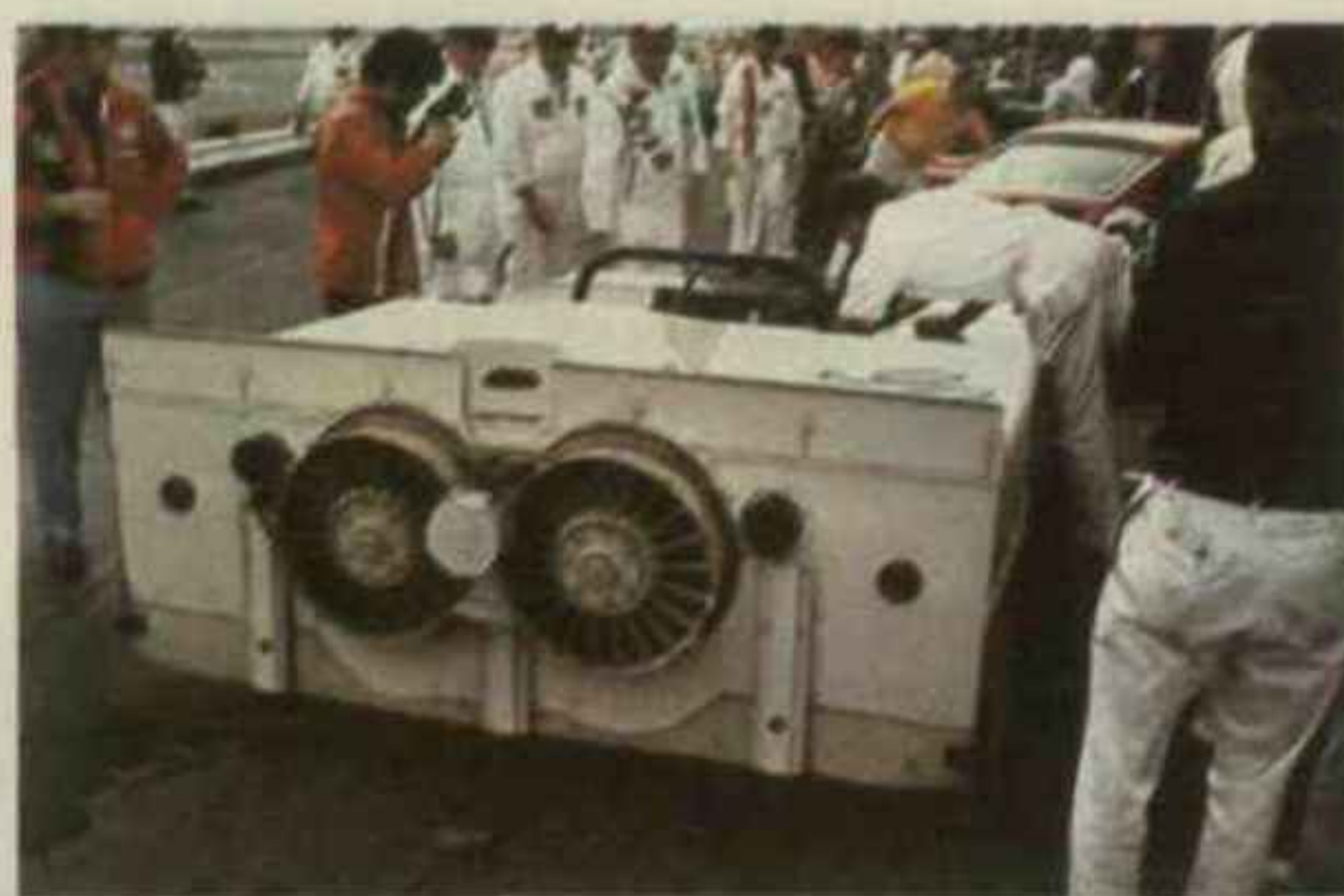
After the 2H came the amazing 2J – the sucker car on which two snowmobile engines extracted air from the underside to create the ultimate downforce device. Like the high wings, the cunning idea was legislated out of business.
