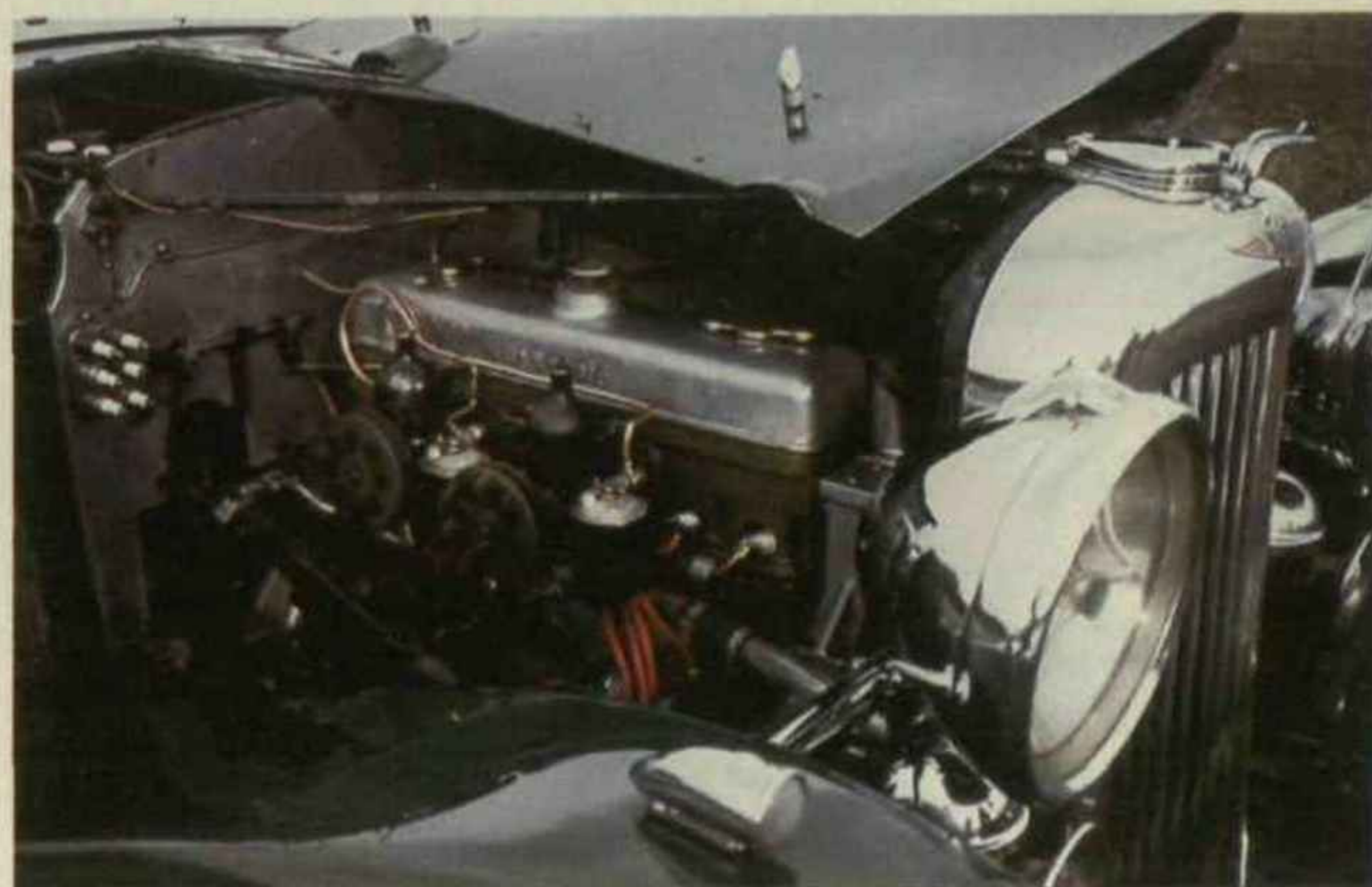
Sanction 1 engine has Sanction 3 head and Rapide pistons, giving higher compression.
