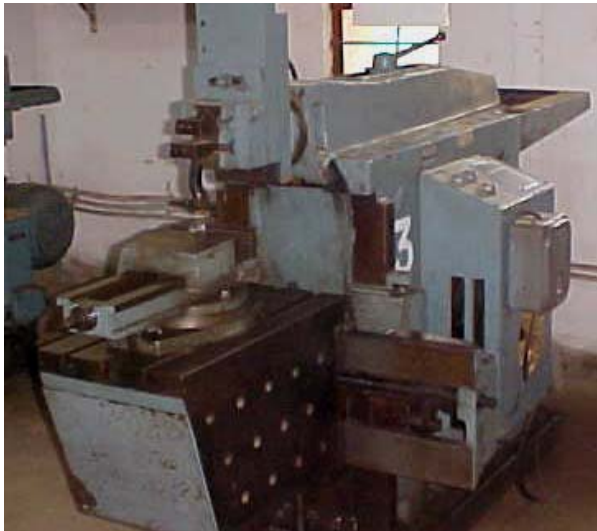
Fig. 4.5.19 Mounting of job and tool in shaping machine.
