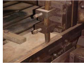
Fig. 4.5.20 Mounting of cutting tools in planing machine
