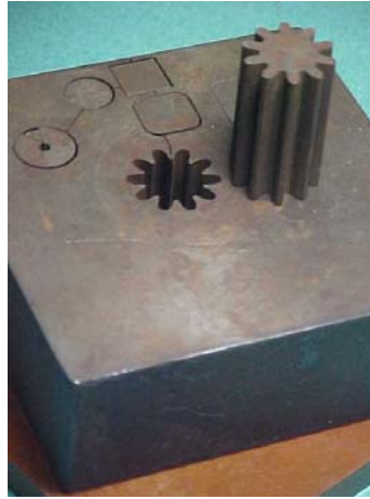
Fig. 7.2.9 Production of teeth of external and internal spur gears by Wire-Electrodischarge machining (EDM)
