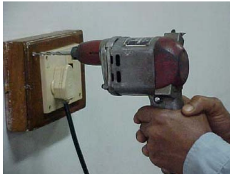
Fig. 4.2.5 Hand drill in operation
