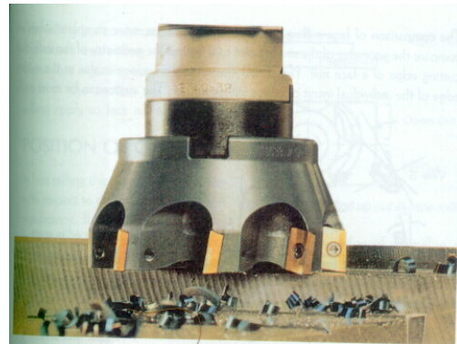
Fig. 4.3.17 Face milling cutters and their working
