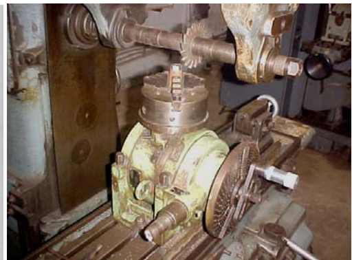
Fig. 4.5.22 Mounting of job on the dividing head in milling machine.
