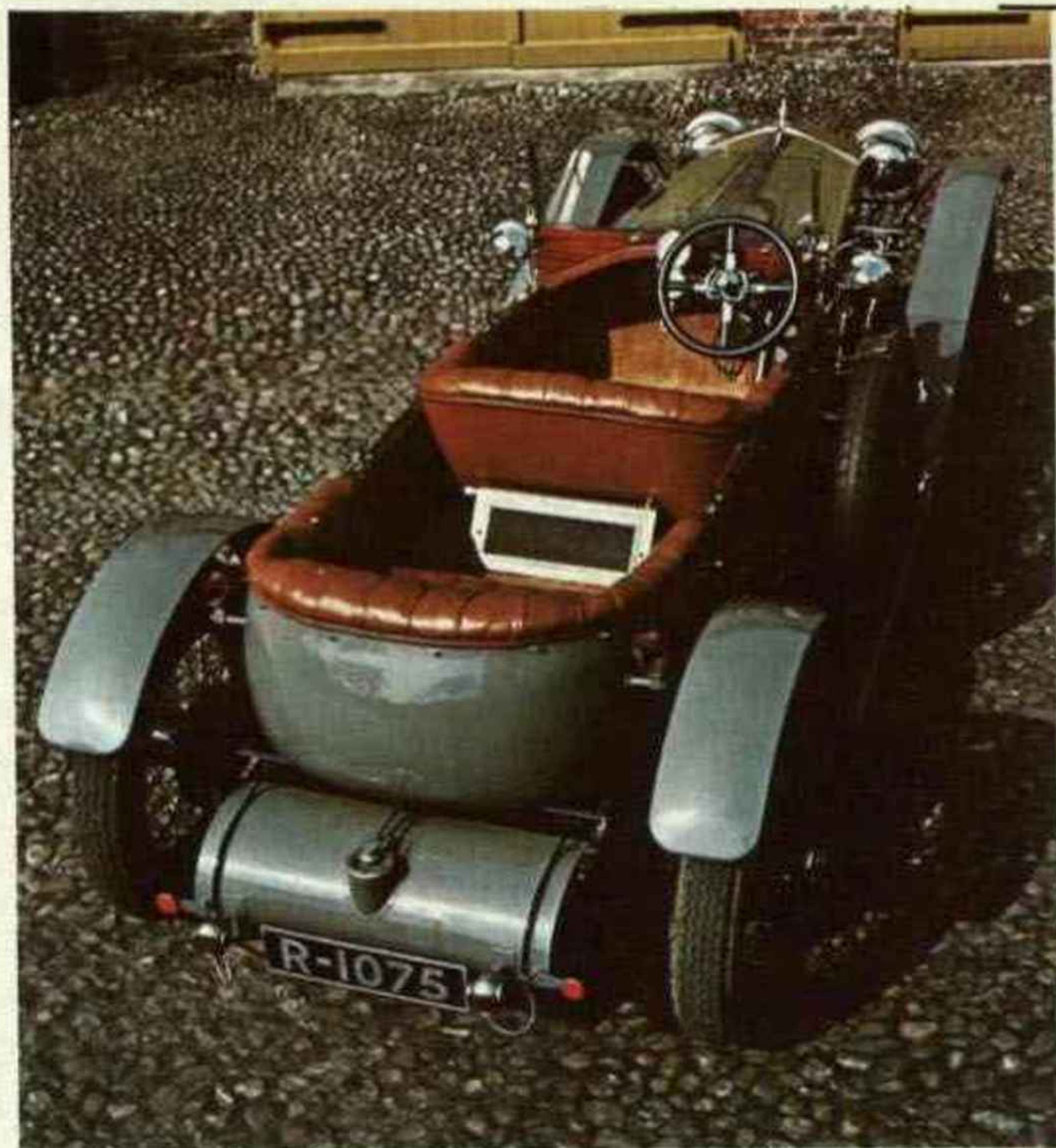
This three-quarter rear view of the sporting Silver Ghost shows the elegant curves of the tail, made like the remainder of the body in Mr. Neve's home garage, and of which the Frazer Nash "Chain Gang" fraternity should strongly approve. Note the foot-ramp, concealing a tool-locker, for the back-seat passengers and the original registration number.
