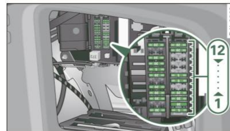
Fig. 236 Right luggage compartment: fuse panel layout
