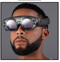
The Nreal Light weighs roughly 88 grams while the Magic Leap One is nearly four times heavier at about 325 grams for the headset, plus an additional 415 grams for the computing pack.<sup>10</sup> The
