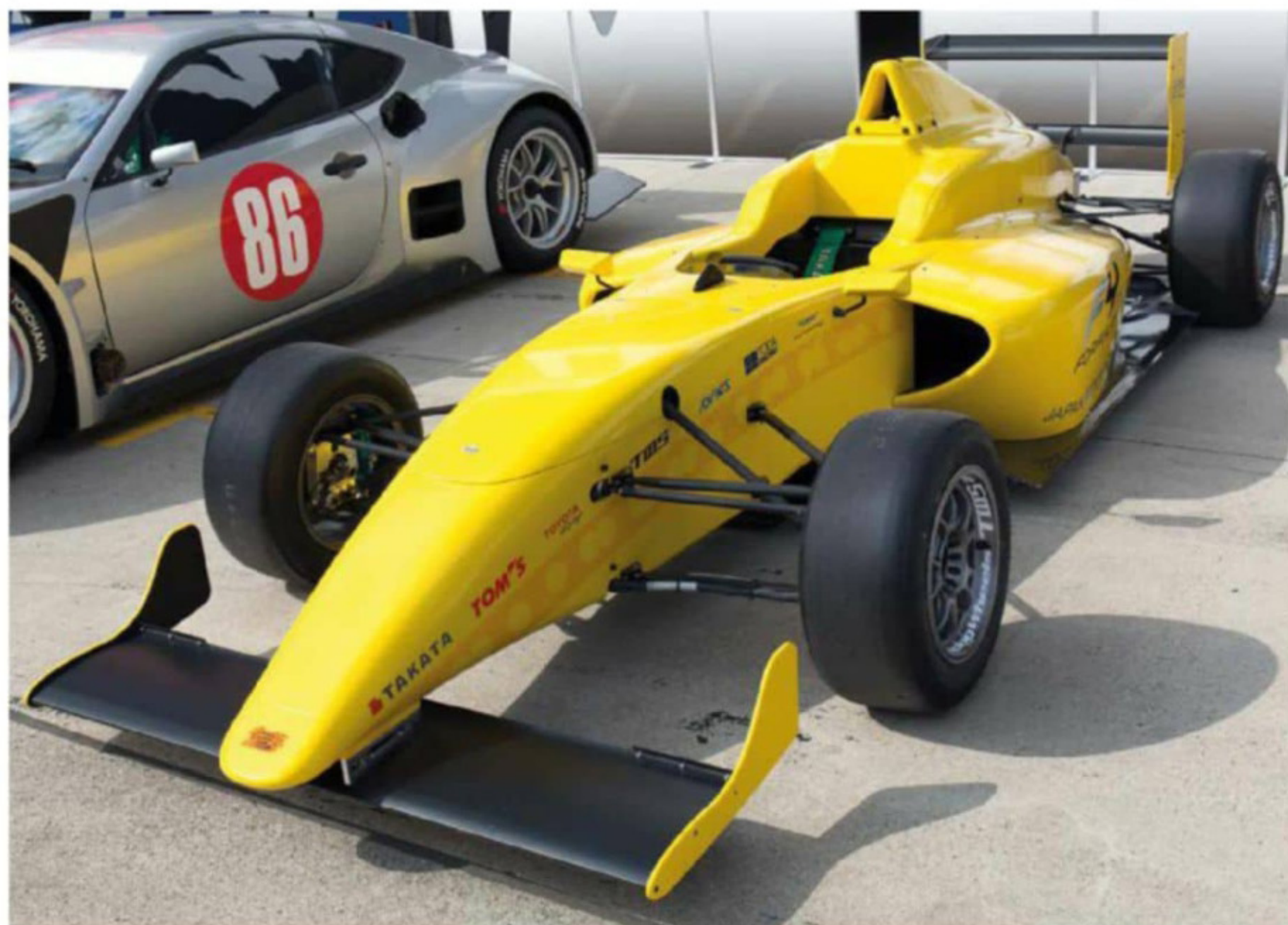
Dome F110 in standard F4 trim. ERA has designed a frame for the rear so the suspension pick-ups will remain the same
