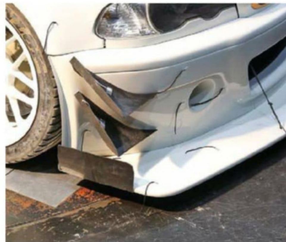
Two splitter end fence sizes were tested; this is the larger one
