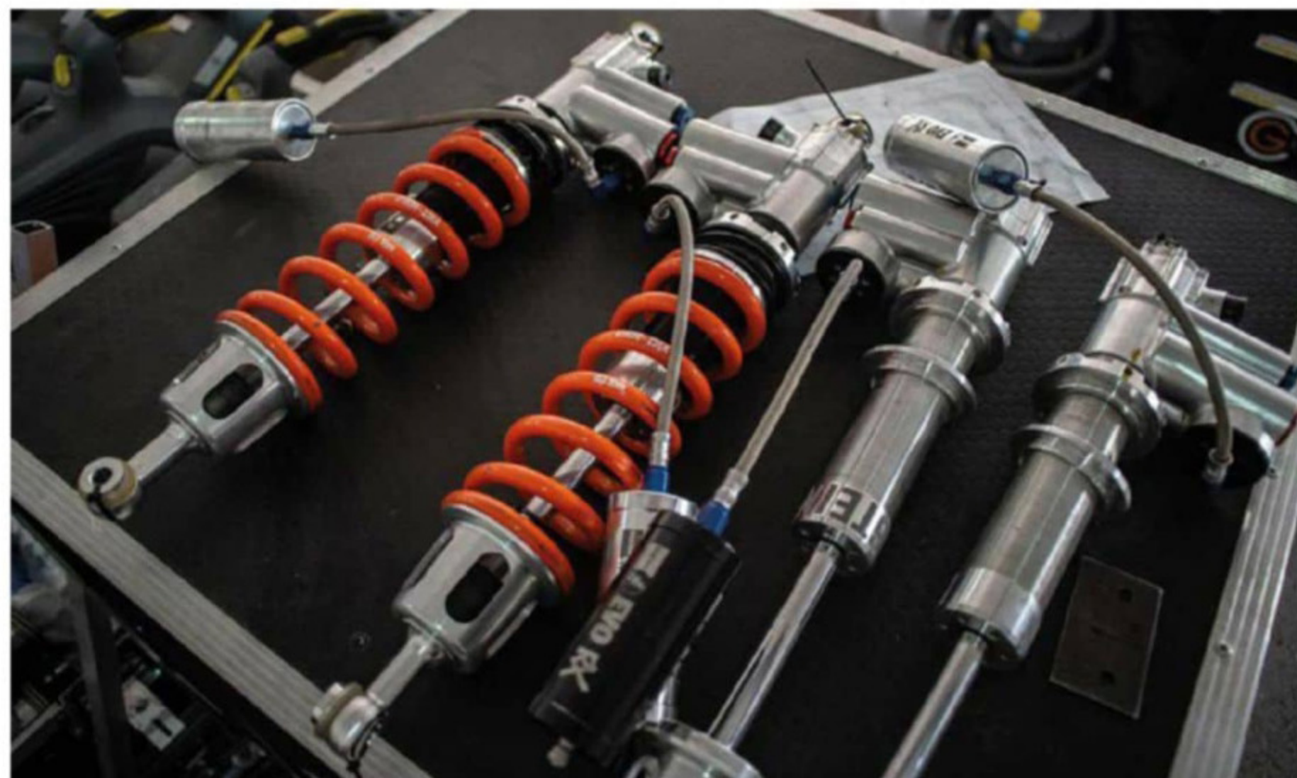
For 2019 GCK switched from Ohlins to Bilstein. Damper design is a challenge due to the tight confines of the wheel housing
