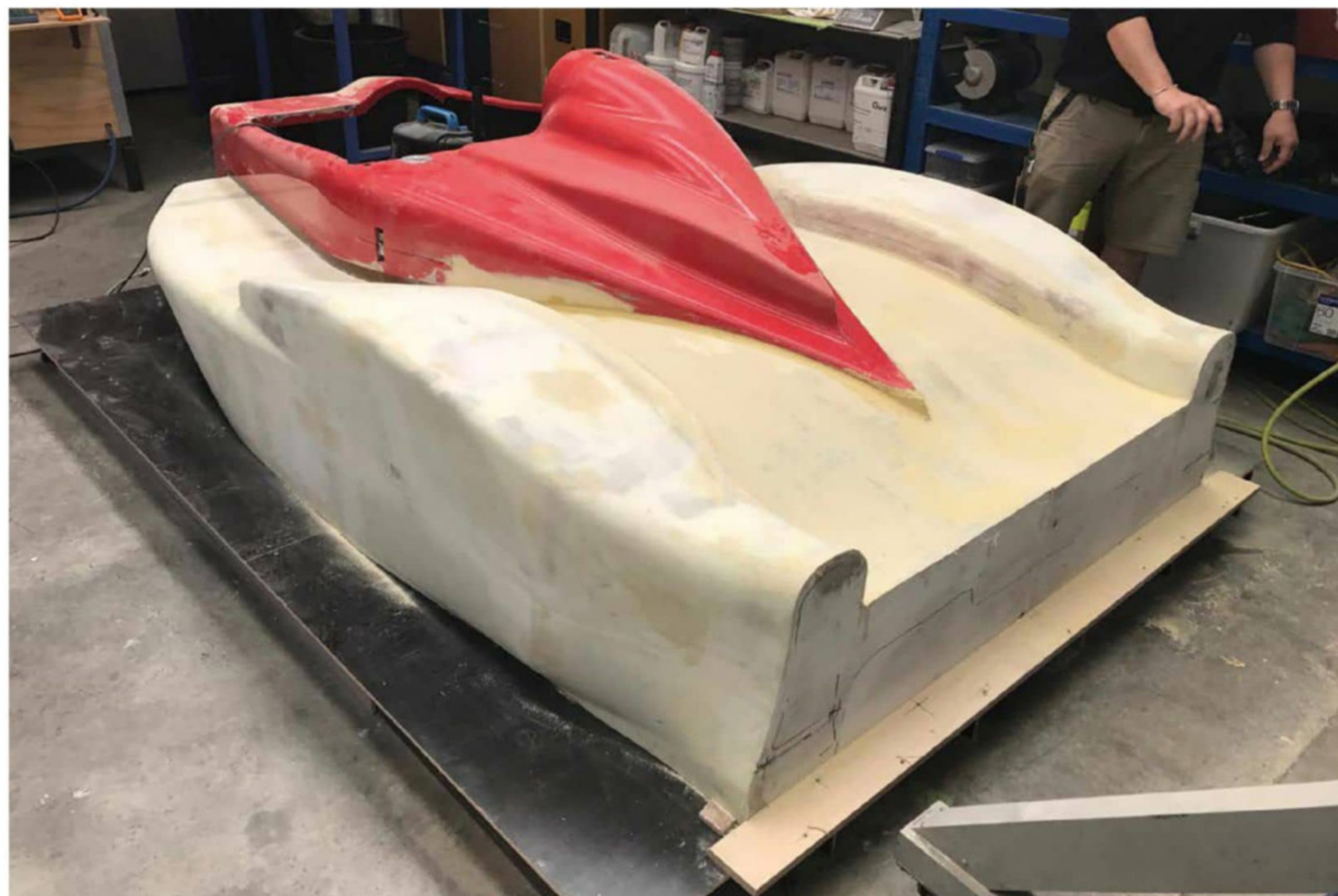
The manufacturing of the carbon moulds is by way of a vacuum infusion process with a relatively low temperature cure. The entire body will be in carbon when the racecar is finished
