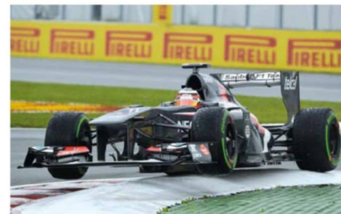
Drivers have a habit of using kerbs and you will need to factor the likelihood of this sort of chassis abuse in to your racecar design
