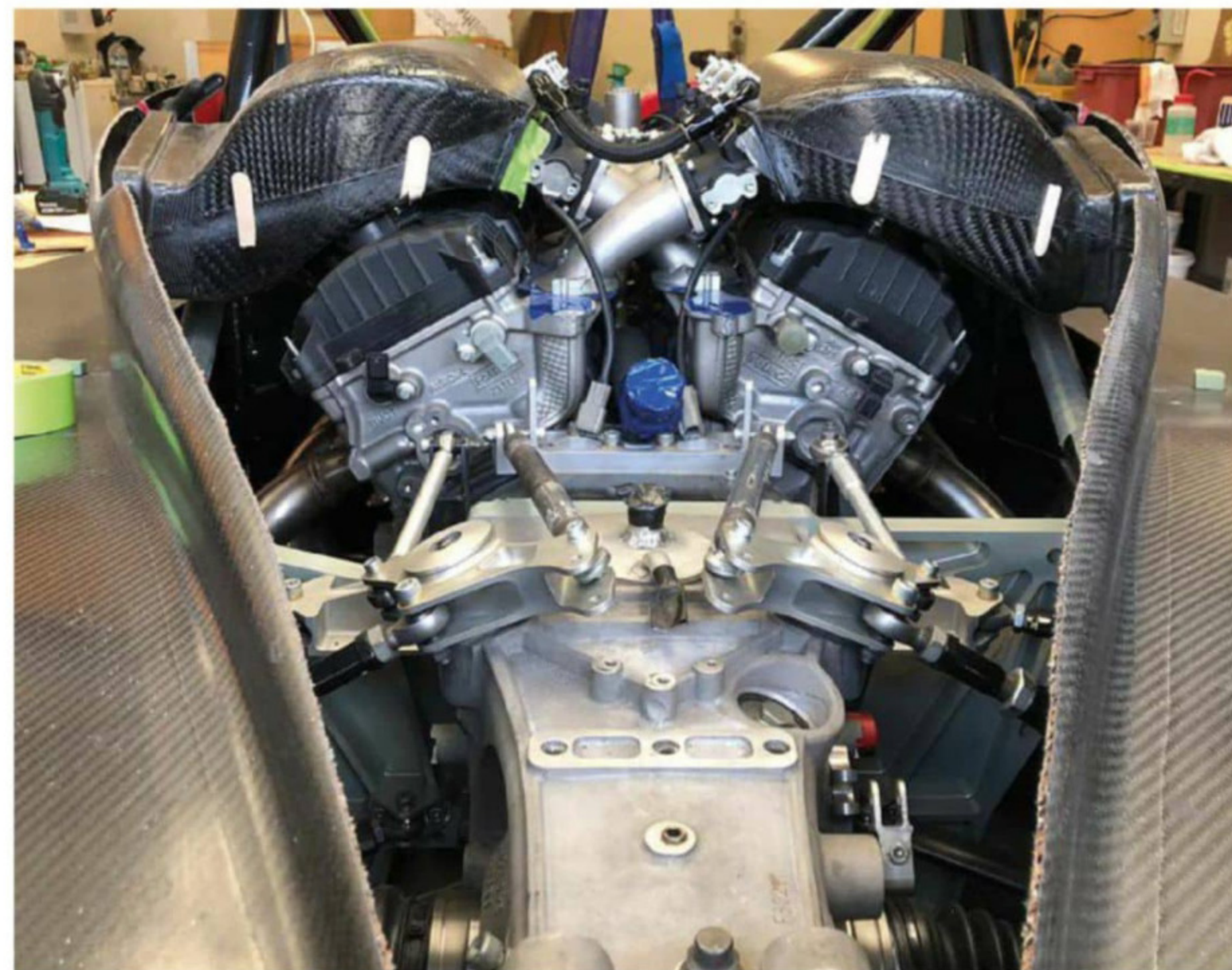
Power is courtesy of a 3-litre Duratec that's been bored out to close to 4-litre. The gearbox is a 6-speed Drexler sequential
