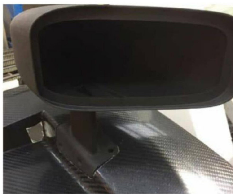
The team behind the Matos is especially proud of the racecar's mirror housings, designed and produced with CRP Windform
