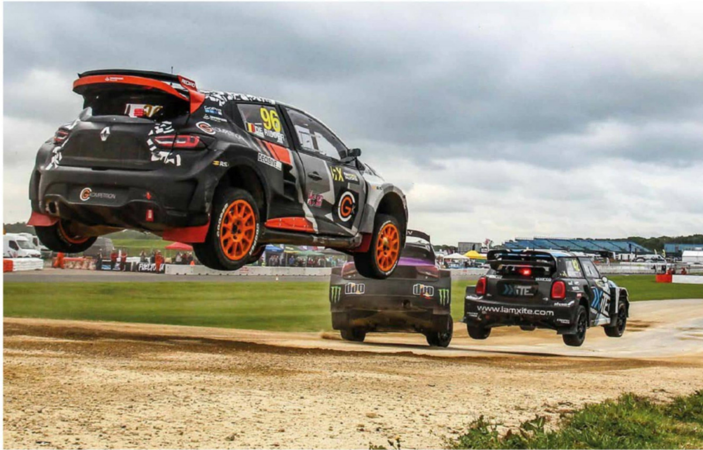
Dampers are really put to the test on the jumps in WRX, where they require a soft rebound yet a stiff compression. Silverstone's jump, at two metres, is the highest of the season
