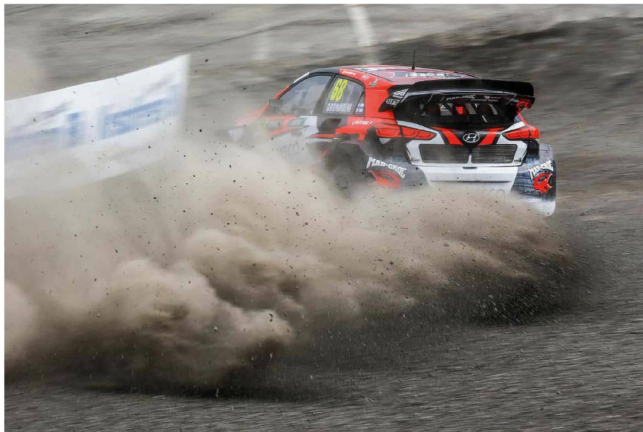
With an ever-changing track surface on the gravel sections of a rallycross circuit drivers need a good feel for the available grip and so the cars often use a soft suspension set-up
