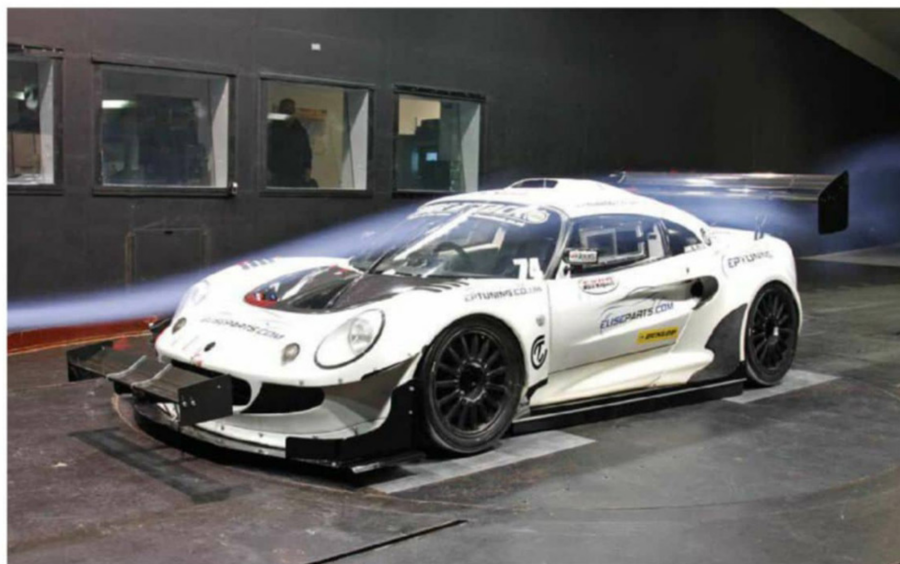
A wind tunnel is, in essence, a dyno for aero and as such it's a great comparative tool. But it won't give you absolute numbers
