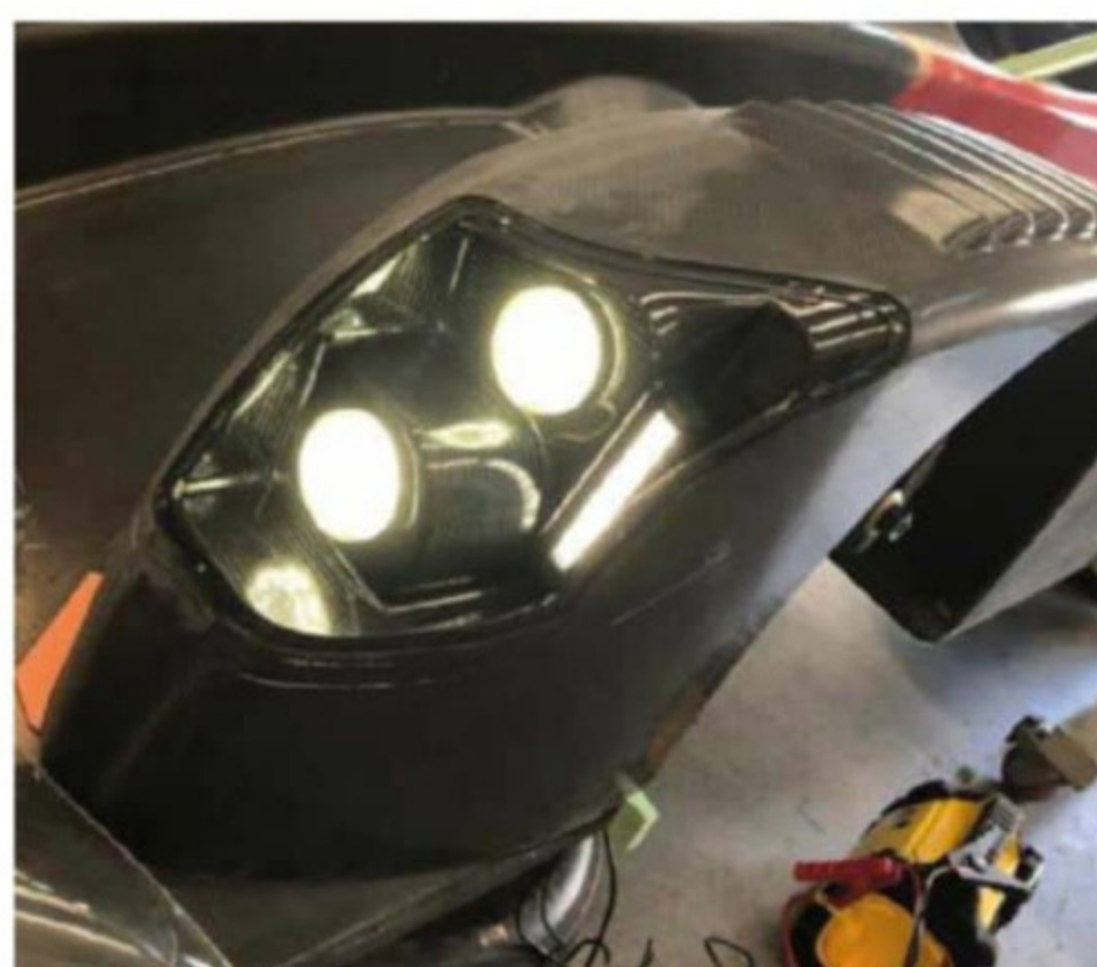
The lenses for the LED lights are made using a vacuum forming process with a mould that's taken from the fender's own mould
