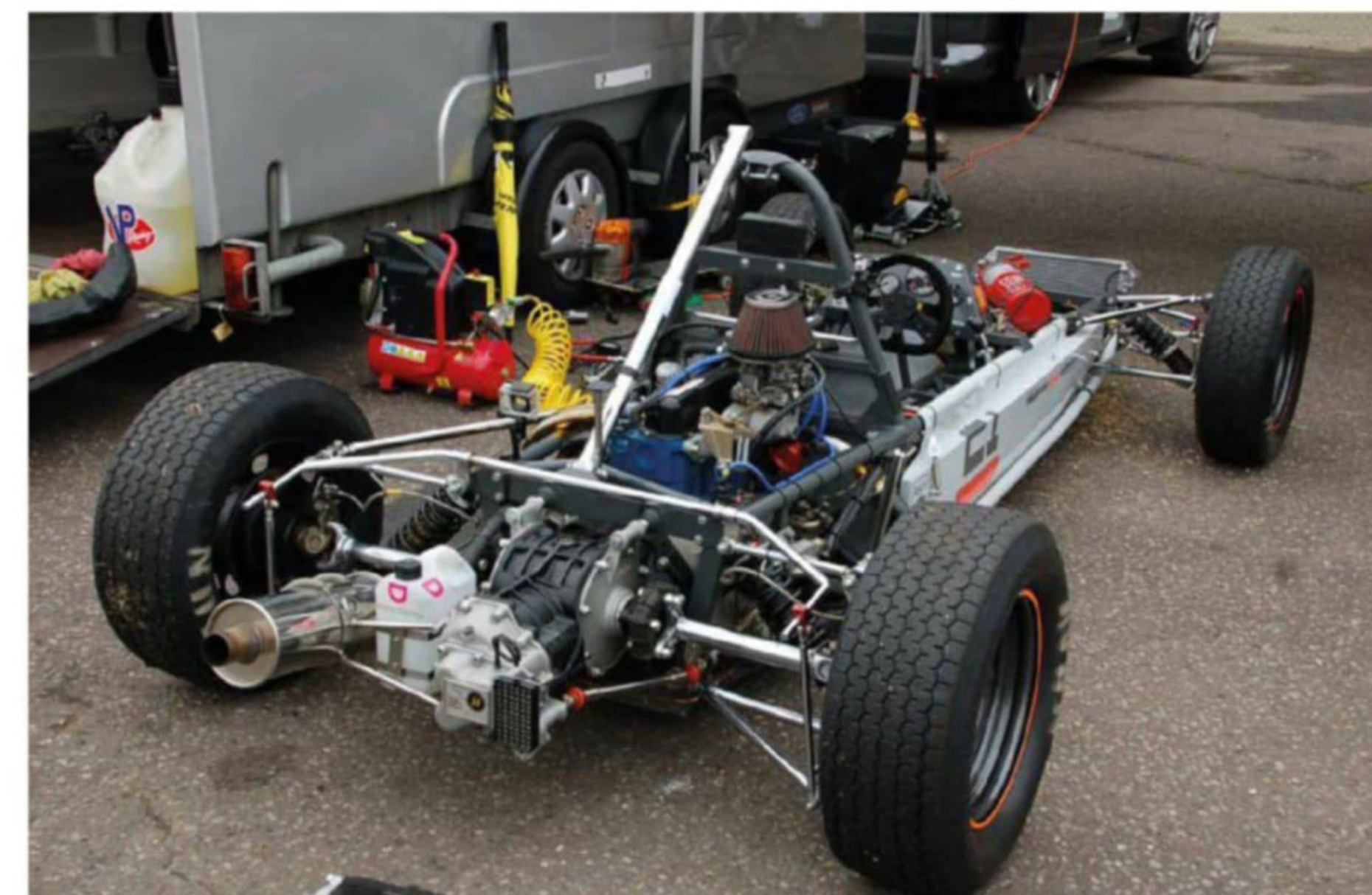
Old style anti-roll bar on a Formula Ford 1600 – it's adjusted by sliding the vertical rods on either side along the bar
