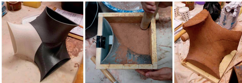
Image 2: The initial mold system made with 3d printing, and the first casting experiment of the unit cube of Gyroid.
