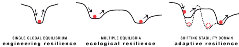
Figure 1: Ball and cup model of system stability in competing resilience frameworks. The valleys in the surface represent equilibrium or stability domains, the ball represents the system, and arrows represent disturbances. (Laboy & Fannon, 2016).
