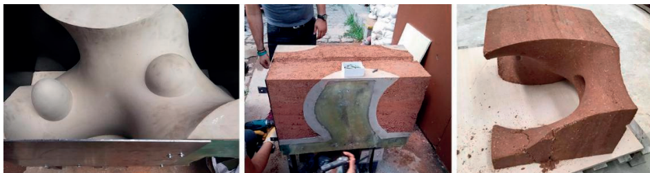
Image 3: Left: The industrial mold. Middle and right: The second casting experiment made with a revised compound recipe, using the industrial mold.
