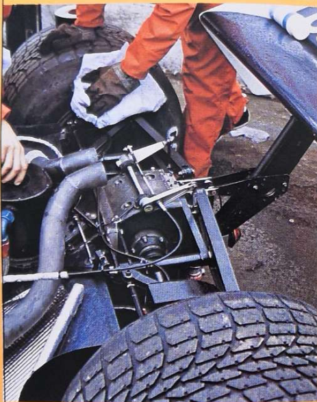
Zunino used the Weismann transverse gearbox.
