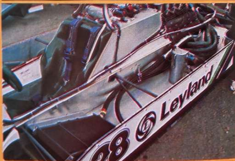
Oil radiator in place of the heat exchanger.
