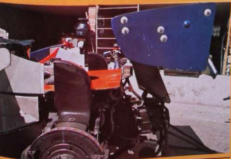
Forward mounted rear wing tested.
