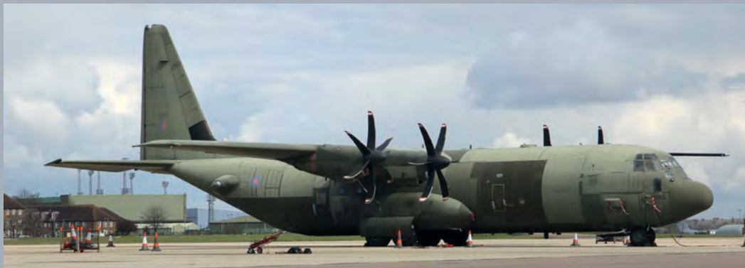
Above: C-130Js have now been in service for 17 years and, after tireless work in Iraq and Afghanistan, have needed plenty of patching up. If the C4s, like this one, are to continue until 2035 they will need their wing-boxes replacing too. Alan Warnes
