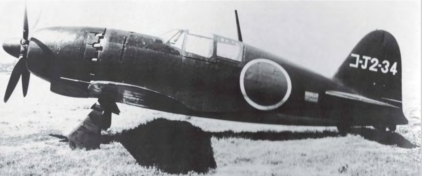
BELOW: The prototype of the J2M3 was issued to the Air Arsenal in October 1943, this variant featuring an enlarged oil cooler and external intake beneath the engine. It was the most-produced of all Raiden variants, 260 being built. This particular aeroplane subsequently served with the Chushi Kokutai in China. VIA YASUHO IZAWA
